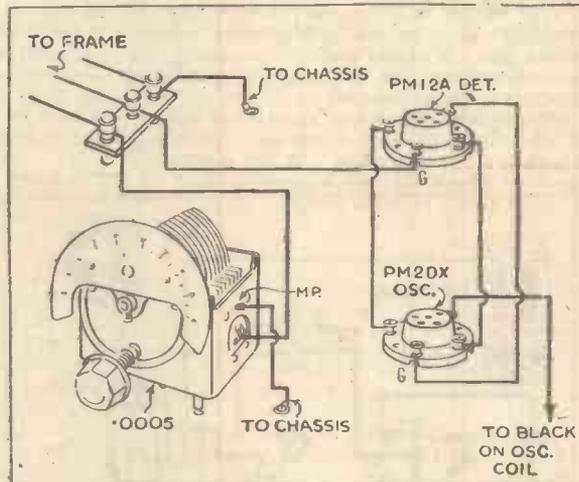
Improved results are obtained if the frame aerial has a centre tap (three terminals)
