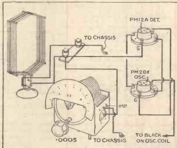
Connections for a two-terminal frame aerial on the 1934 Century Super
