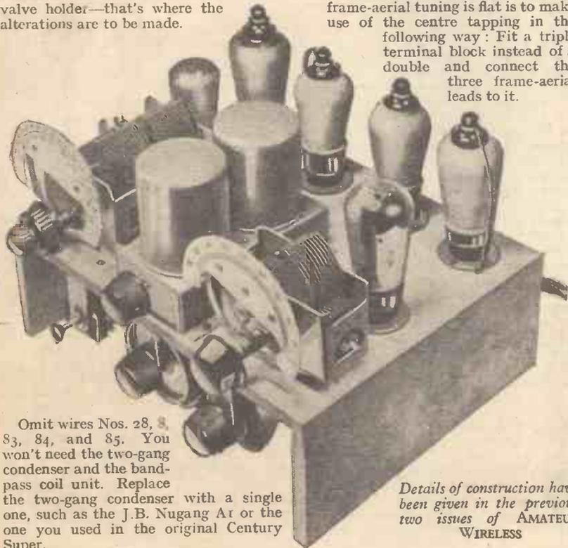
Omit wires Nos. 28, 83, 84, and 85. You won't need the two-gang condenser and the band-pass coil unit. Replace the two-gang condenser with a single one, such as the J.B. Nugang A1 or the one you used in the original Century Super.
