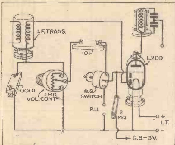
*How to fit the 1934 Century Super with a radiogram switch to change over from radio to pick-up at will. Nearly everybody will want to make this improvement!*
