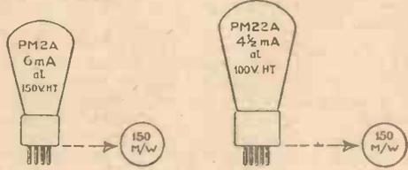
Here you see a Mullard PM2A power valve and a PM22A pentode, giving the same output. Note that the pentode requires 1 1/2 milliamperes less than the power valve and 50 volts less high tension
