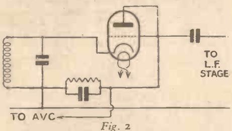
The only difference between this and the ordinary diode circuit is that here it is the grid end of the tuning coil that is earthed and
