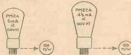
Here you see a Mullard PM2A power valve and a PM22A pentode, giving the same output. Note that the pentode requires 1 1/2 milliamperes less than the power valve and 50 volts less high tension
