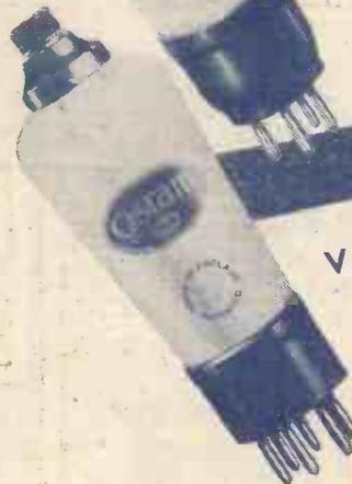
**VP21** The first screened H.F. Pentode for Battery Sets. Particularly useful for maximum amplification with low H.T. voltages, or in conjunction with high efficiency tuning coils. 7-pin base fitting which enables metal coating to be earthed.
