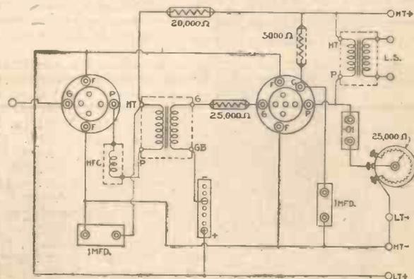
Typical pentode circuit, with an output transformer for correct matching, a tone control and a grid-stopper
