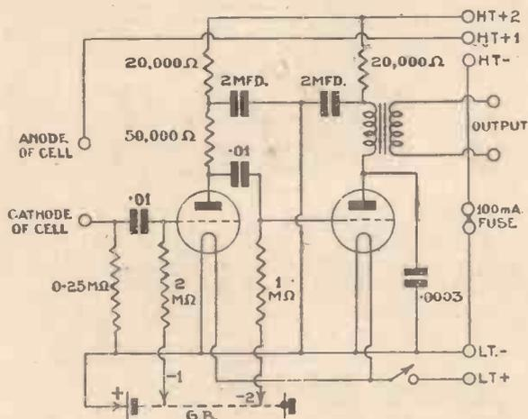
Circuit of simple amplifier for experimental photoelectric work
