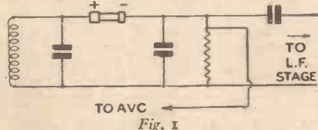
tion, however, rather obscures the fact that the resistance and the condenser are the usual grid leak and condenser which we use in ordinary valve circuits; it has the distinct advantage, however, that automatic volume control can be used with one set of vanes of the preceding tuning condenser earthed. It corresponds to the use of a diode valve upside down!
