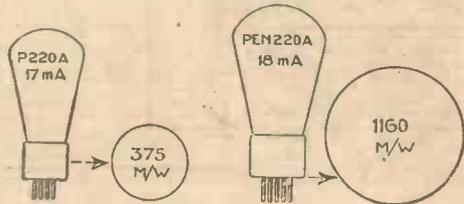
Output of a Mazda P220A and the output of a Pen220A compared with the approximately same anode current. The output of the pentode is three times as great
