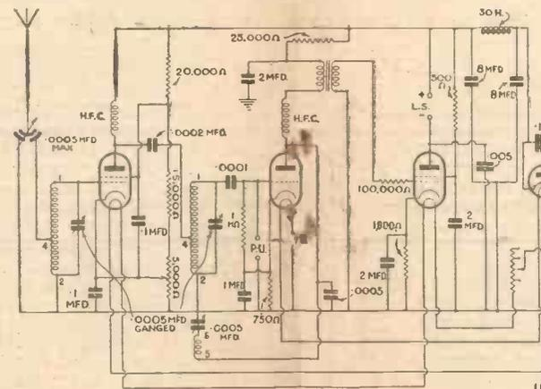
Circuit used for the A.C./D.C. three-valver fully described these pages. A full-size blueprint appears on the inside
