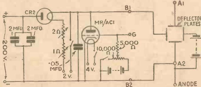
Fig. 1.—The single time-base circuit showing the connections to the deflector plates: note the biasing battery to centralise the movement of the beam
