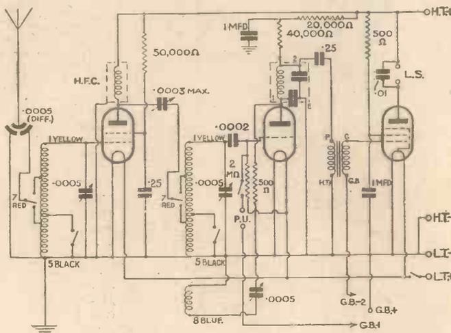
This is the complete theoretical circuit diagram of the 1934 Ether Searcher, which consists of an ordinary screen-grid stage, detector and pentode output. There are many important circuit improvements incorporated.
