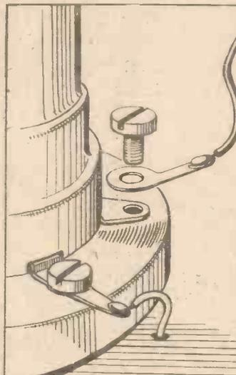
Soldered connections are rarely made to the component—the contact between the lead and the terminal is still a screw-down one, if soldering tags are used
