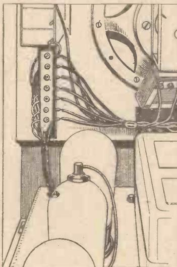
Earth wires, filament wires and low-frequency leads are unaffected by bunching, as in this example from a modern factory-produced receiver
