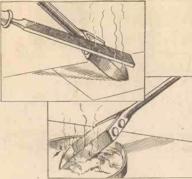
To tin a soldering iron quickly file the bit bright and without delay rub it in a mixture of solder and soldering flux
