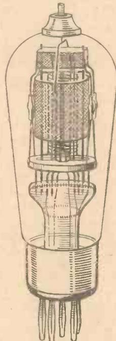
An Osram MHD4 high-slope detector
