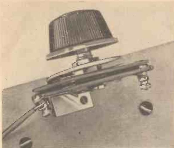
How the volume control is fixed by means of a special metal bracket, which is mounted on the baseboard
