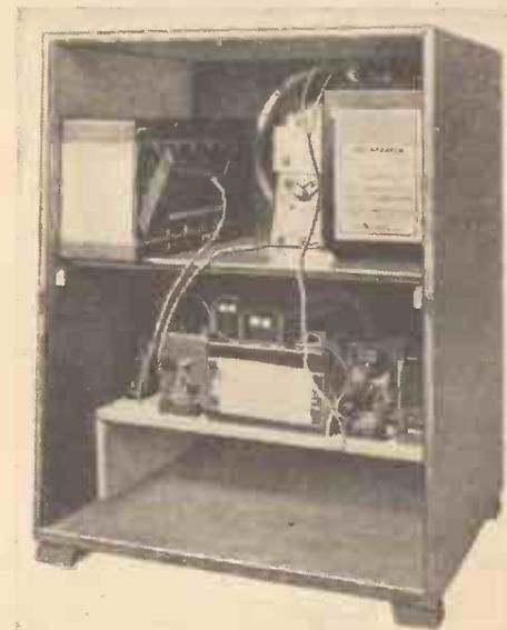
Back view of the cabinet, showing the positions of the set, the loud-speaker and the batteries
