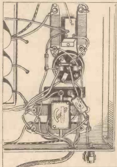
In a modern receiver parts are arranged to make essential leads short, while the non-critical wires are run in braided sleeving in groups
