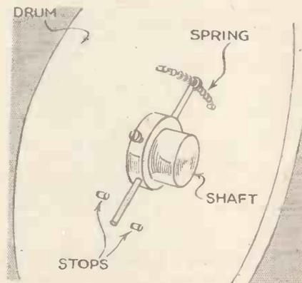
Fig. 2.—The movement of the drum or visor is controlled by two tension springs attached to an arm on the centre boss
