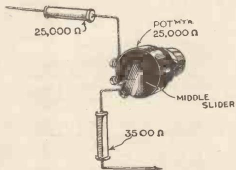
Fig. 1.—Use of three resistances in series, two fixed and one variable
