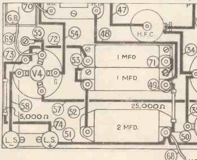
How the wiring is altered for pentode output. A complete full-size blueprint can be obtained for 1s. 6d., post paid; No. AW433 with triode output and No. AW433a with pentode output
