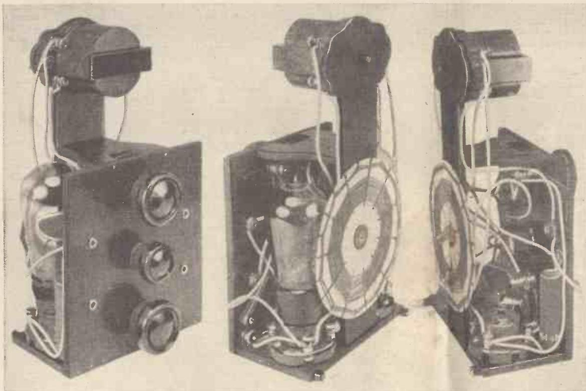
How the components are arranged on the wooden framework is very clearly shown by these three photographs. The low-frequency transformer is screwed to the shaped end-piece. Note the position of the basket coil
