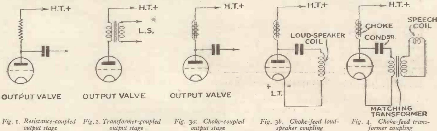
Fig. 1. Resistance-coupled output stage
