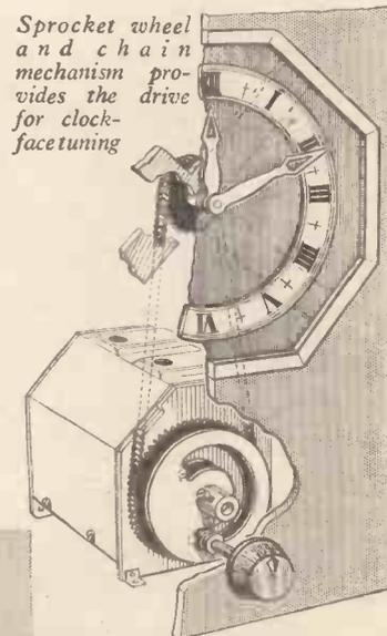
Sprocket wheel and chain mechanism provides the drive for clock-face tuning
