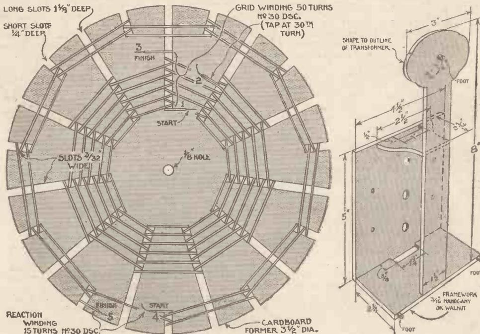
All you need to know for the basket coil, which is home wound as explained in the article. Note the double series of slots: one for the tuning and the other for reaction. This sketch is actual size
