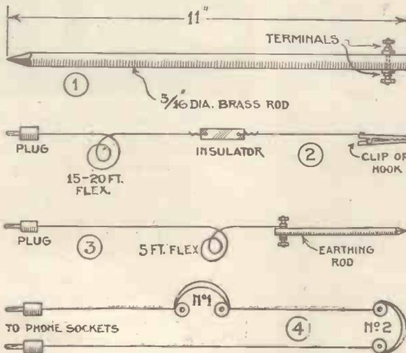
Fig. 1.—Earthing rod to go inside attaché case. Fig. 2.—Suitable aerial arrangement. Fig. 3.—Connecting the earth rod. Fig. 4.—Connecting two pairs of headphones in series for two people to listen
