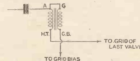
Fig. 4.—Reversing connections to transformer primary
