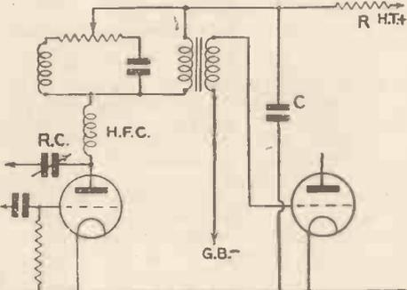
Fig. 2.—Circuit with capacity reaction
