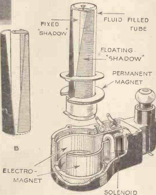
How the Weston tuning indicator is arranged. At A the fixed and moving "shadow pieces" are in the maximum position and at B they are in the minimum position. On the right three positions of the indicator are shown
