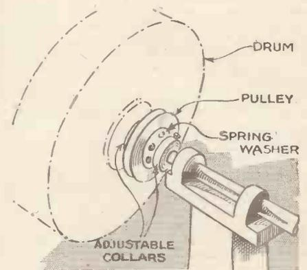
Fig. 3.—A type of mechanical filter favoured in Germany; it employs a slipping clutch
