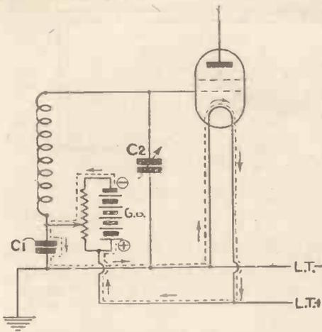
How a valve can be burnt out if grid-bias positive is connected to low-tension positive (see "Grid Battery Plays Up")
