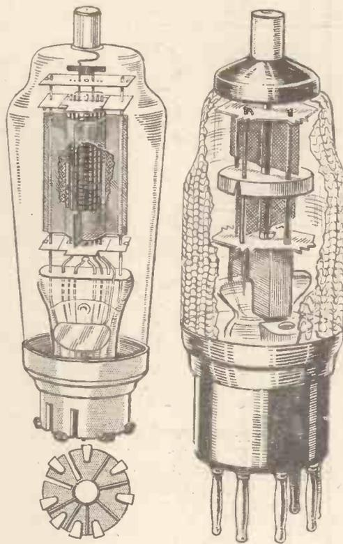
(Left): Mullard type DB26 26-volt output valve. (Right): Ostar-Ganz B2 A.C./D.C. valve for universal mains sets
