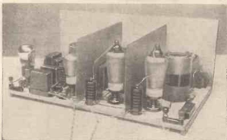
Here is a set for the real radio fan. Home-made components and two screen-grid stages—the Lucerne Major
