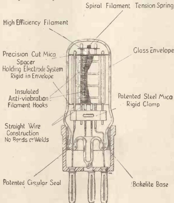
How the Catkin rigid electrode construction has been applied to the K valves for battery operation
