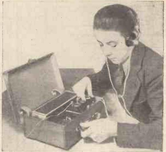
Tuning in the local station during an early test of the Hiker's Headphone Portable. A short indoor aerial wire was used, without any earth
