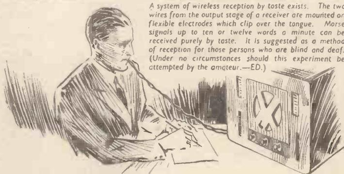
A system of wireless reception by taste exists. The two wires from the output stage of a receiver are mounted on flexible electrodes which clip over the tongue. Morse signals up to ten or twelve words a minute can be received purely by taste. It is suggested as a method of reception for those persons who are blind and deaf. (Under no circumstances should this experiment be attempted by the amateur.—ED.)
