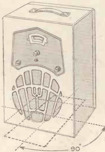
After the set has been tuned, it should be rotated through an arc of 90 degrees in order to find the position of maximum sensitivity
