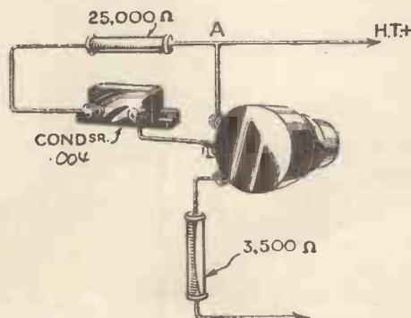
Fig. 2.—Addition of a .004-microfarad by-pass condenser to give mutual balance
