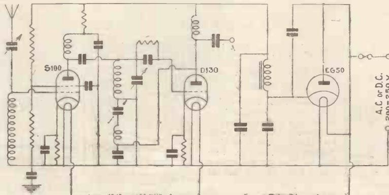
Circuit of Universal High-voltage Radio Converter illustrated above
