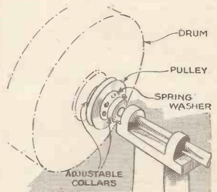
Fig. 3.—A type of mechanical filter favoured in Germany; it employs a slipping clutch
