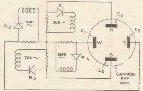
Fig. 3.—Cathode-ray receiver
