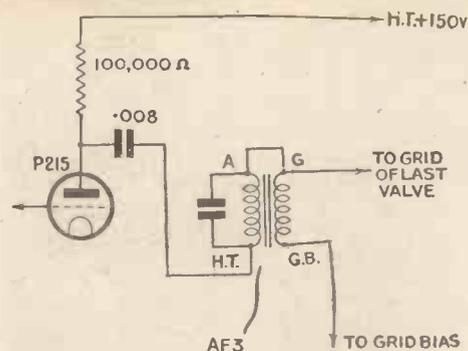
Fig. 2.—Coupling between second and third low-frequency valves
