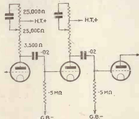
Fig. 1.—Two stages of low-frequency coupling in which the special coupling of the first stage is repeated in the next. The result would be very poor indeed
