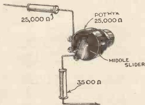
Fig. 1.—Use of three resistances in series, two fixed and one variable
