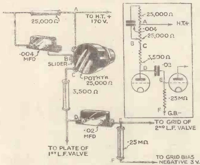
Fig. 3.—Complete circuit of the low-frequency coupling recommended by Noel Bonavia-Hunt
