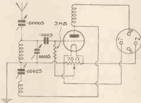
Circuit of simple short-wave plug-in adaptor
