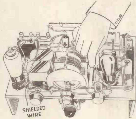
"In some cases the aerial wire itself is housed in the middle of an earthed tube made up of braided wire"
