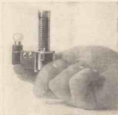
Light from the bulb shines through a triangular opening in the tube, a moving shutter varying the size of the triangle of light thus formed
