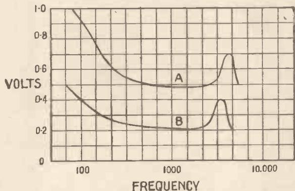
Fig. 1.—Characteristic curves of two imaginary pick-ups according to a voltage scale
