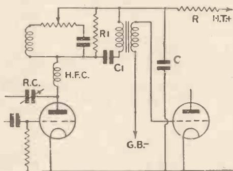
Fig. 3.—Tone-control as applied to a parallel-feed circuit
