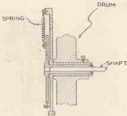
Fig. 1.—Here is a simple type of mechanical filter of the kind used by the Baird Co.
