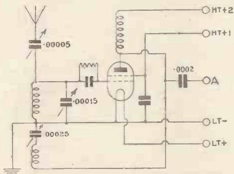
Circuit of simple short-wave super-het converter
