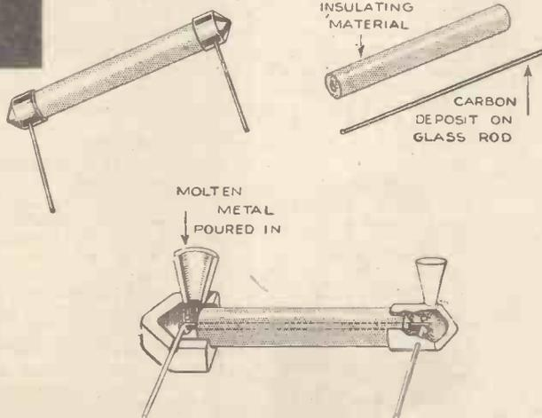
How Dubilier resistances are made. The mould shown in the lowest sketch is simply the artist's impression of what the inside shape is like. The cone piece corresponding to the funnel is knocked off
