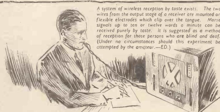
A system of wireless reception by taste exists. The two wires from the output stage of a receiver are mounted on flexible electrodes which clip over the tongue. Morse signals up to ten or twelve words a minute can be received purely by taste. It is suggested as a method of reception for those persons who are blind and deaf. (Under no circumstances should this experiment be attempted by the amateur.—ED.)
