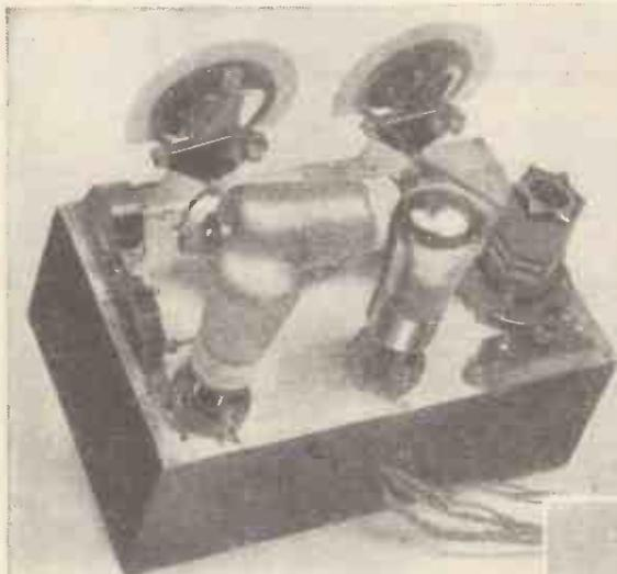
No space wasted here! See how the screen-grid valve is mounted on its side?
