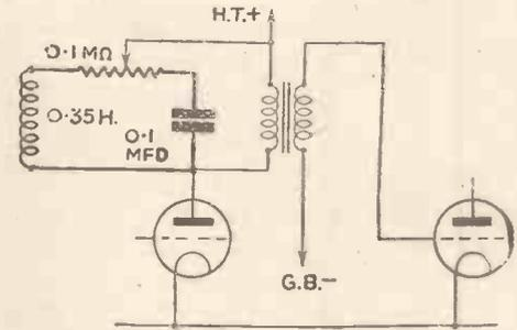
Fig. 1.—Tone control applied to circuit with direct transformer connections
