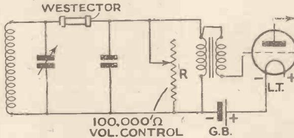
Fig. 1.—The only form of volume control permitted in a real quality receiver is the variable resistance R shown above in the circuit diagram
