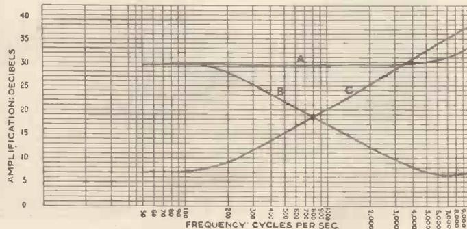
Fig. 4.—Results obtained with tone control in circuit
