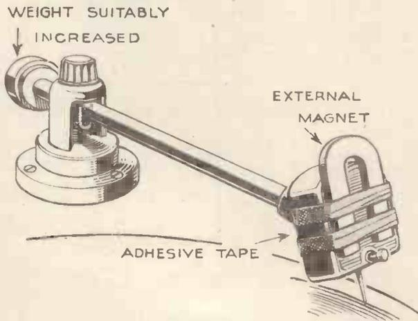
How an extra horseshoe magnet can be fixed to an old pick-up to increase its sensitivity
