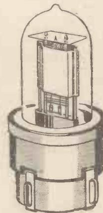
The glass bulb is actually not much bigger than a fountain-pen cap—and the diameter is in the same proportion. Ideal, obviously, for midget sets—and don't forget these valves are available to the amateur.
