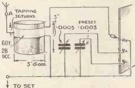
Theoretical circuit of the whistle filter—which can also be used as a wavetrapp
