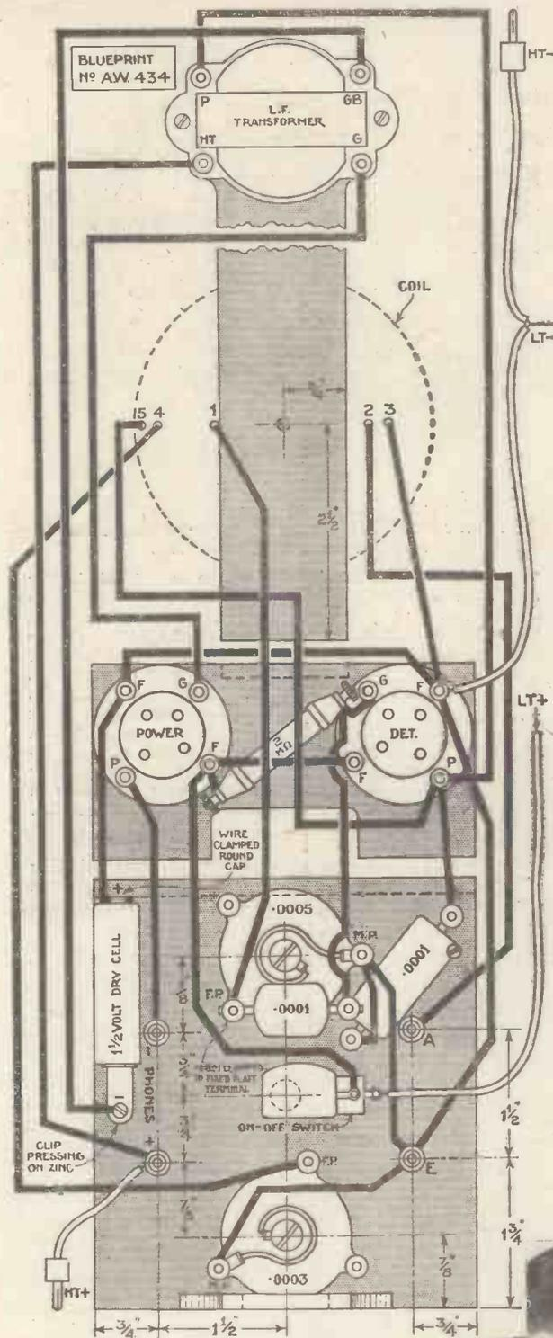
Half-scale reproduction of the blueprint of the Hiker's Portable. The full-size print can be obtained price 1s., post paid. (No. A.W. 434). It gives all the component dimensions and the point-to-point wiring
