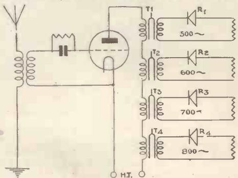
Fig. 2.—Receiver circuits arranged with tuning-fork selectors
