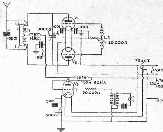
Fig. 3. Speech transmitter for 5-metre working
