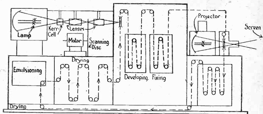
An endless film is used at the receiver also, the picture being impressed upon it as it passes in front of the scanner
