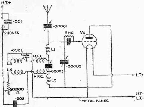
Fig. 1. Simple super-regenerative detector circuit using home-made coils
