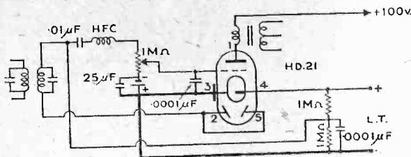
SIMPLE DIODE DETECTOR WITH BATTERY-BIASED TRIODE (DIODE BIASED TO (+) POSITIVE)
