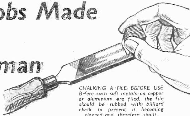
CHALKING A FILE BEFORE USE Before such soft metals as copper or aluminium are filed, the file should be rubbed with billiard chalk to prevent it becoming clogged and, therefore, spoilt.
