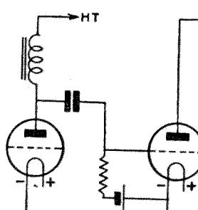
Fig. 3.—Choke-capacity coupling
