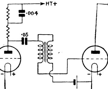
Fig. 8.—Partially-shunted anode resistance parafeeding
