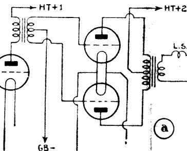
Fig. 6a.—Push-pull transformer coupling
