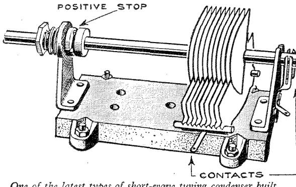
One of the latest types of short-wave tuning condenser built up on a Steatite base
