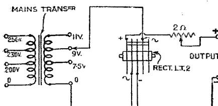
Theoretical circuit diagram of the charger, showing fuses, transformer, metal rectifier and output terminals
