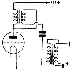
Fig. 7.—Auto-transformer-fed auto-transformer coupling
