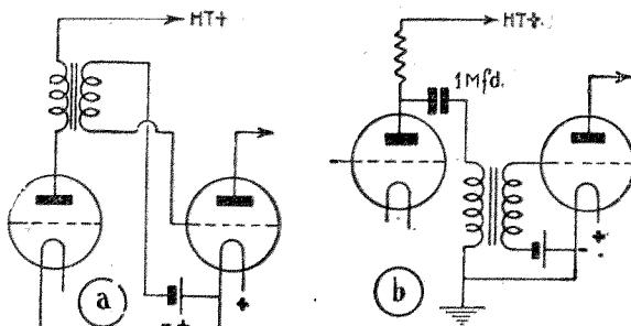
Fig. 1.—Transformer coupling, direct (a) and parallel-fed (b)
