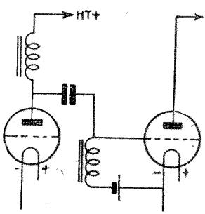
Fig. 4.—Dual-impedance coupling
