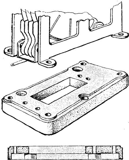
Low-loss Steatite base for short-wave variable condenser
