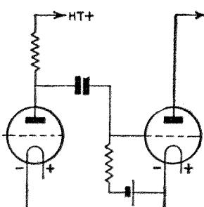
Fig. 2.—Resistance-capacity coupling
