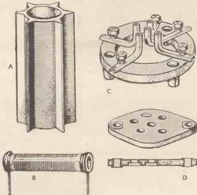
(A) Ribbed former for short-wave coils. (B) Ultra-short-wave high-frequency choke. (C) Low-loss valve holder. (D) Component parts of chassis-mounting valve holder for short waves
