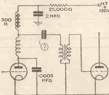
Fig. 2. Don't forget that when using a parallel-fed transformer a big condenser does not always mean more bass
