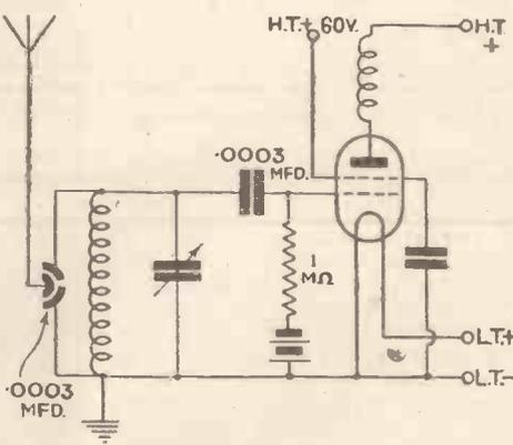
Fig. 3. This is how we are now using variable-mu screen-grid valves. Note the differential volume control
