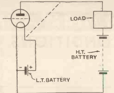
Fig. 1. Simple circuit showing current path in a valve circuit—following, it should be noted, the old convention
