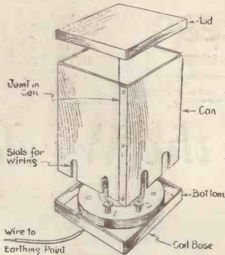
Fig. 4.—Completed can. It should be noted that the bottom piece is fixed underneath the coil base, with a wire gripped underneath for earthing to the chassis
