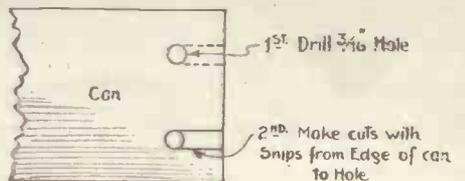
Fig. 3.—Follow this method for making neat slots in cans for the wiring connections
