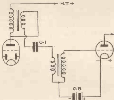
Fig. 2.—Special method of coupling between diode-triode and output valves
