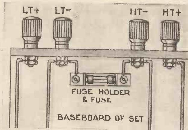
Typical fuse between high-tension negative and low-tension negative—fitted inside the set
