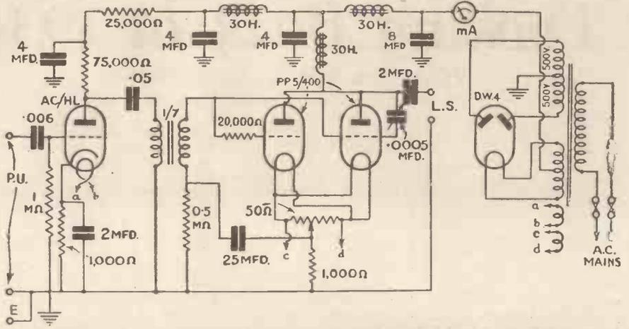
Fig. 5. Circuit of our A.C. amplifier, very simple considering it gives an output of 11 watts
