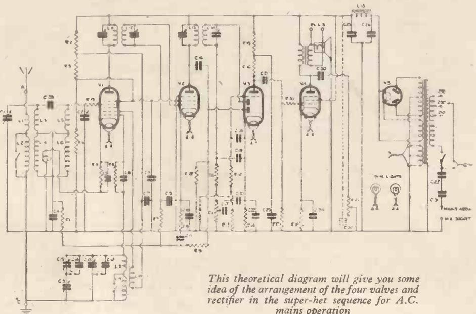
This theoretical diagram will give you some idea of the arrangement of the four valves and rectifier in the super-het sequence for A.C. mains operation
