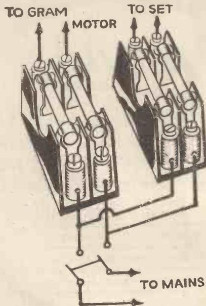
Twin fuses arranged for motor and set of a radio-gramophone on the instrument side of the mains-input switch
