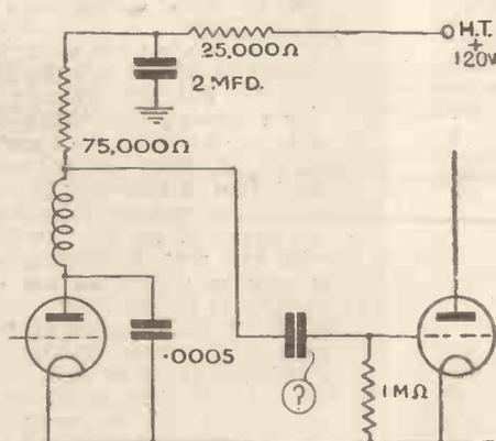
Fig. 1. Suggested resistance-capacity-coupled circuit with critical coupling condenser
