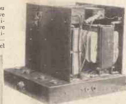
See how the power pack is kept to one side in the A.C.-mains amplifier, with division across the centre of the can
