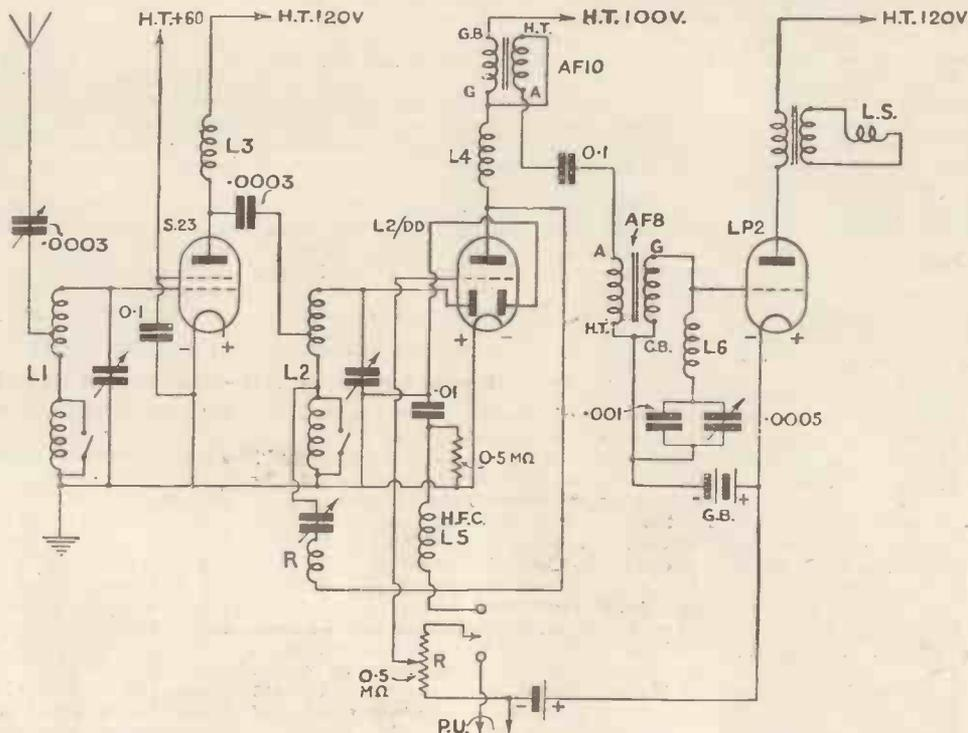
Fig. 1.—Circuit of three-valver battery set for real quality, suggested by the author. A list of recommended parts appears above
