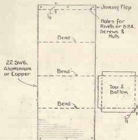
Fig. 1.—Layout of metal for square can—the top and bottom being separate pieces
