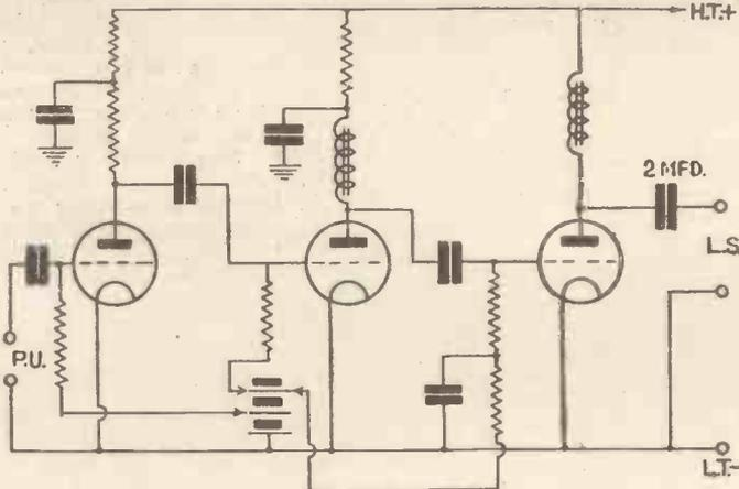
Fig. 4. Battery-operated amplifier, the main values for which are given in the article
