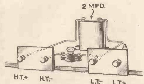
Fig. 2. Sometimes this fuse arrangement will "blow" every time the set is switched on, as explained in the article
