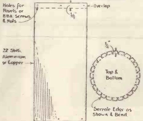
Fig. 2.—Layout of metal for circular can—the top and bottom being separate pieces
