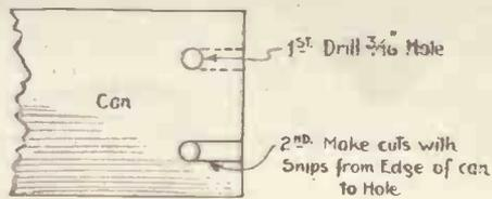
Fig. 3.—Follow this method for making neat slots in cans for the wiring connections
