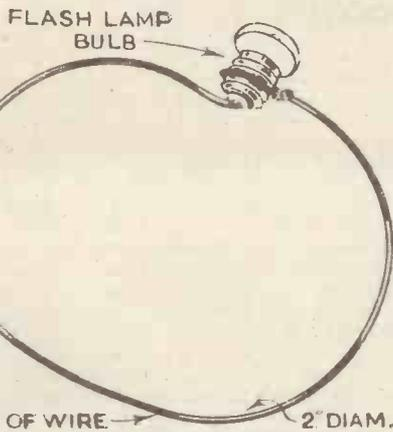
If a loop of wire is connected to a bulb it will light up brightly when brought near a transformer
