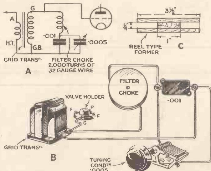
Fig. 3.—Details of whistle filter for quality set: A, circuit; B, diagrammatic connections; C, dimensions of former
