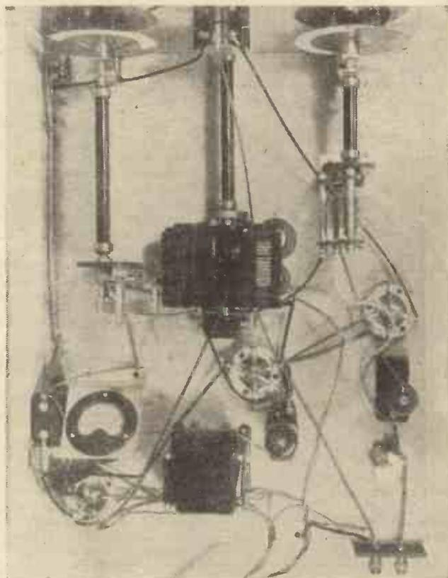
Plan view of the hook-up, showing how the all-wave coil and other components are arranged on the baseboard
