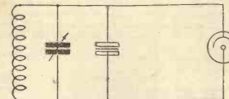
Fig. 3.—Neon-cum-crystal circuit for transmitting
