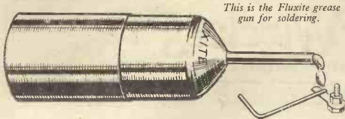
This is the Fluxite grease gun for soldering.
