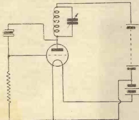
Fig. 1.—Quartz crystal across grid and anode of a valve
