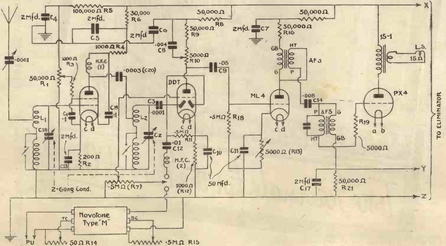
Fig. 1.—Complete circuit of real-quality three-valve A.C. radio gramophone
