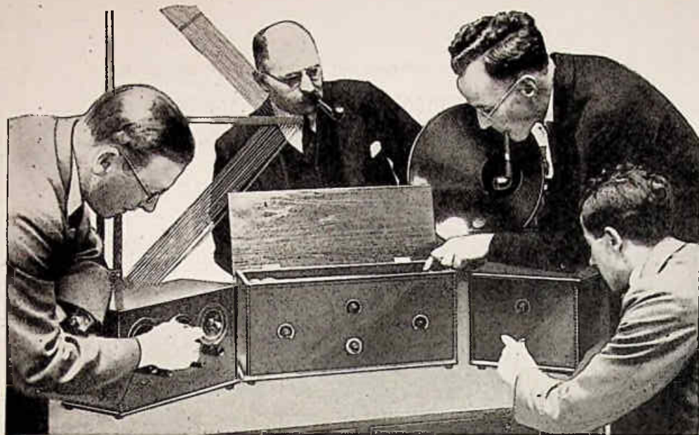
Fig. 34.—Testing the Three-unit Super-het. Note the Frame Aerial on the left
