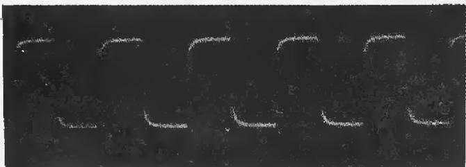
Fig. 12. Square-wave response, 10 kHz and 0.1- $\mu$ F load.
