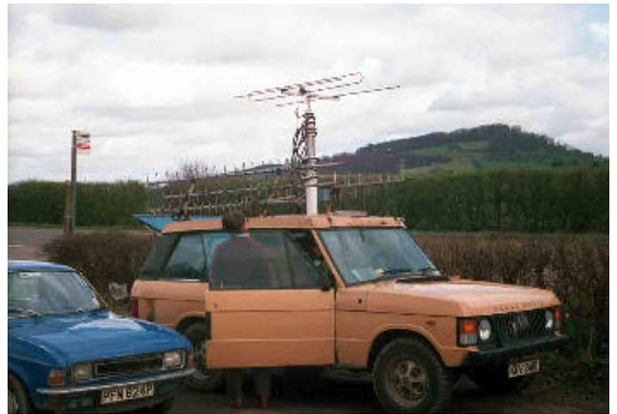
verify the predicted service area. *(Above Alun Maddocks is checking the antenna on the borrowed Range Rover)* Unfortunately the new transmitters caused interference to listeners of the Pontypool VHF relay station and so the service was temporarily closed down after a week. The problem was eventually cured by changing the frequency of the smaller Pontypool relay.
