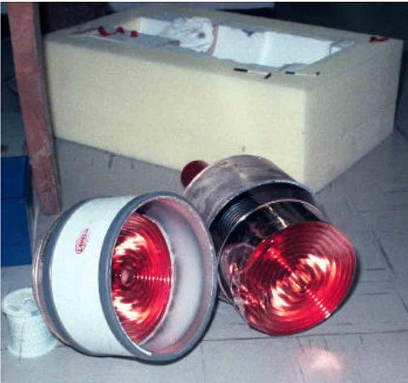
Then a small disaster occurred when both S81 and S82 both blew holes in the HT cable to the Penultimate stage due to excessive RF on 21 MHz. Marconi came back with a modification and all senders were done. It also became apparent that the previous purchasers of these senders had
