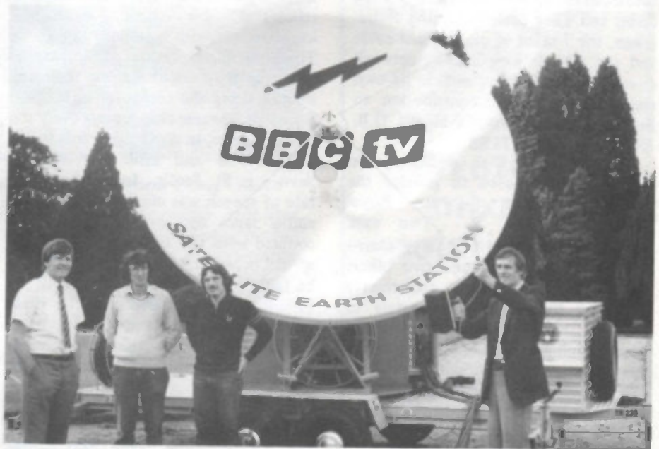
'Project manager Malcolm Harman (right) checks for radiation hazards around the periphery of the transmitting dish during acceptance tests at Kingswood Warren, with (from left to right) Trevor Denham (TVOBs), Derek Hodge and Chris Gandy (satellite team, RD).'
