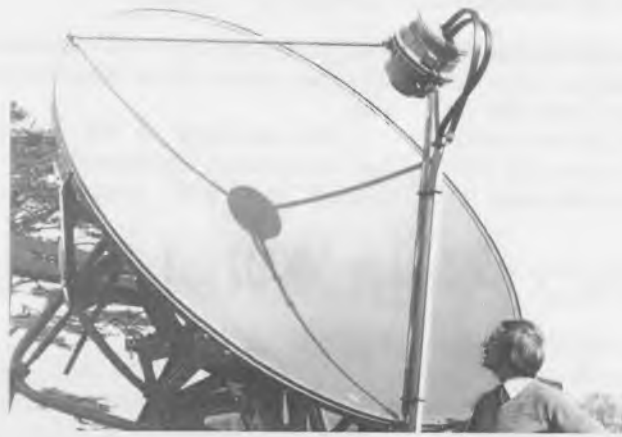
2.4 metre Multi-polarization Receiving Dish at R.D. for OTS
