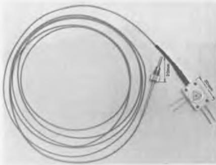
*Optical fibre cable, laser and a ferrule connector.*
