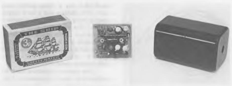
Single limiter (centre) with case (right) for holding two for stereo.
