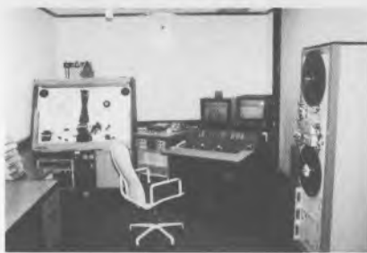
News Telecine 1 showing the Rank Cintel Mk III machine and Schlumberger sepmag facility
