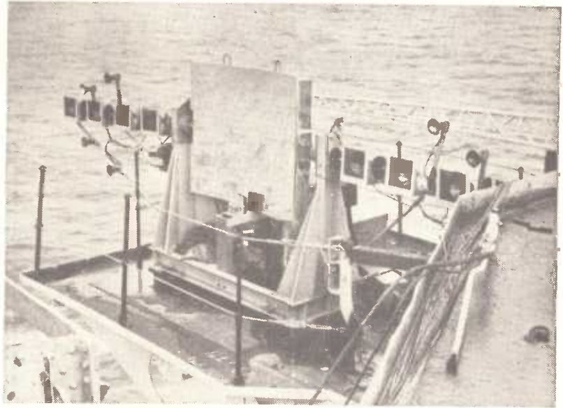
With the optical system the pilot landing on a carrier keeps the image of a reflected light in the centre of this concave mirror for a perfect touchdown
