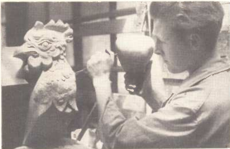
A mason fashions a gargoyle for York Minster: the stone is very workable and is consequently much used for sculptured masonry
