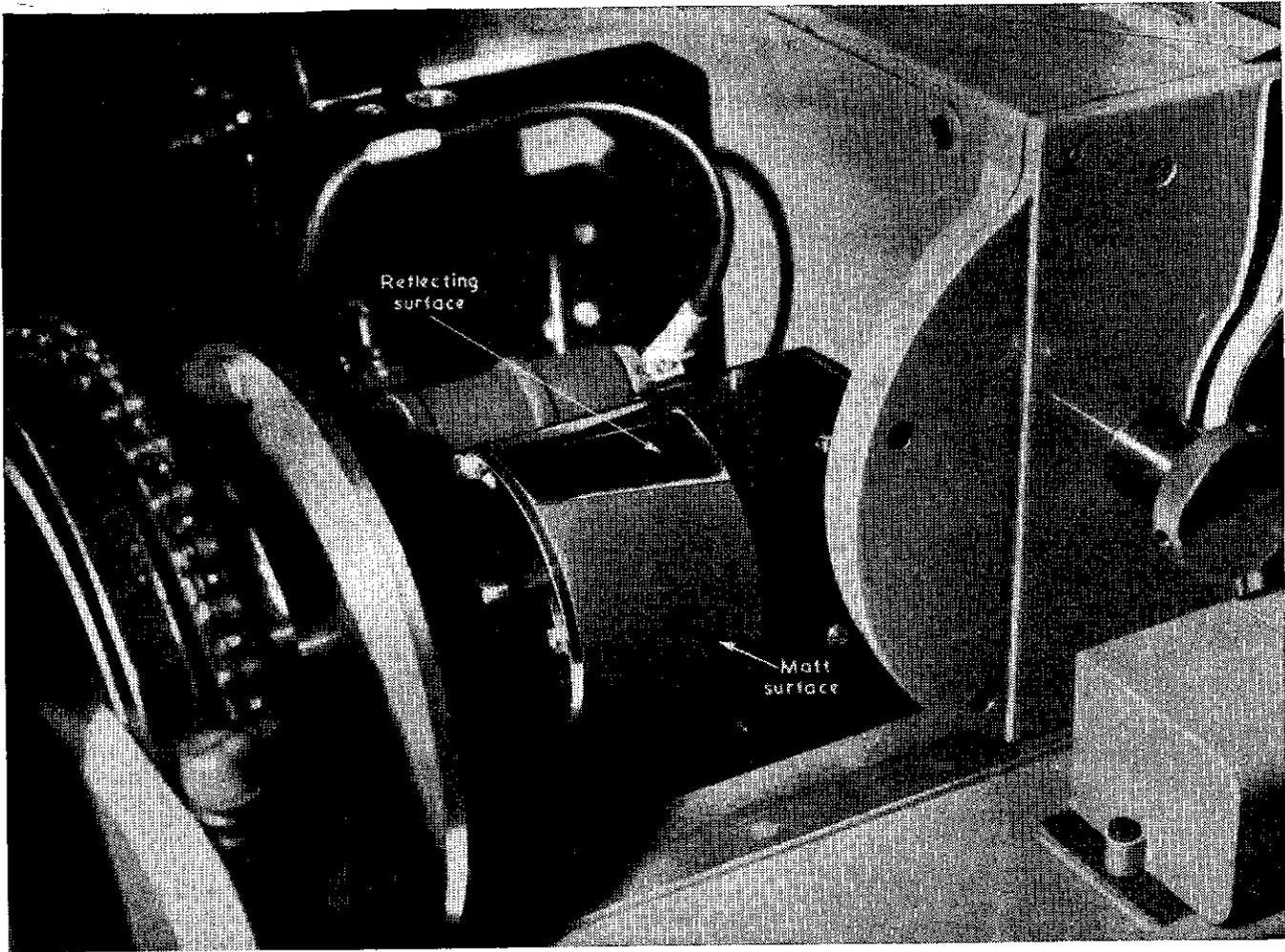
Fig. 2 — Mirror-drum assembly for television frame suppression
