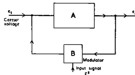
Fig. 9 — Method of taking the reciprocal of a signal
