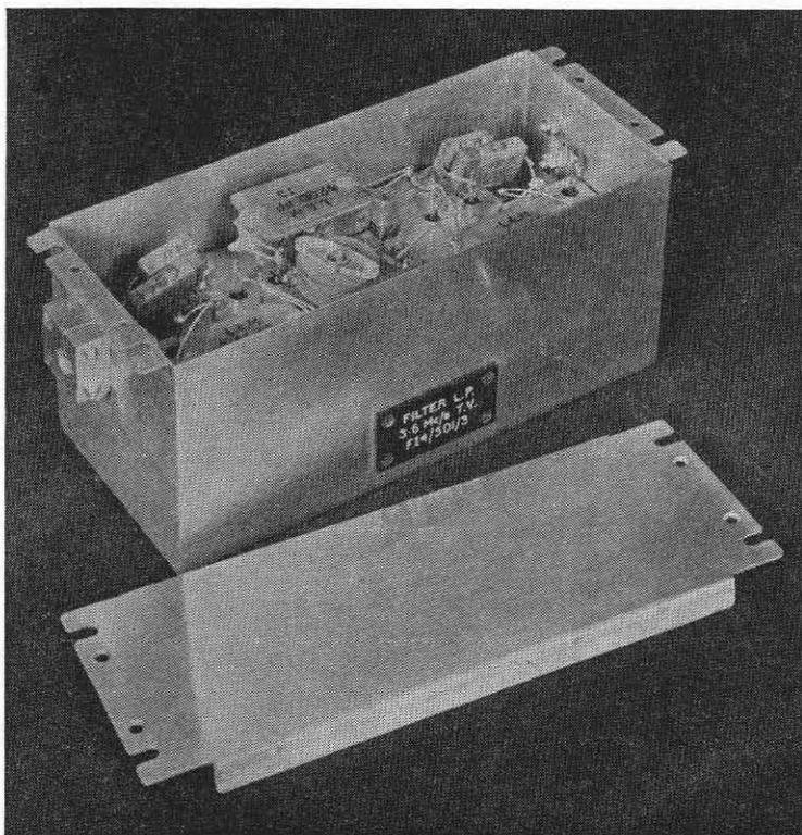
*Fig. 12 — Filter mounted in can*
