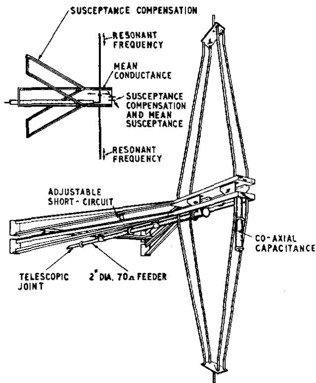
Fig. 3 — Single-dipole element for upper half of aerial
