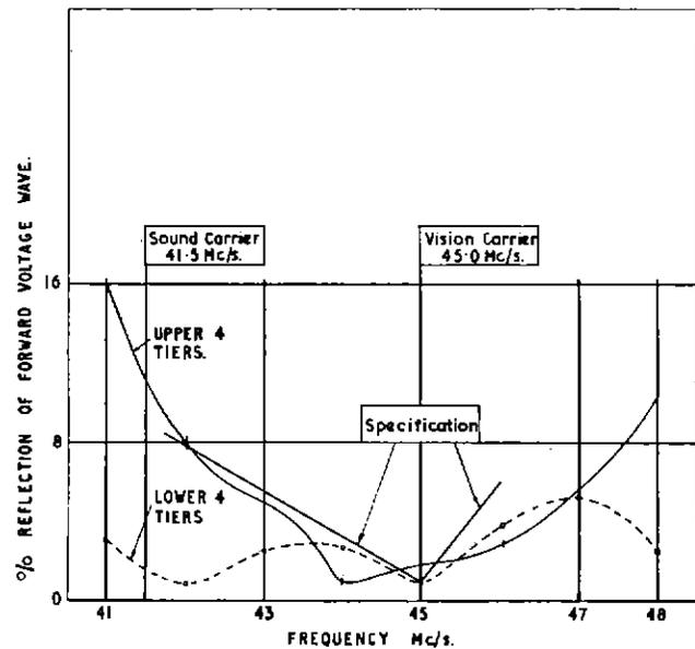
Fig. 9 — Reflection coefficients of both halves of aerial
