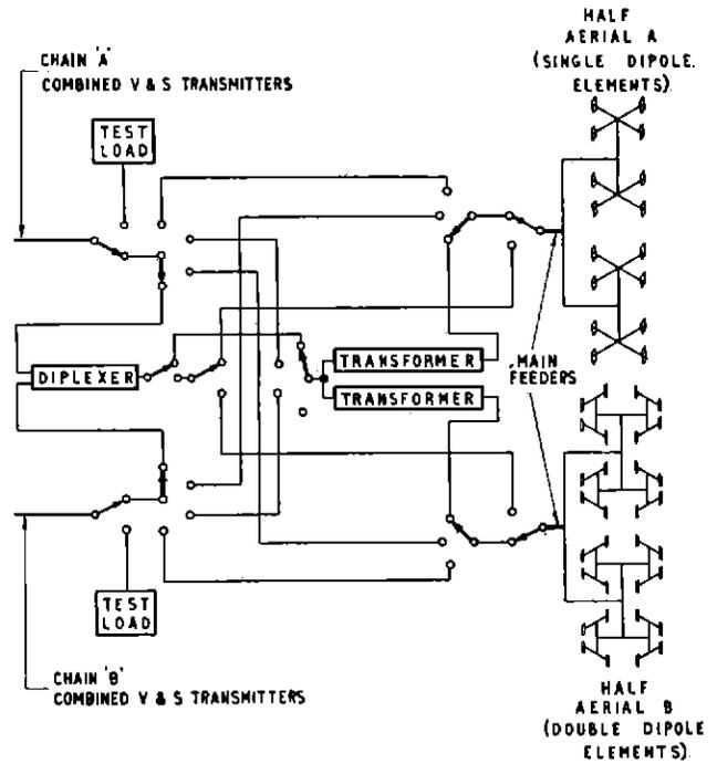
Fig. 2 — Schematic of aerial, feeders, and switching
