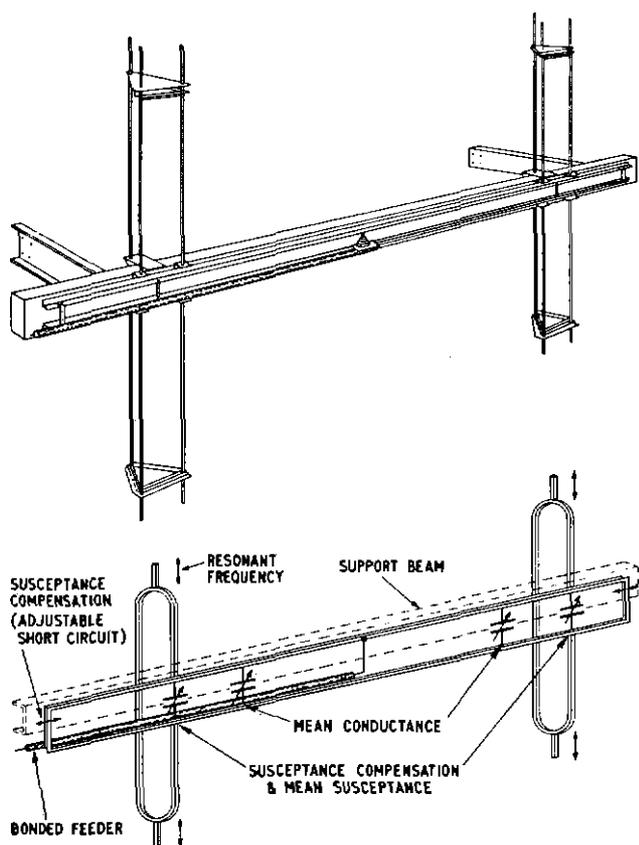
Fig. 4 — Double-dipole element for lower half of aerial
