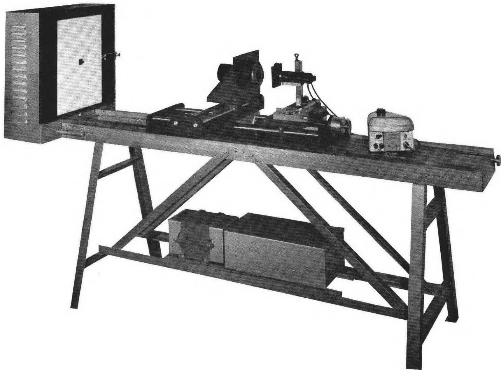
*Fig. 4 — Optical bench constructed for veiling-glare measurement*
