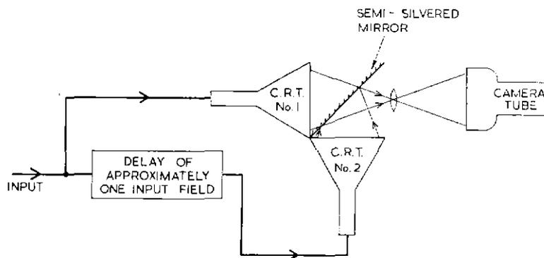
Fig. 13 — A method of obtaining conversion in pictures
