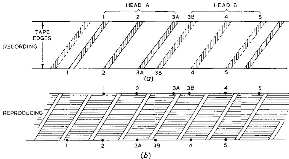
Fig. 14 — N.H.K. field-frequency converter using helical magnetic recorder
