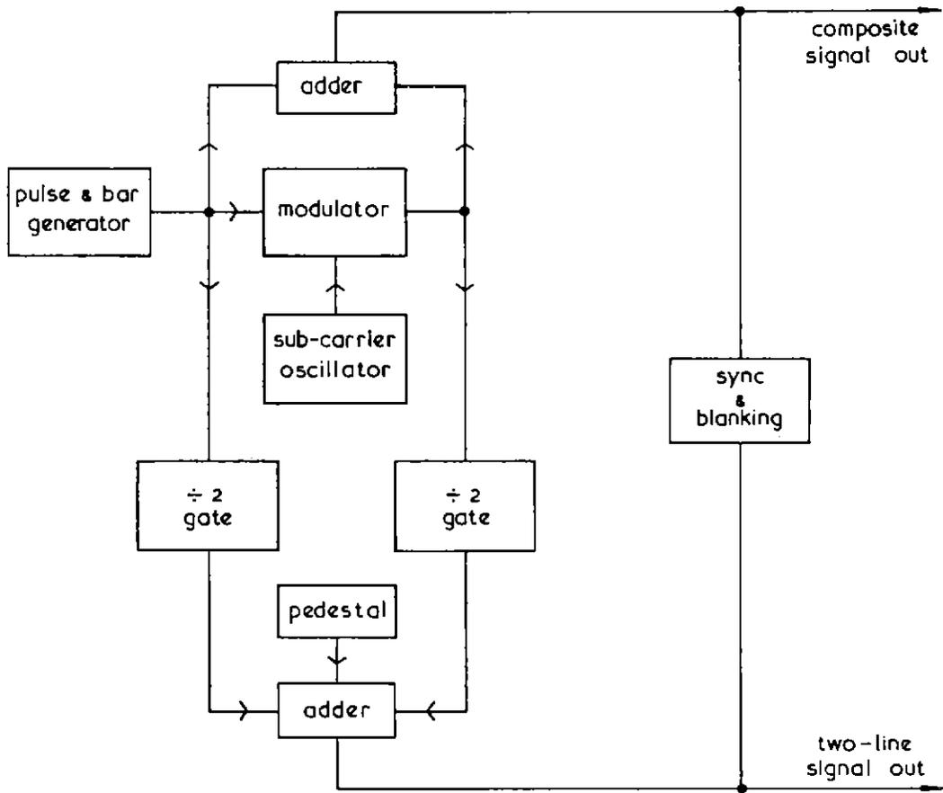
Fig. 7 — Functional schematic of experimental generator
