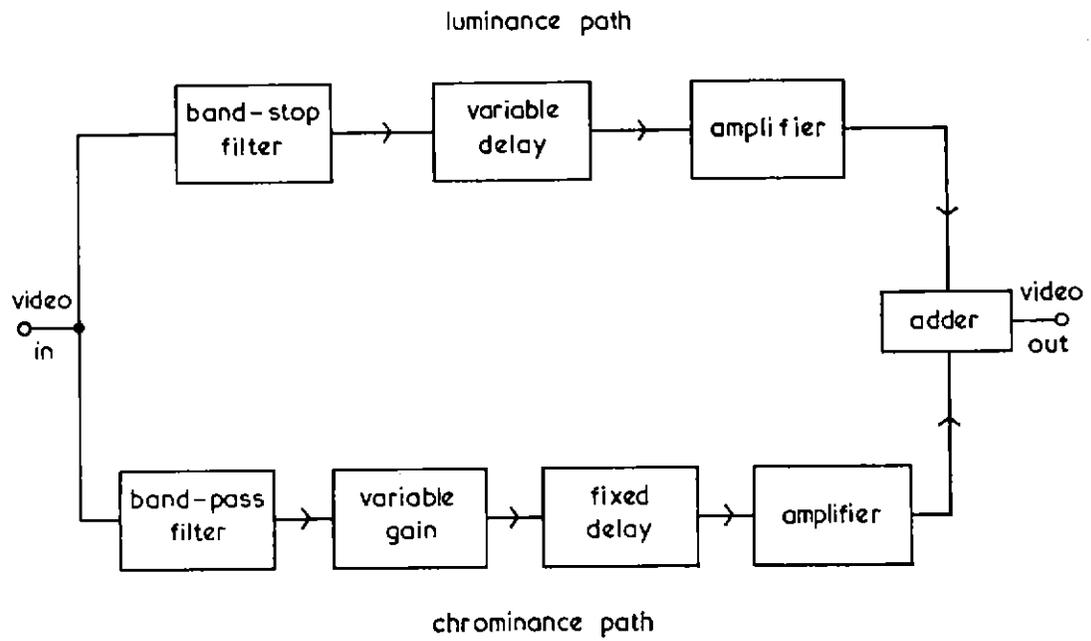
Fig. 8 — Functional schematic of measuring unit
