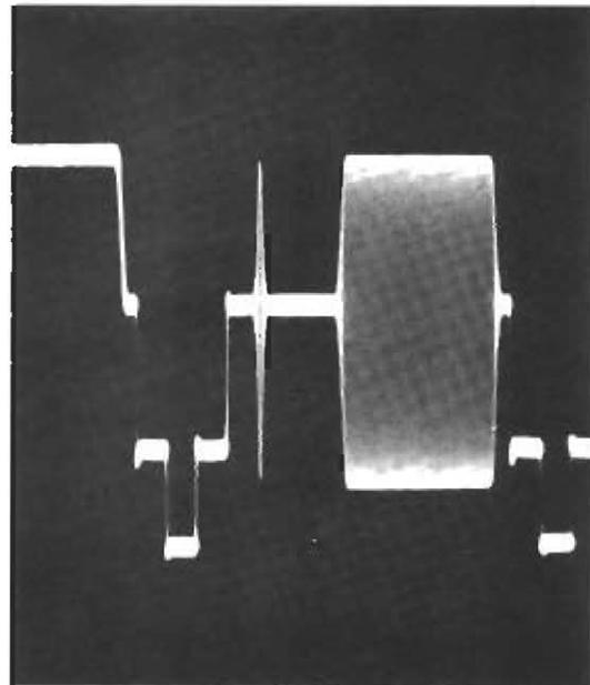
*Fig. 12 — Two-line signal after modulation and envelope demodulation*
