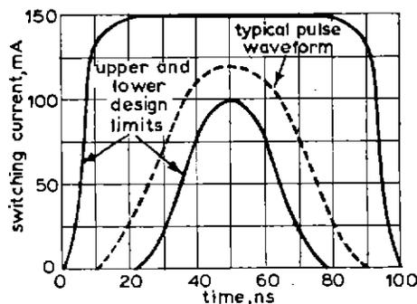
Fig. 6 — Design tolerances for the switching pulse
