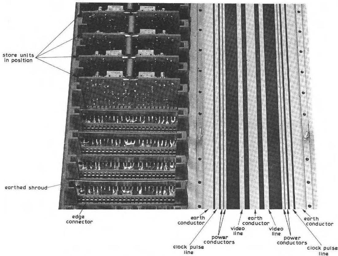
Fig. 17 — Store assembly layout using strip transmission-lines
