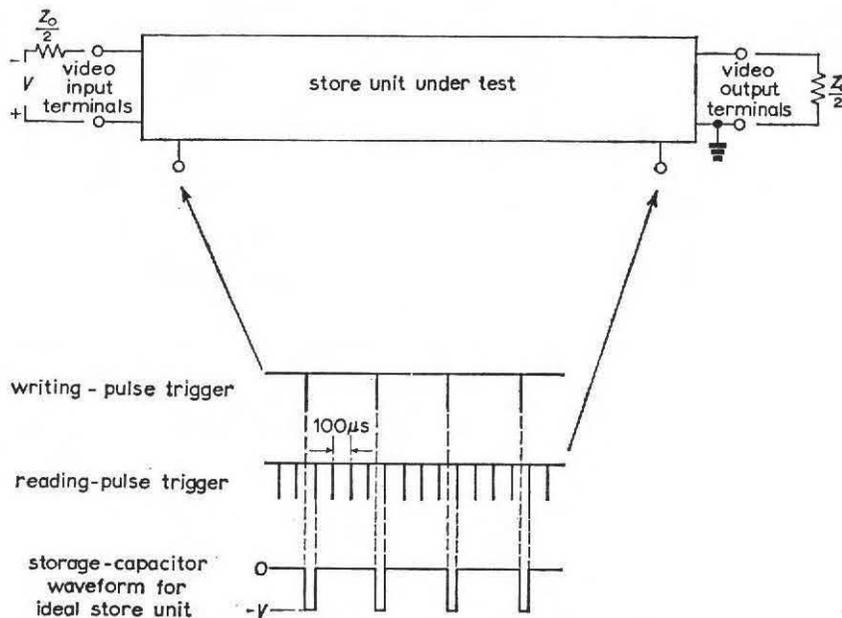
Fig. 8(a) — Testing arrangements for store units
