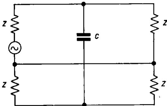
Fig. 13 — Equivalent circuit showing inter-line capacitance
