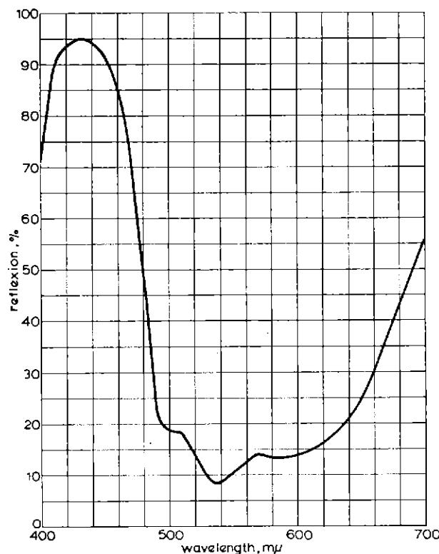
*Fig. 10 — Spectral characteristics of the blue-reflect dichroic mirrors
