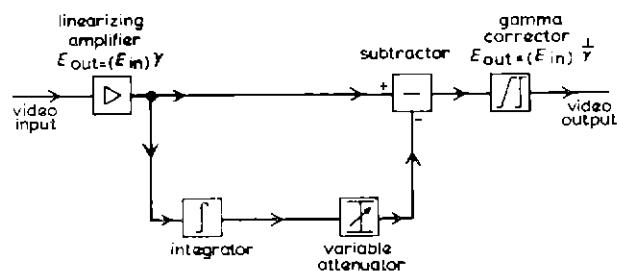
Fig. 13 — Illustration of a veiling-glare corrector
