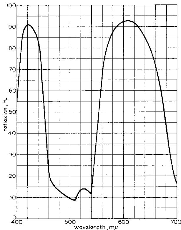
Fig. 9 — Spectral characteristics of the red-reflect dichroic mirror
