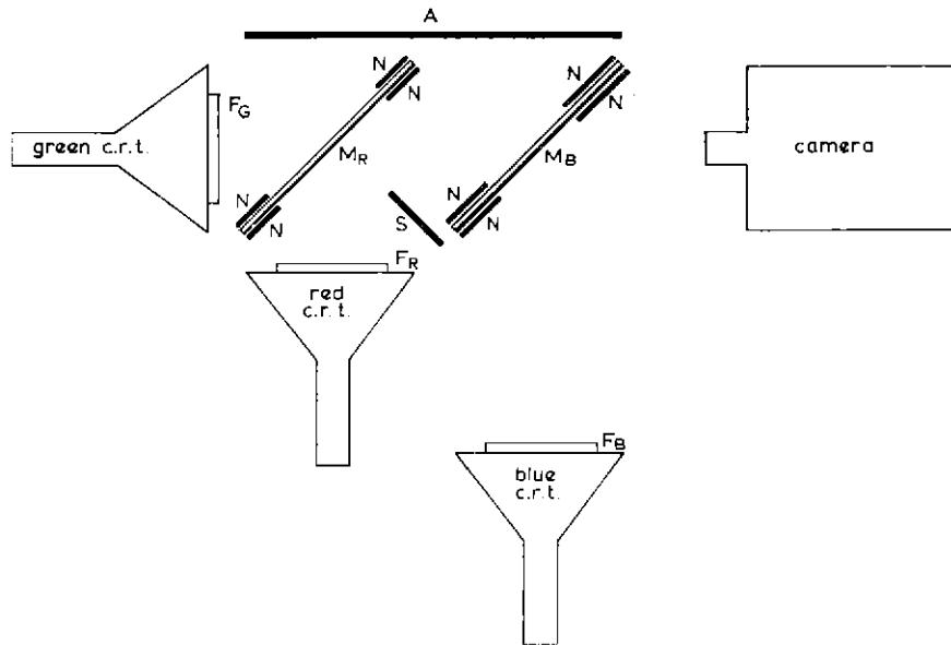
$F_R, F_G, F_B$ —Absorption-type shaping filters
