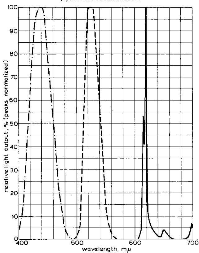
*Fig. 11 — Spectral characteristics of the light from the three colour-separation channels
