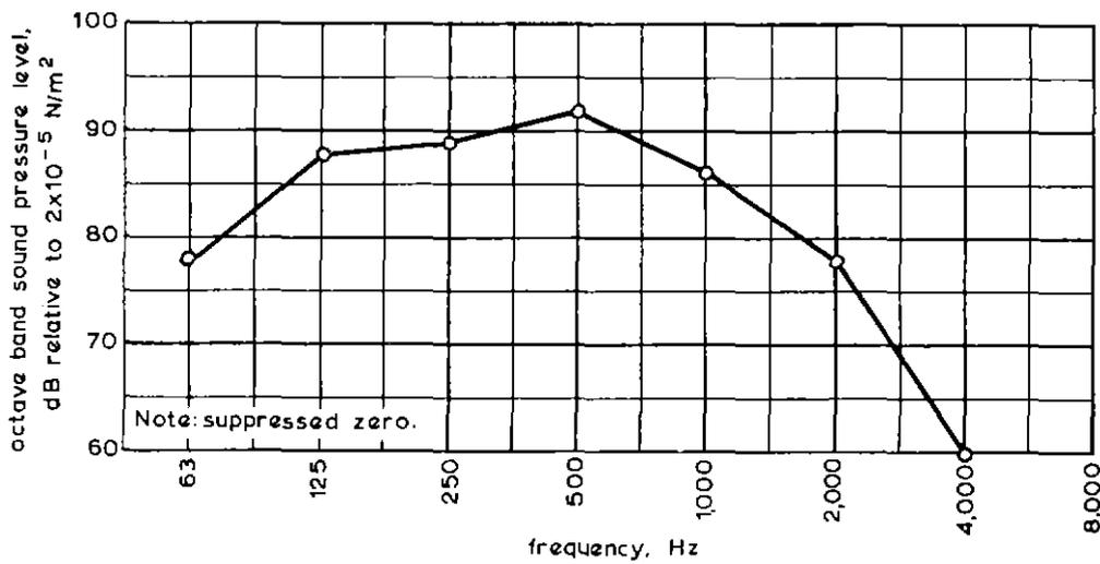
Fig. 15 — Aircraft noise levels measured at BBC Television Centre 21-25 March 1966
