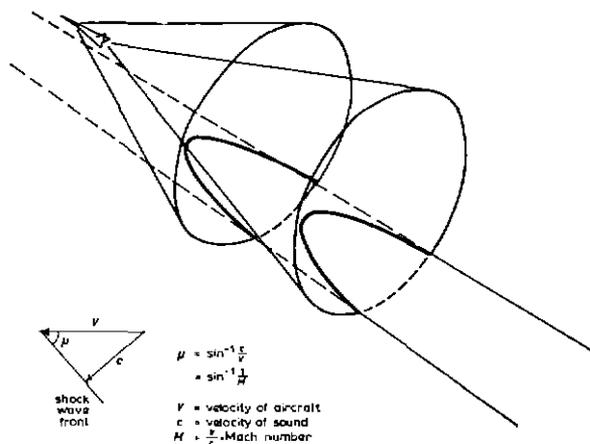
Fig. 3 — Aircraft shock waves intersect ground in hyperbolae which sweep over the ground
