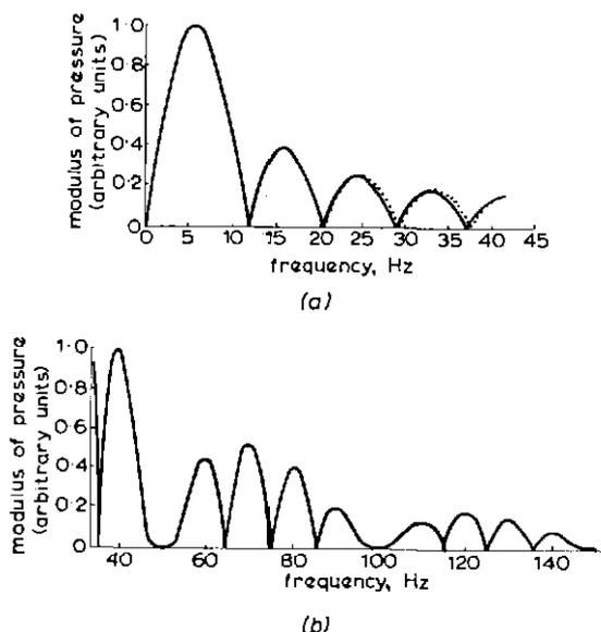
Fig. 4 — Amplitude spectra of 'N'-waves of duration 120 ms
