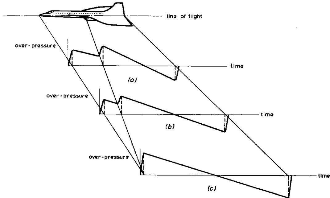
Fig. 1 — Pressure distribution in a shock wave from a supersonic aircraft
