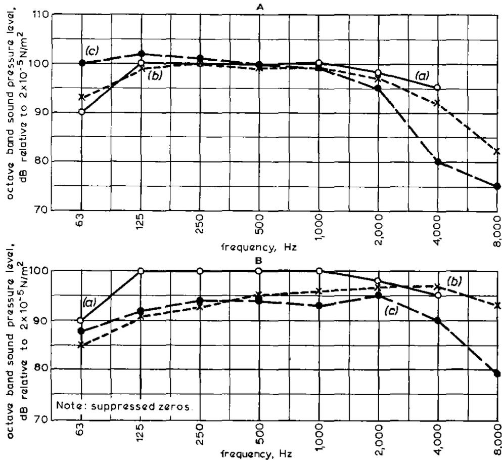
Fig. 11 — Aircraft noise spectra
