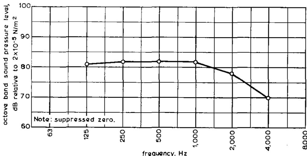
Fig. 16 — Noise levels produced by S61N helicopter distant 120 m
