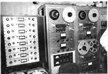
Lansdowne 8 track machine on the left with playback panel on the right.
