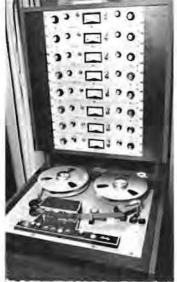
Note the wide tape necessary for 8 track recording.
