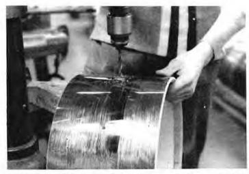
At Pullman Road, the finished drum shells are drilled for their fittings. The polyester finish has already been applied.
