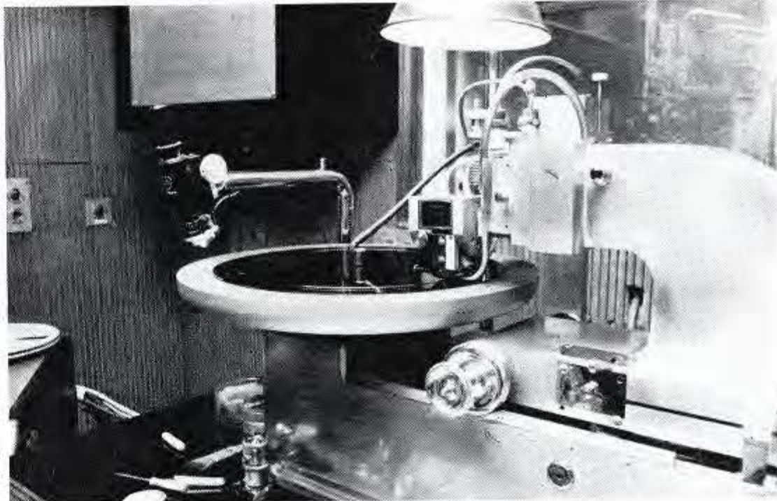
Pye studios' stereo cutting machine in operation—a morning's session can be on disc by the afternoon
