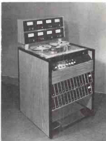
Leavers-Rich eight-track recorder with channel selection logic control circuitry.
