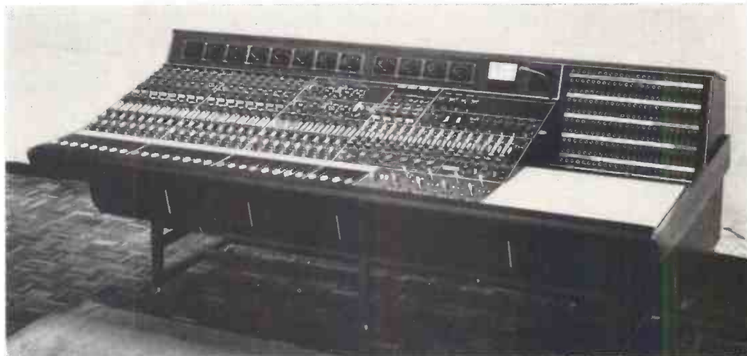
Neve 16-channel with quadraphonic pan facilities, built and designed for Eel Pie Studios
