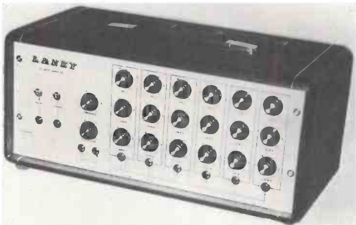
Laney LA100 Super: 100 watt P.A. Mixer/Amplifier
