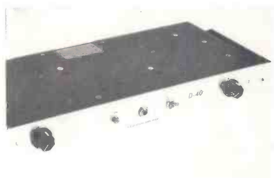
The Crown D-40 Amplifier, rated at 170 watts
