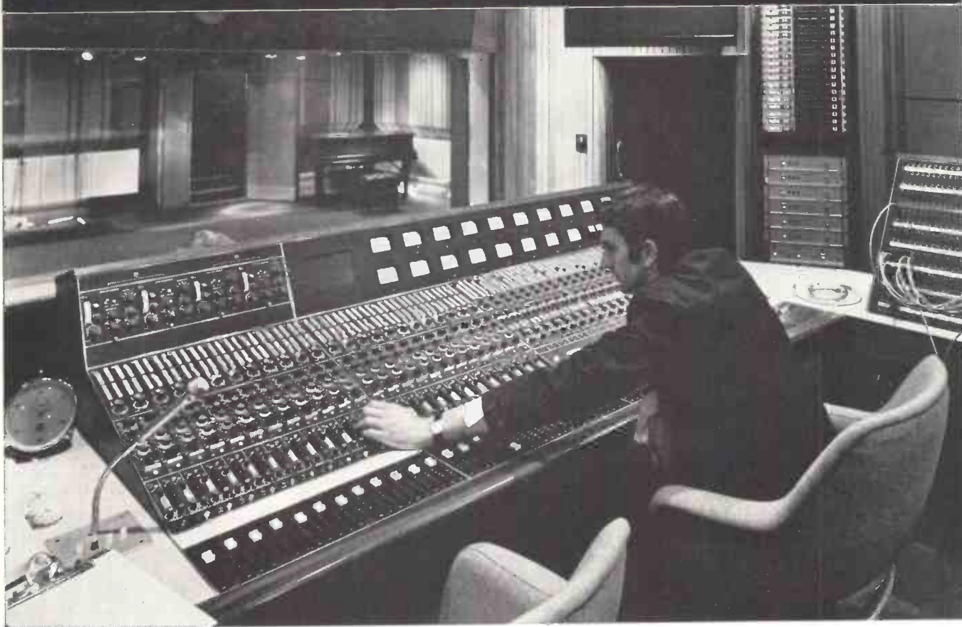
24 input/16 output channel console by Neve for the newly opened Audio International Recording Studios Ltd., London. General manager Richard Millard at the controls.
