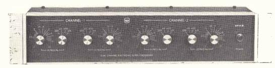
The Amcron VFX-2 provides continuously variable filters which can be used to perform either crossover or band pass functions. The dual channel unit employs two filters per channel, each continuously variable from 20 Hz to 20 kHz. Filter rolloff is at a fixed 18dB/octave.
