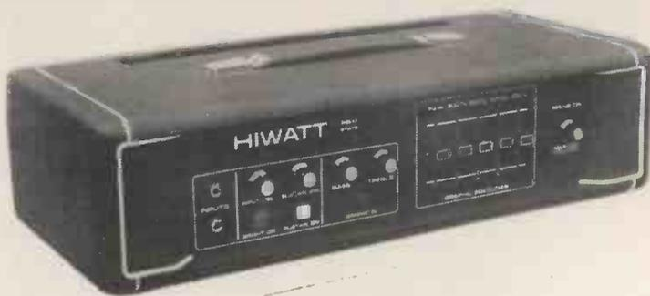
sound similar to that obtained from conventional valve amplification, Hiwatt recommend setting input and master volumes to approximately 2 o'clock, treble and bass to almost full and graphic equaliser in a V-shape. The sustain control can then be brought into play to increase the rough-
