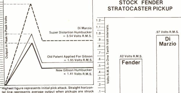
Highest figure represents initial pick attack. Straight horizontal line represents average output when pickups are struck with an Open E Chord in the treble position of a new Les Paul.
