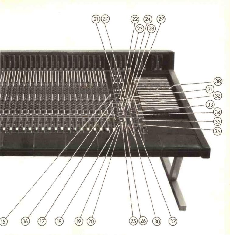
22. Master Programming switches — control the status of all Input/Output modules. There is an "A" group and a "B" group of four buttons apiece, which switch the modules assigned to them to: Source Monitor (recording from desk) — Return Monitor (playback from multi-track Machine) — Return Mix — source Mix.
