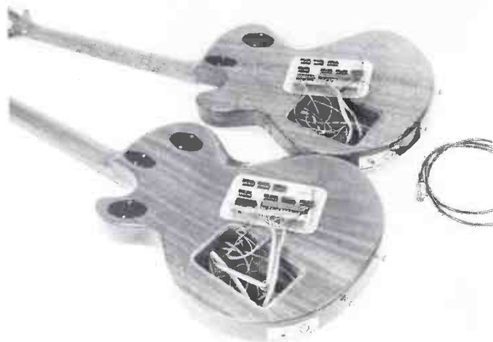
The internal circuitry of the Hagstrom 'Patch 2000' synthesizer guitar showing 4 string bass below and 6 string lead above.
