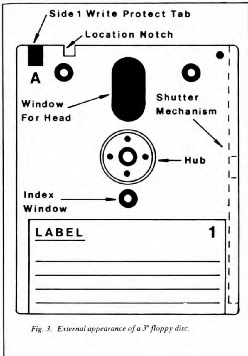
*Fig. 3. External appearance of a 3" floppy disc.*
