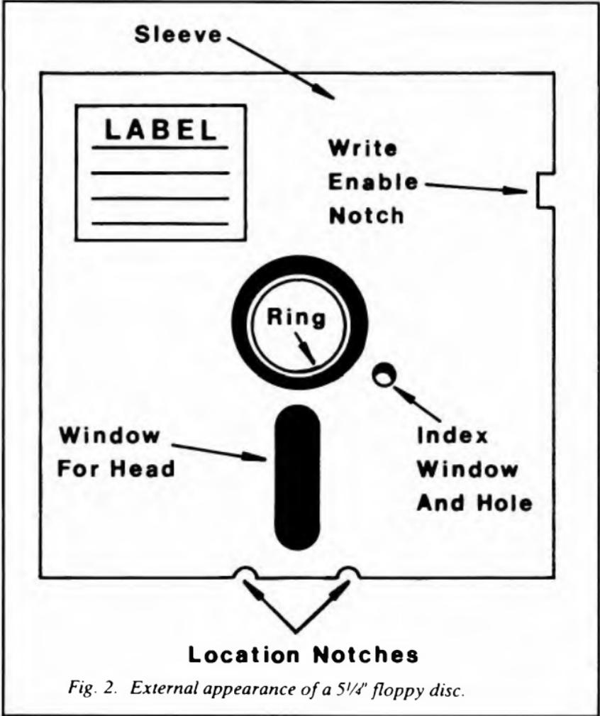
*Fig. 2. External appearance of a 5 1/4" floppy disc.*
