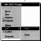
The toolbar (see below) is a very useful feature of an MS-DOS window. You can mark text and copy it to the Windows clipboard, or paste from the clipboard. You can also carry out these functions from the Command menu, by selecting Edit. Mark. Edit. Copy, or Edit, Paste, as shown here.
