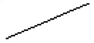
Notice that although it is recognisable as a straight line it's no a very adequate straight line — the ZX81's graphics are good but not that good! To gain confidence, it's a good idea to try out the previous program with various values of M and C. You should discover that M alters the slope of the line and C move it up and down. You should also notice that sometimes you get an error message because for some values of X the Y value is off the screen.
