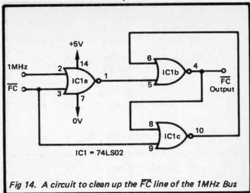
Fig 14. A circuit to clean up the FC line of the 1MHz Bus
