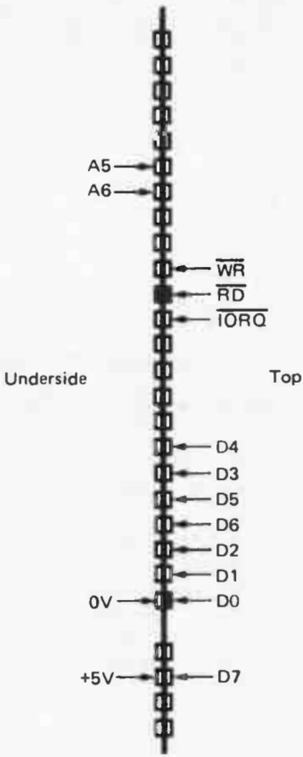
Fig 17. Connection details for the Spectrum's expansion port
