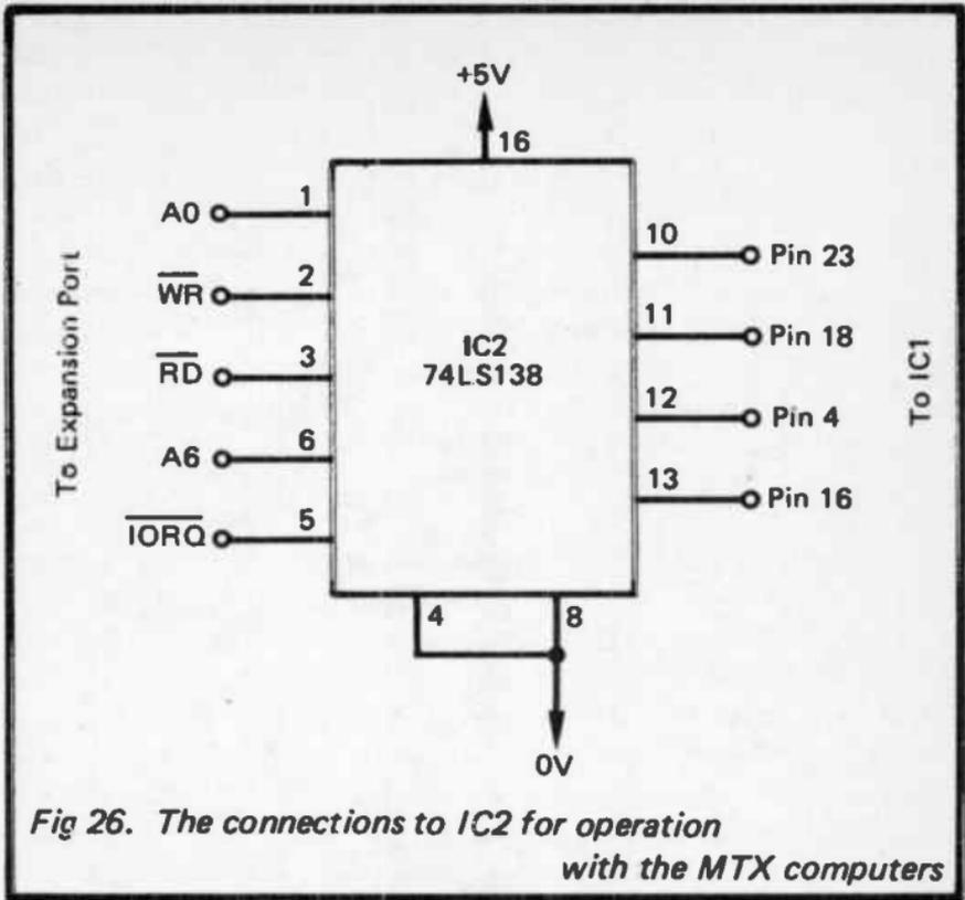
*Fig 26. The connections to IC2 for operation with the MTX computers*
