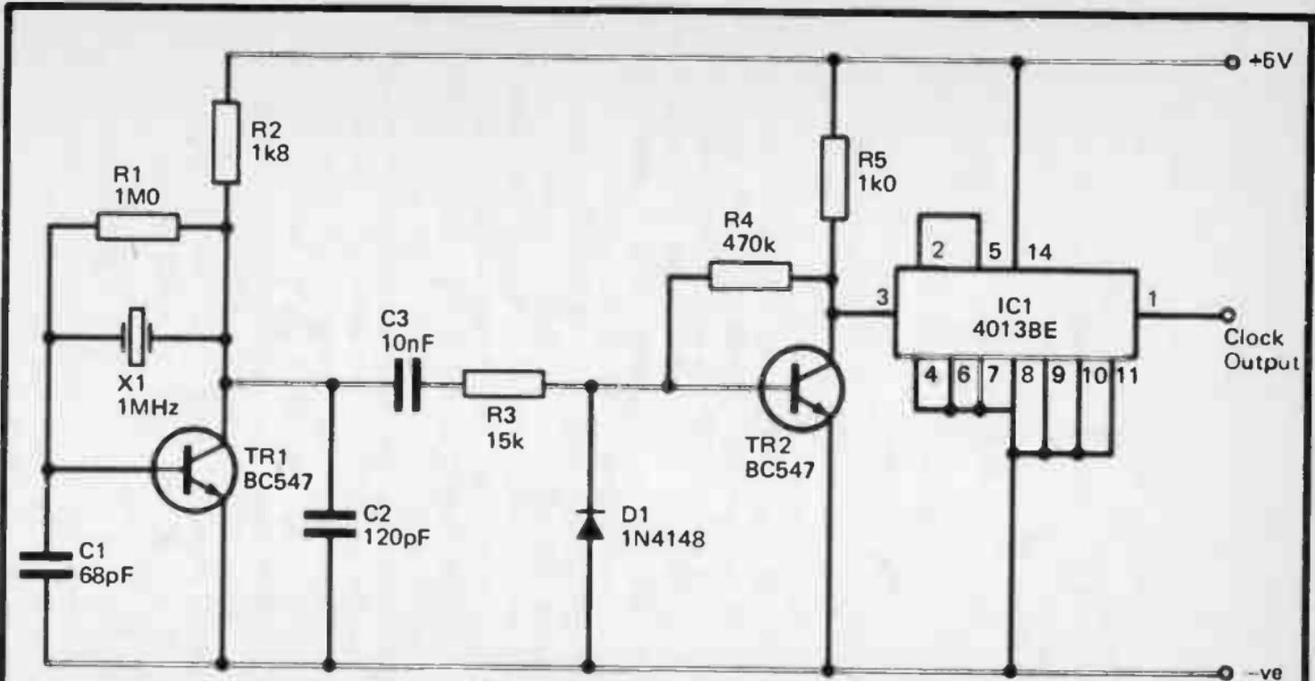
Fig 6. An alternative clock generator using a 1MHz crystal
