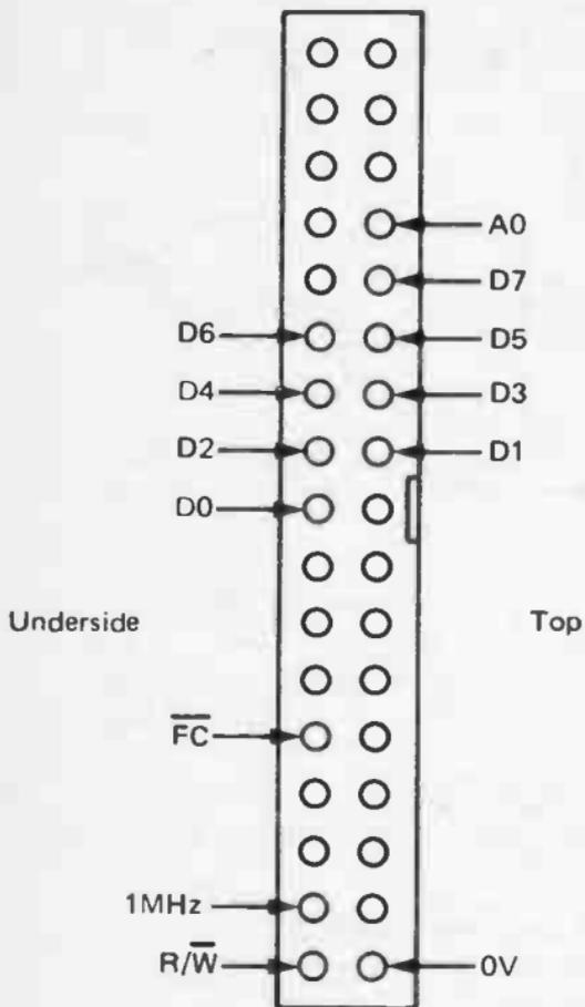
*Fig 15. The connections to the 1MHz Bus
