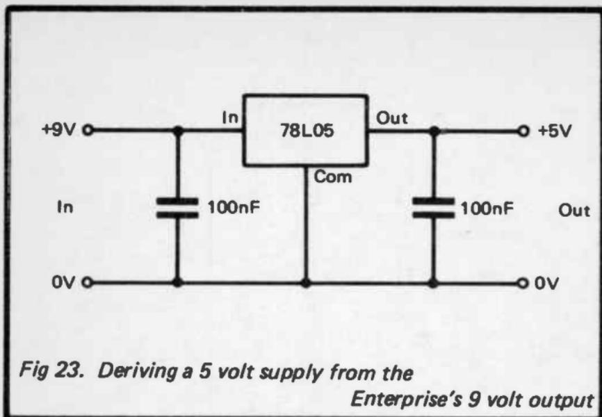
*Fig 23. Deriving a 5 volt supply from the Enterprise's 9 volt output*
