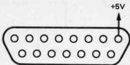
*Fig 13. A +5 volt supply can be taken from the BBC computer's analogue port*
