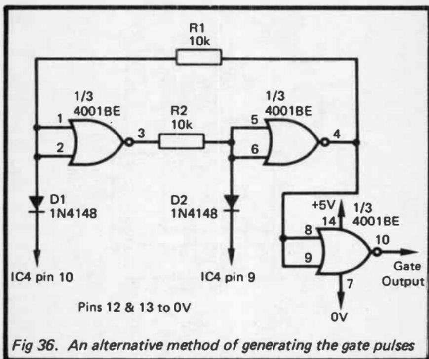
Fig 36. An alternative method of generating the gate pulses
