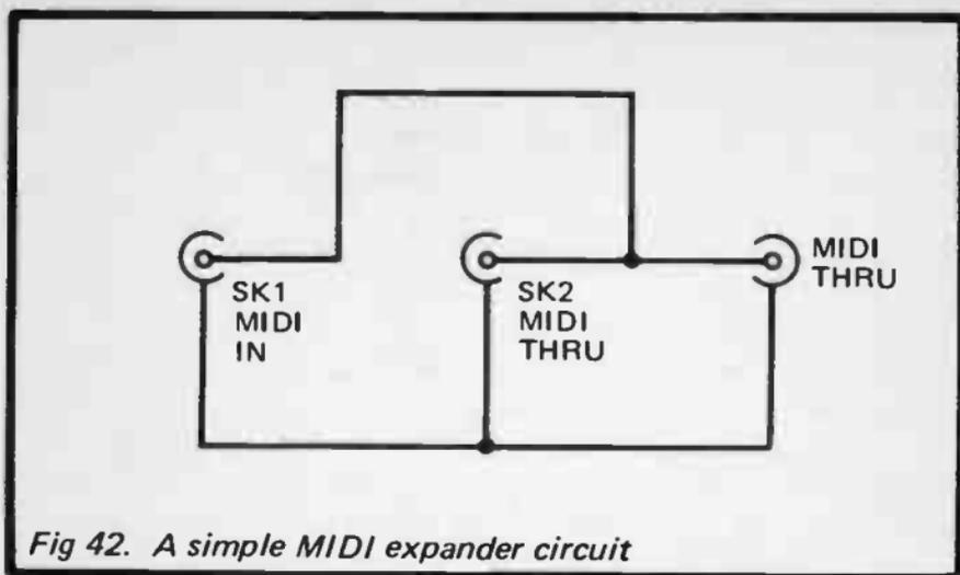
Fig 42. A simple MIDI expander circuit
