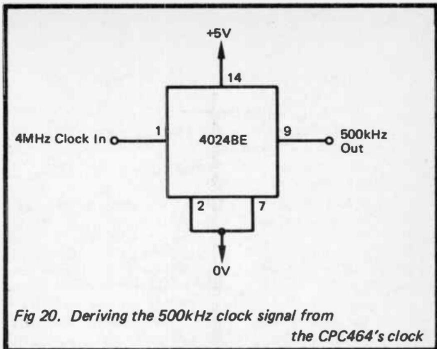
*Fig 20. Deriving the 500kHz clock signal from the CPC464's clock*
