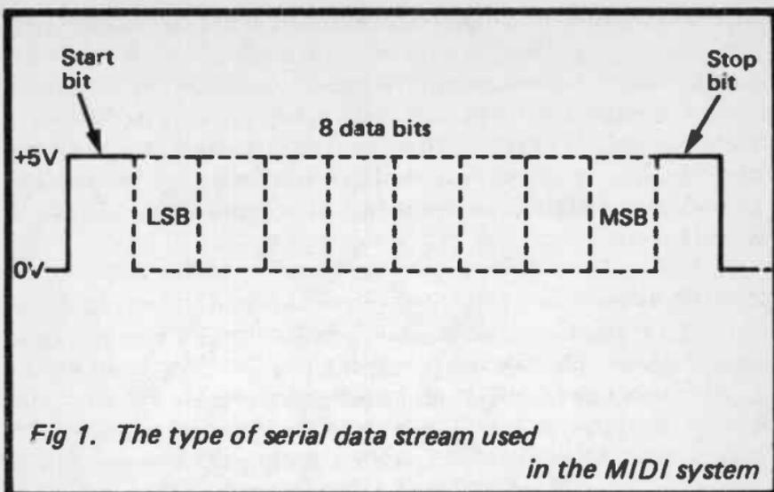
*Fig 1. The type of serial data stream used in the MIDI system*
