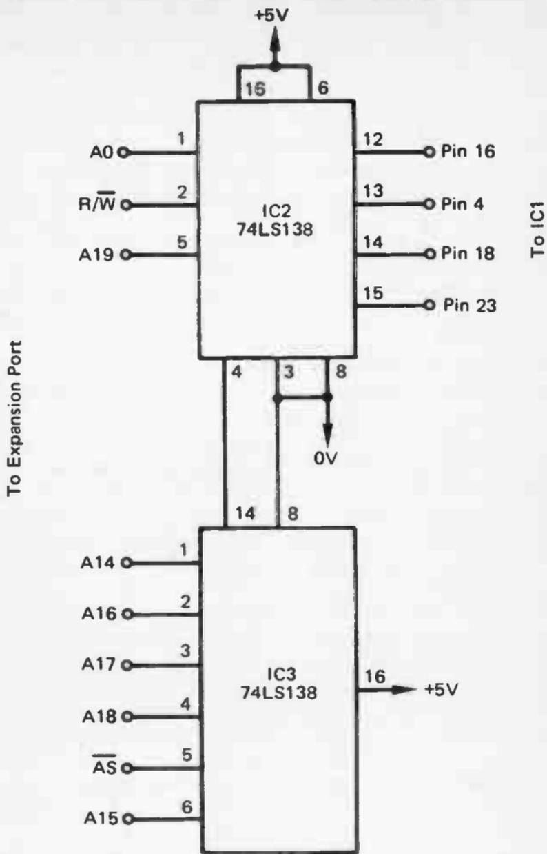
Fig 31. The address decoder for operation with the QL computer
