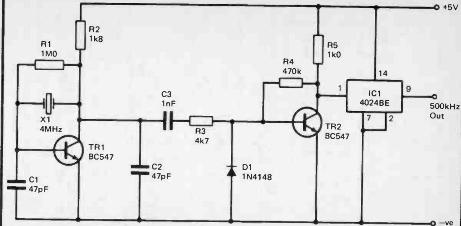
Fig 5. A 500kHz clock circuit using a 4MHz oscillator
