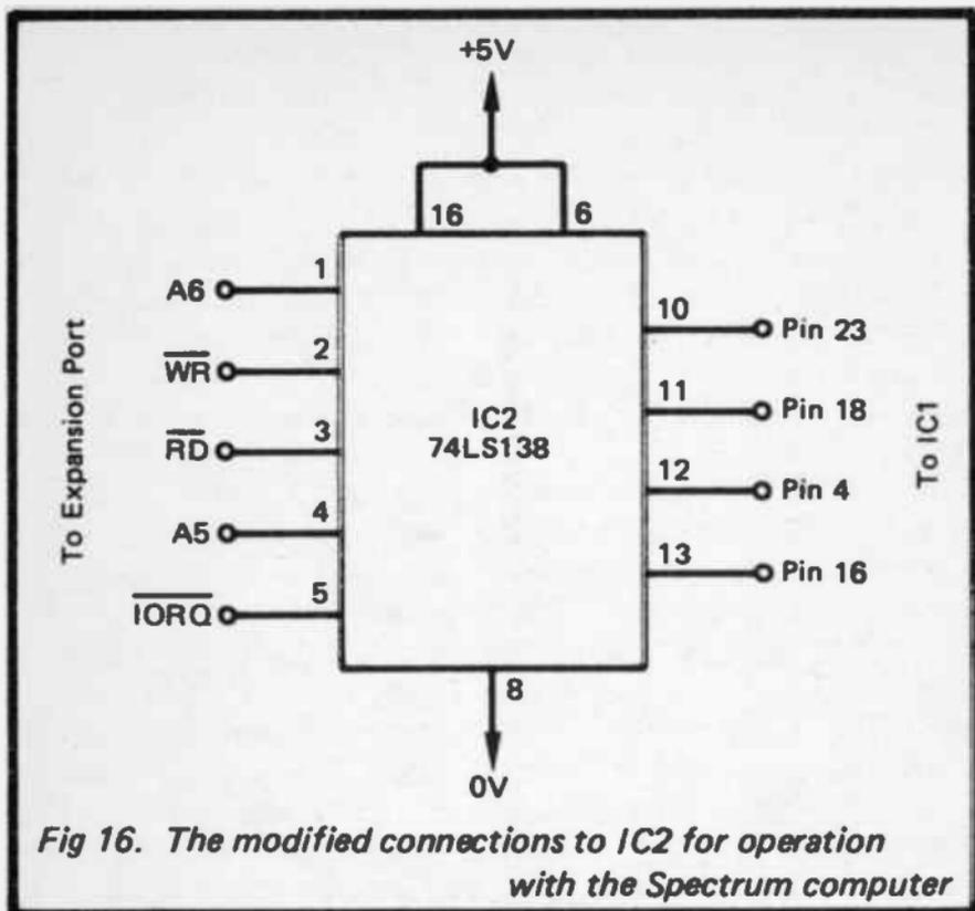
write lines are decoded by the three address inputs of IC2. As only two addresses are required it is not necessary to decode A7 as well.
