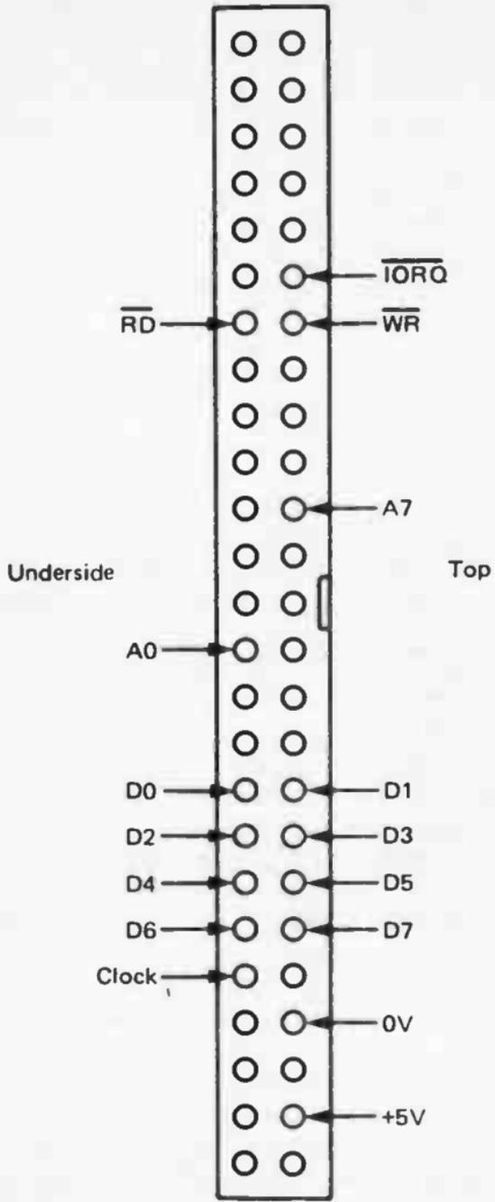
Fig 25. Connection details for the MSX expansion port
