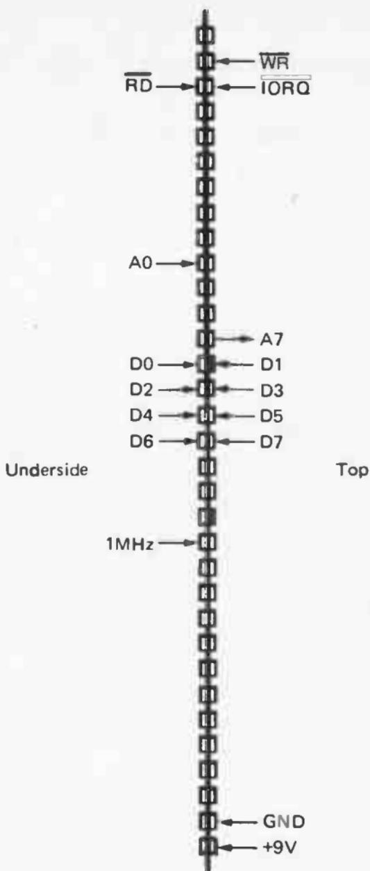
Fig 24. The connections to the Enterprise expansion port
