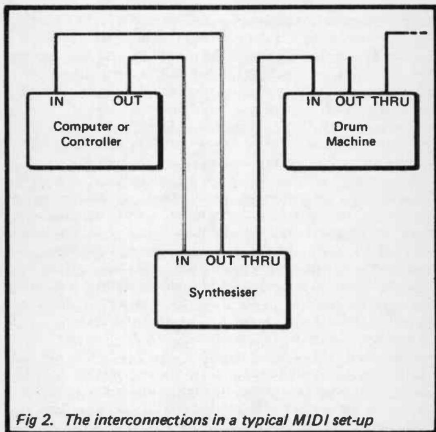
*Fig 2. The interconnections in a typical MIDI set-up*
