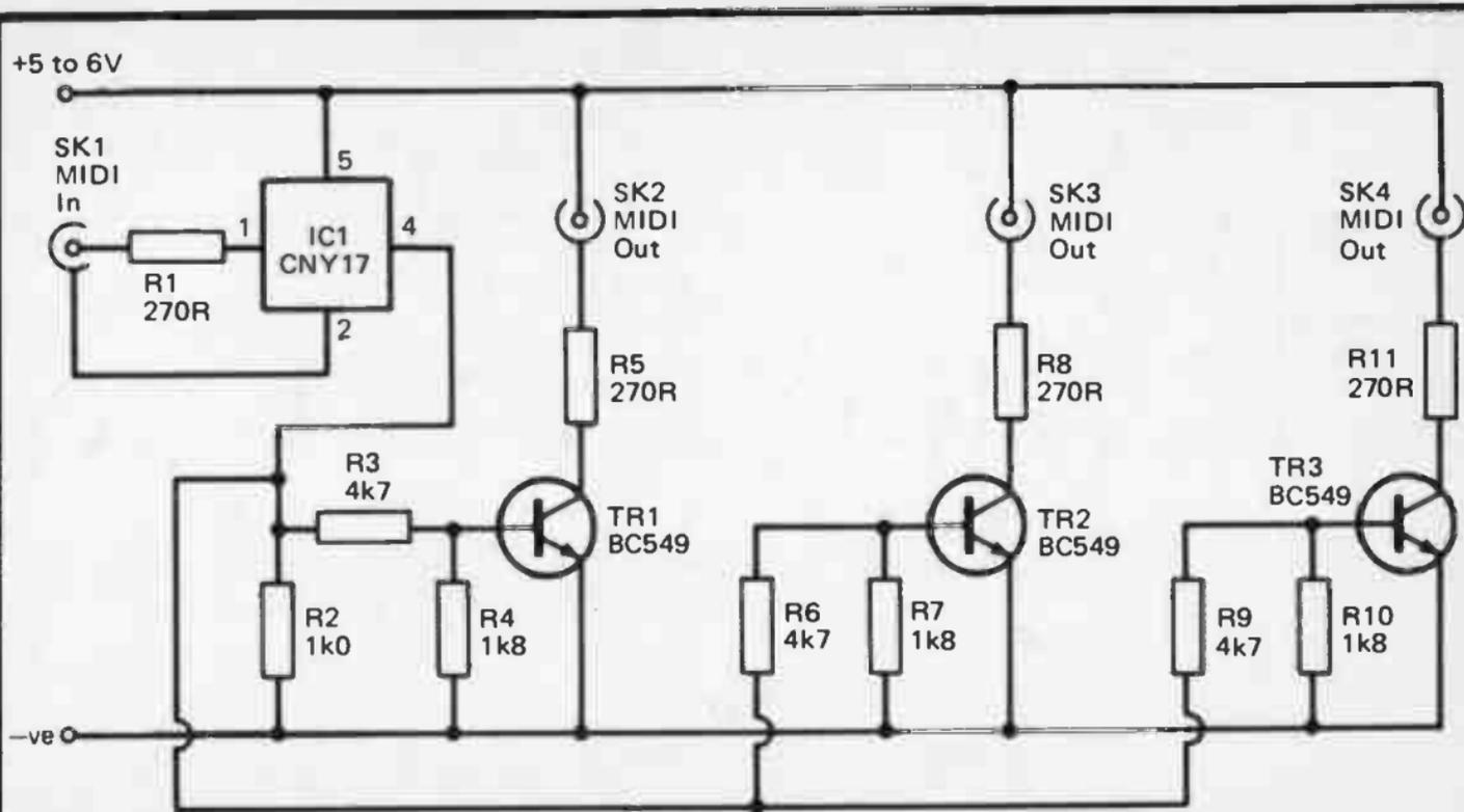
Fig 43. An active MIDI expander circuit
