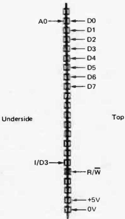
Fig 10. Connection details for the VIC-20 cartridge port
