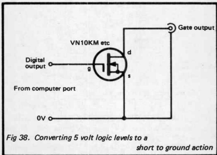
Fig 38. Converting 5 volt logic levels to a
