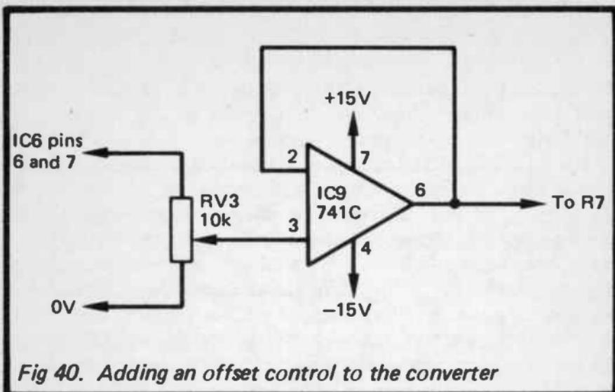
*Fig 40. Adding an offset control to the converter*
