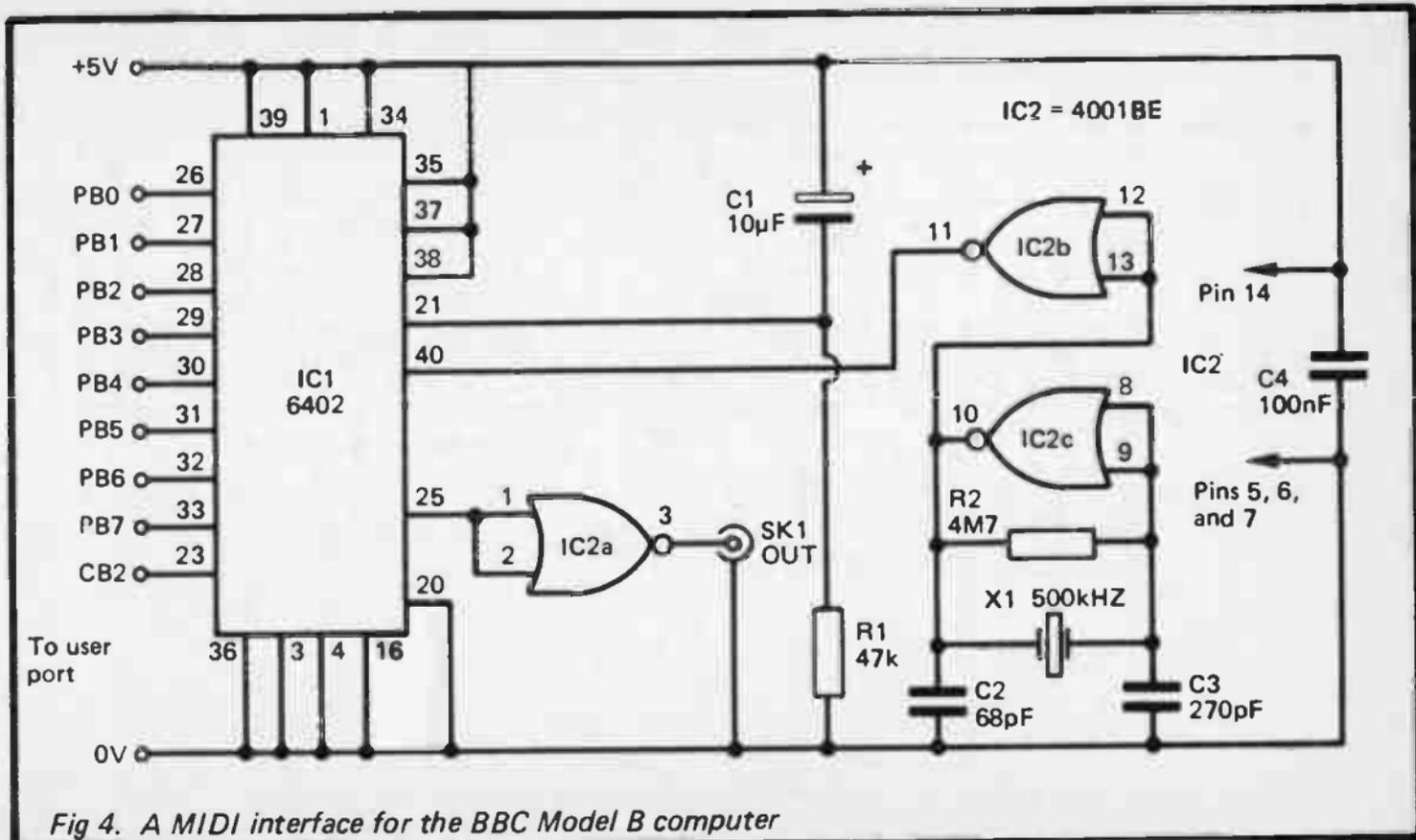
Fig 4. A MIDI interface for the BBC Model B computer
