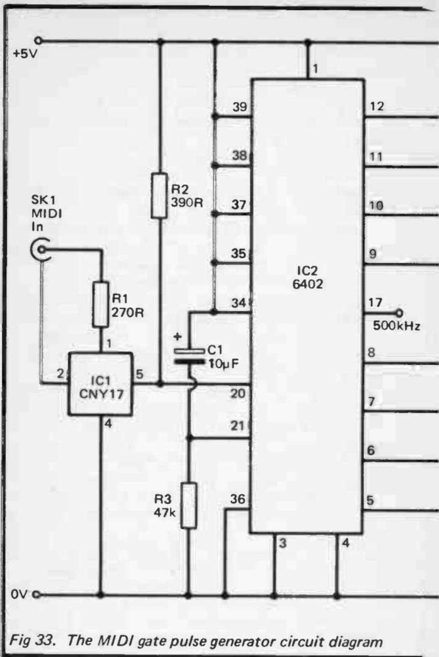
Fig 33. The MIDI gate pulse generator circuit diagram
