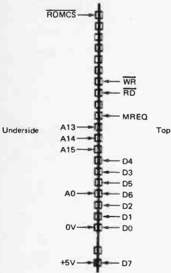
Fig 30. The connections to the ZX81 expansion port
