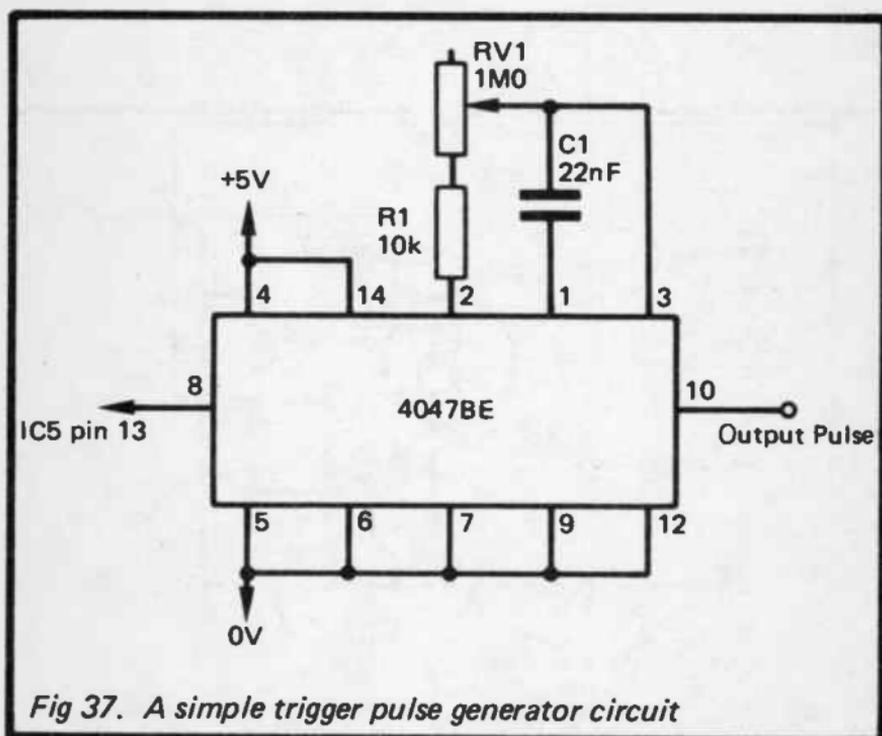
Fig 37. A simple trigger pulse generator circuit
