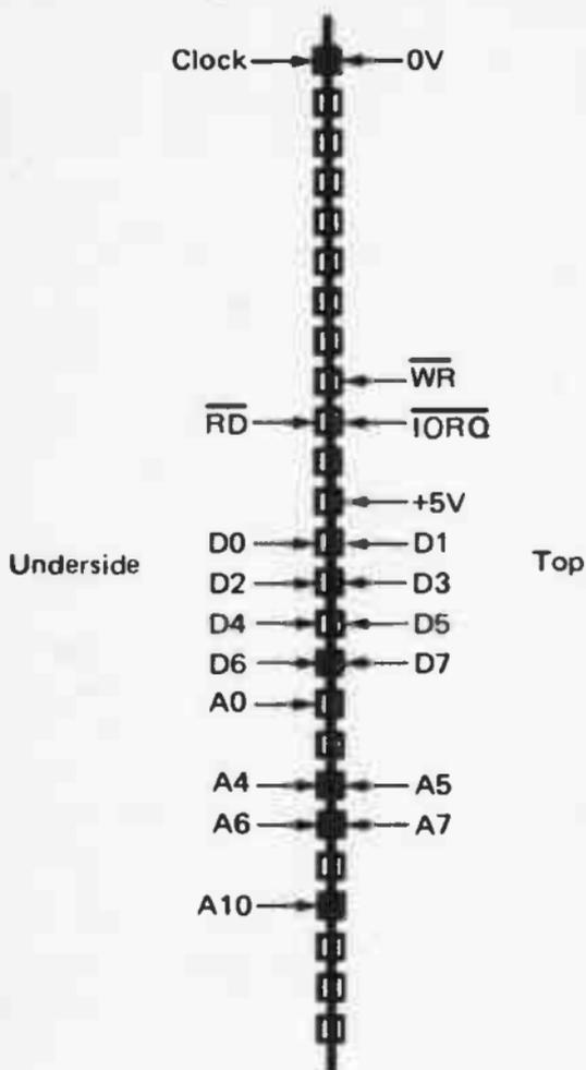
Fig 19. The connections to the CPC464's
