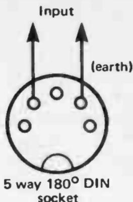
*Fig 7. The connections to the MIDI input socket*
