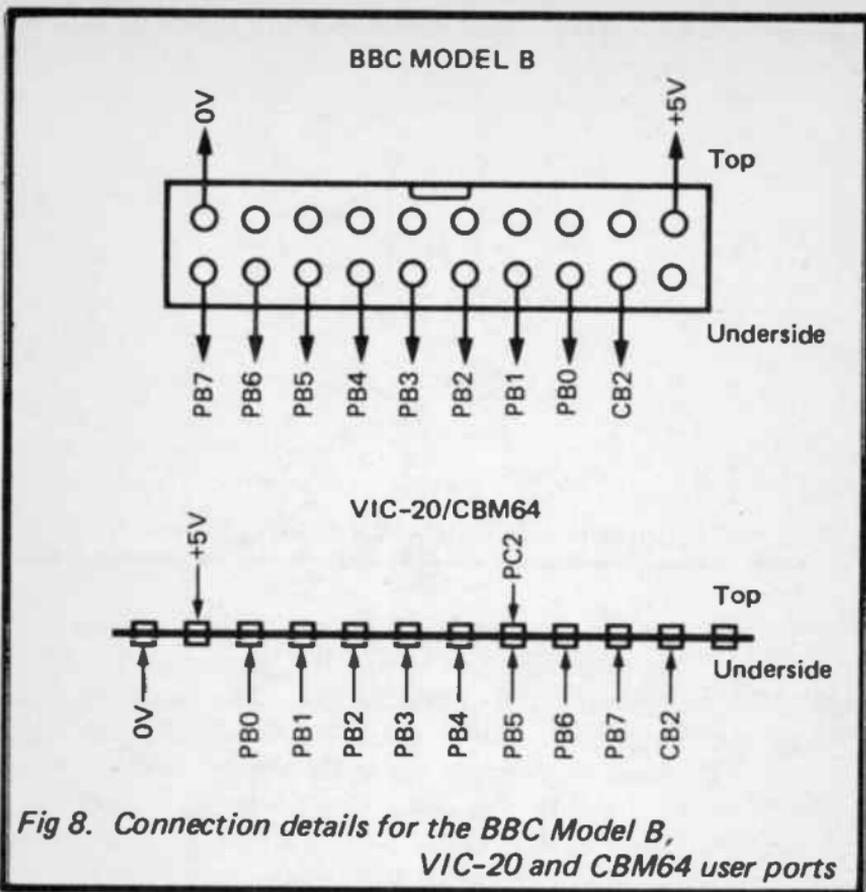
Fig 8. Connection details for the BBC Model B, VIC-20 and CBM64 user ports
