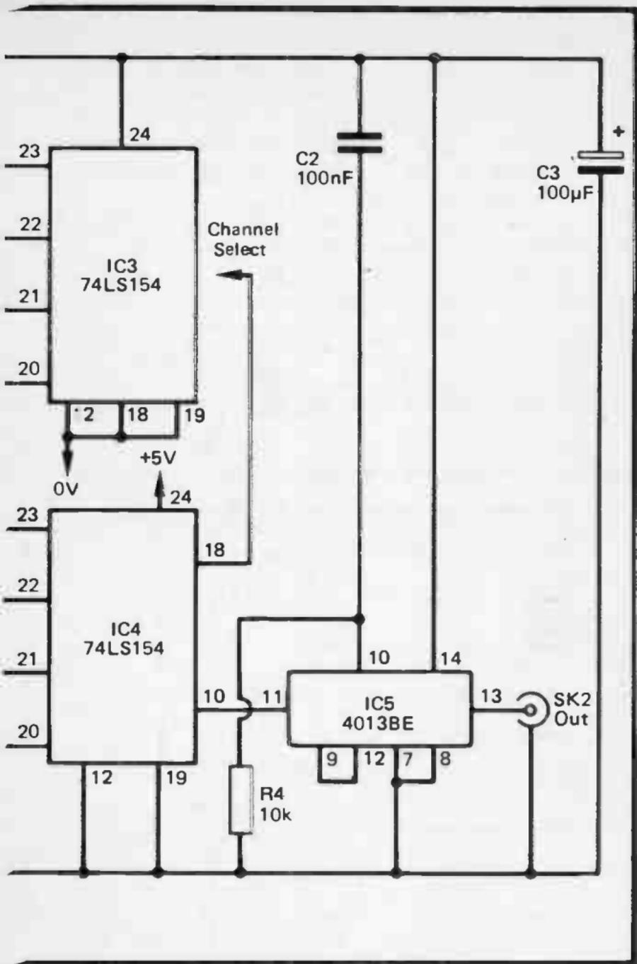
are less than obvious, transmit the same header code when a note is released as when a note is commenced (1001). My SCI Six-Tracks falls into this category, and the circuit has therefore been designed to only respond to the 1001 header code and to ignore
