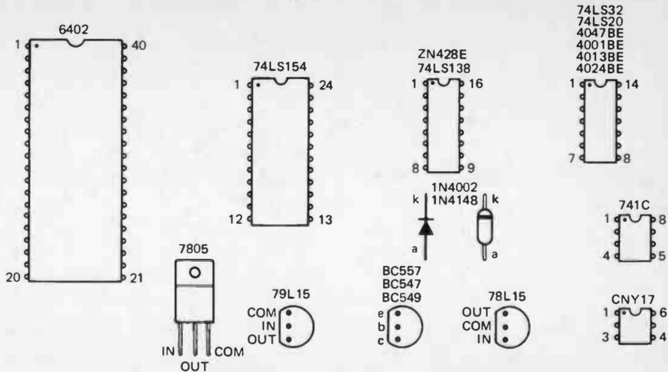
Fig 44. Semiconductor pinout details (transistor base views, IC top views)
