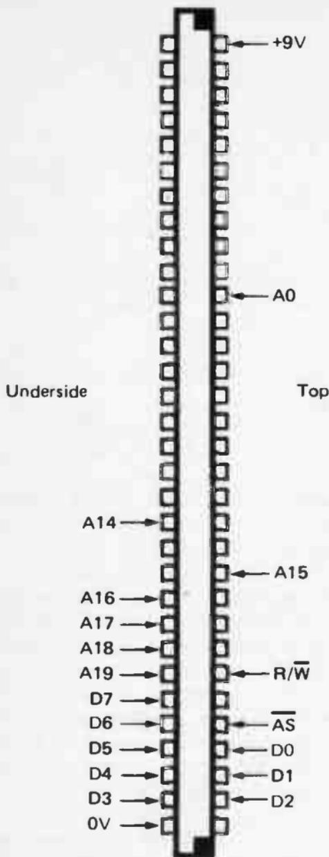
Fig 32. The connections to the QL's expansion port
