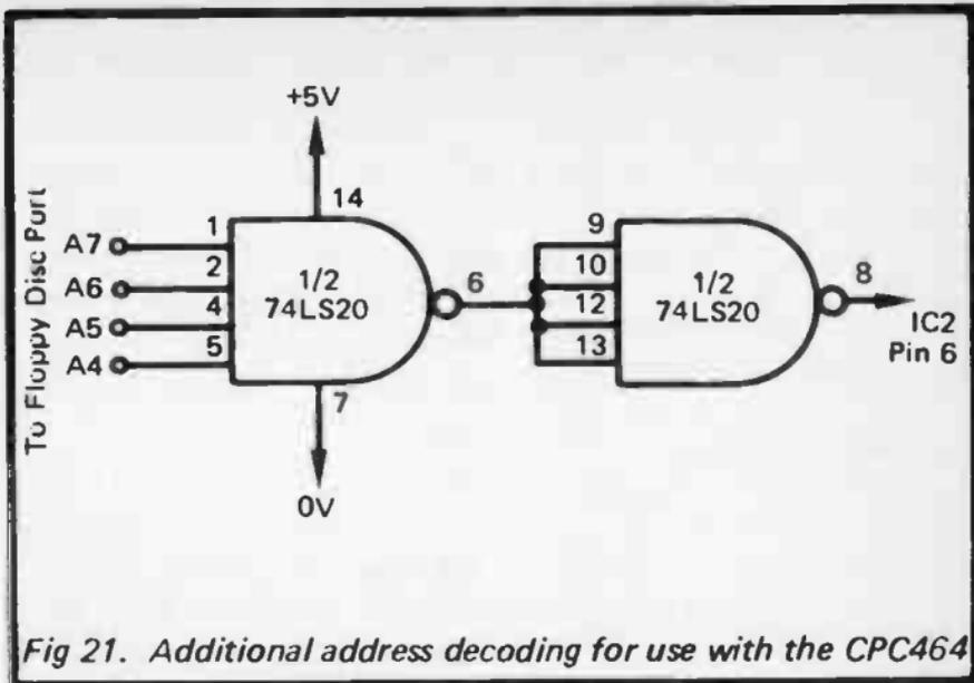
Fig 21. Additional address decoding for use with the CPC464
