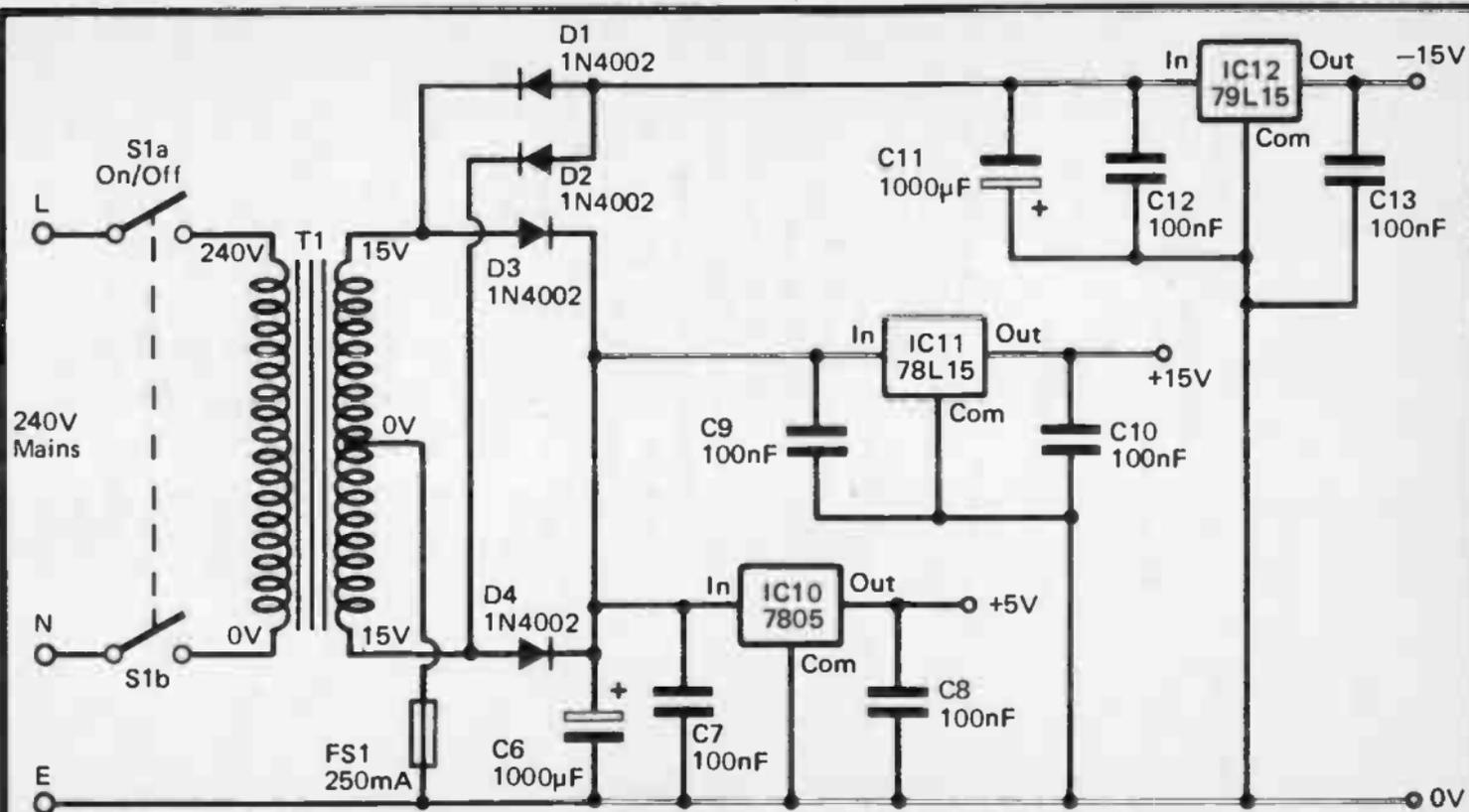
Fig 41. The circuit diagram of the mains power supply unit
