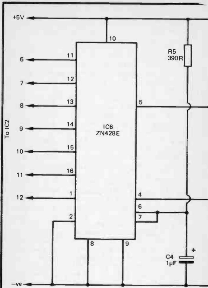
Fig 39. The MIDI to CV converter circuit diagram
