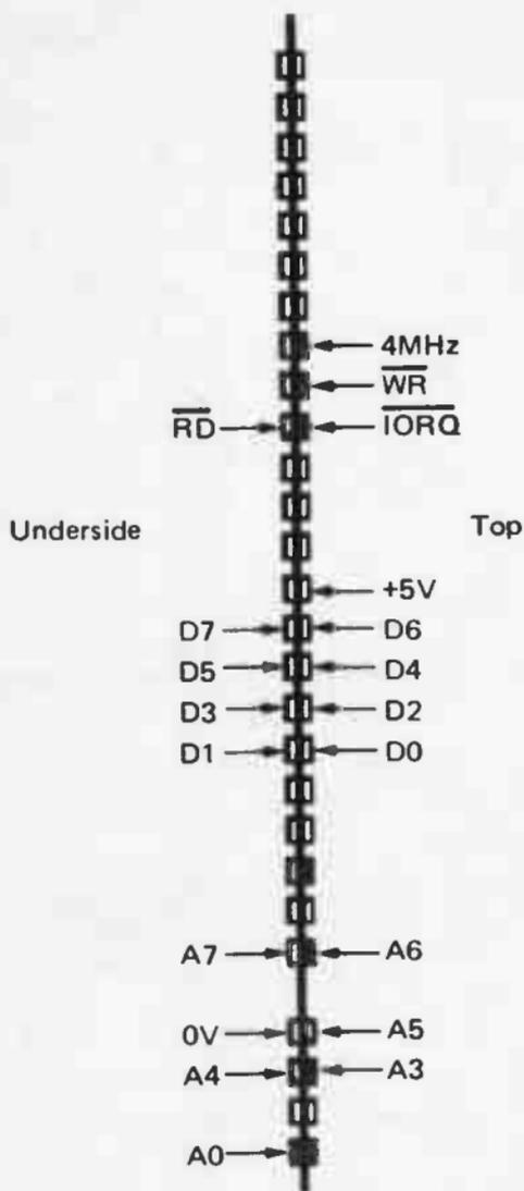
Fig 27. The connections to the MTX expansion port
