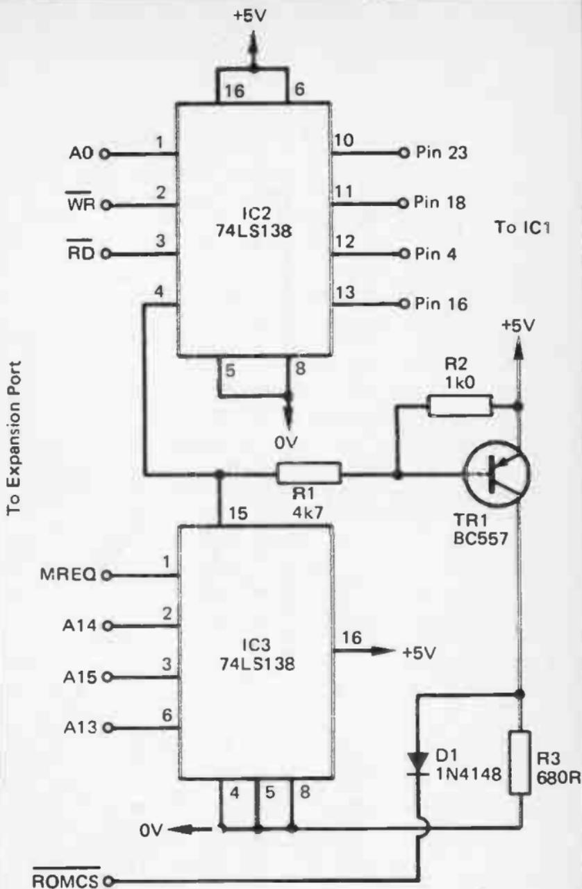
Fig 29. The address decoder for the ZX81
