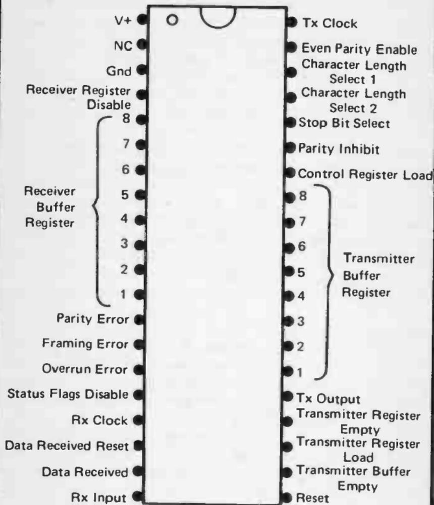
Fig 3. Pinout details for the 6402 UART
