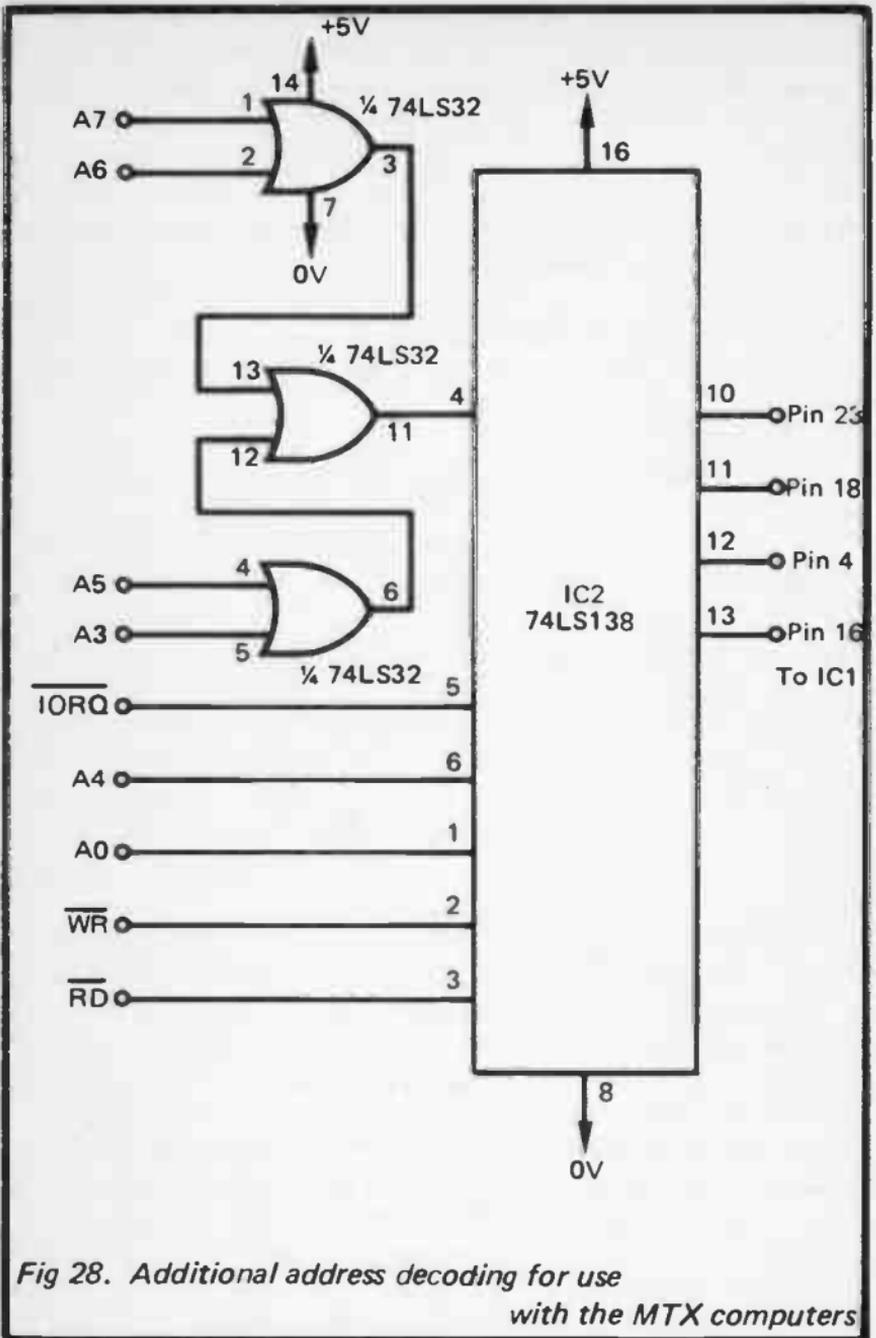
Fig 28. Additional address decoding for use with the MTX computers
