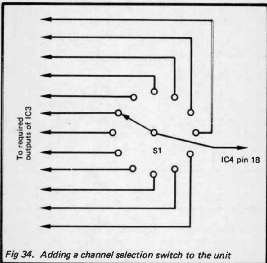
Fig 34. Adding a channel selection switch to the unit
