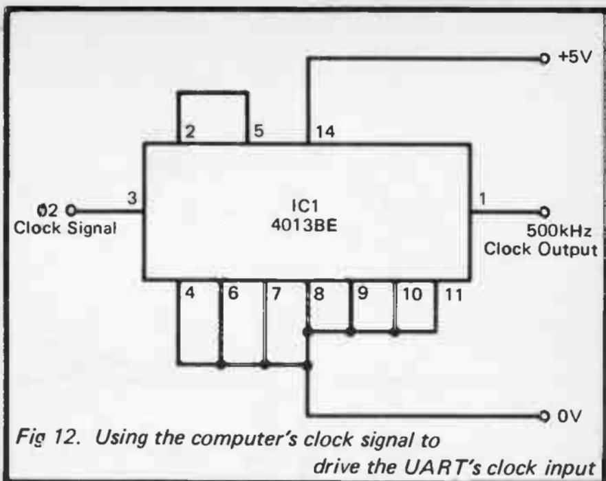
*Fig 12. Using the computer's clock signal to drive the UART's clock input*
