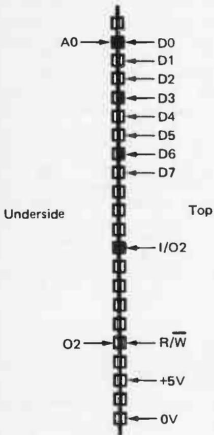
Fig 11. Connection details for the CBM64 cartridge port
