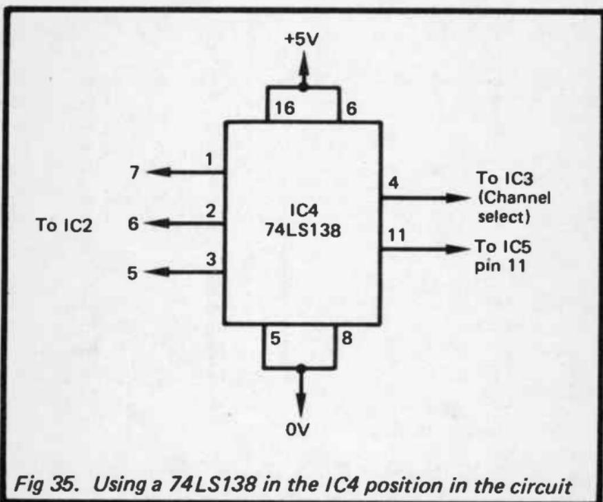
Fig 35. Using a 74LS138 in the IC4 position in the circuit
