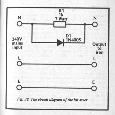
Unfortunately, this gives an excessive reduction in power, and D1 is therefore bypassed to some extent by R1 on half cycles where D1 is reverse biased. This results in the iron being run at roughly 80% of full power, which in practice seems to be sufficient to increase bit life, but not so much as to make soldering impossible or difficult. The value of R1 shown in Fig.38 is for a 15 watt iron, and it should be reduced to 680 ohms for a 25 watt iron.
