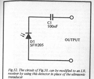
red photo-diode that has a built-in infra-red filter, and does not require a separate filter. When subjected to the pulsed infra-red beam D1 produces a small voltage pulse in response to each pulse of infra-red light, and these are coupled to the input of the receiver circuit by D.C. blocking capacitor C1.
