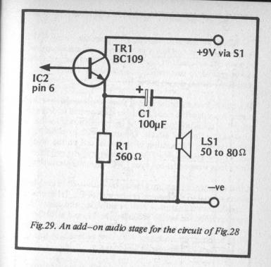
Only a modest output power of milliwatts rather than watts is provided by this output stage, but this is adequate in this application where high volume would not normally be desirable. It may be found that higher volume can be attained by slightly increasing the value of R9 in the main receiver circuit, but this should not be overdone or severe distortion will result
