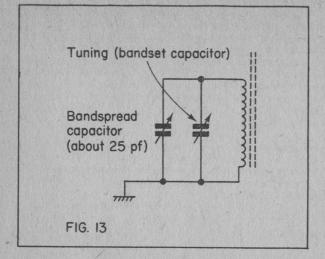
Electrical bandspread is an electrical equivalent of a mechanical reduction drive, and simply consists of adding a low value variable capacitor in parallel with the main tuning capacitor. This is shown in the circuit of Fig.13. The value of the additional capacitor is not critical, and can be anything from about 15 to 50 pF.
