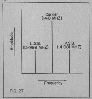
It will be helpful to first consider what exactly an A.M. signal consists of. For the sake of this example we will consider a 14MHZ carrier wave which is modulated by a 1kHZ audio tone. Looking at this in terms of the frequencies that are produced at the output of the transmitter we have the arrangement shown in Fig.27.
