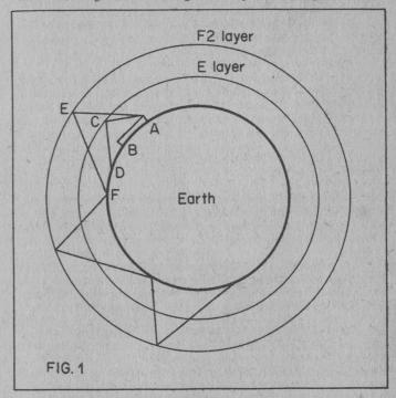
When the transmitter is close to the receiving station the radio waves can travel direct from the transmitter to the receiver. This is represented by line A-B in the diagram, and is termed the 'ground wave'.
