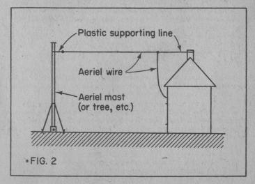
Ideally the aerial should be some 20 to 40 Metres long overall (i.e. including the lead in wire), but as little as 10 Metres will suffice quite well. Generally speaking the longer the aerial the greater the signal it will provide. Thus when conditions are somewhat mediocre a long aerial will provide a usable signal where a fairly short aerial will not.
