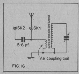
When this occurs it is necessary to reduce the strength of the aerial signal, and this can be accomplished using the simple attenuator circuit shown in Fig.16. SK1 is the normal aerial socket, and when overloading occurs the aerial is connected to SK2 instead. This introduces a low value fixed capacitor into circuit between the aerial and the input coupling coil of the receiver. Losses in the capacitor reduce the signal
