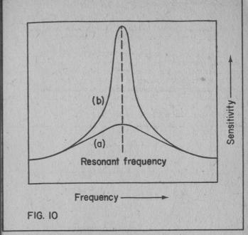
it would look something like the graph shown in Fig. 10(a). The peak occurs at the resonant frequency of the tuned circuit, and the response only falls away gradually either side of this. As a result, the receiver has only a very limited degree of selectivity, and when a transmission is present within a few tens of KHZ of the desired one, both signals will fall within the receiver's passband, and it will not be possible to tune to only one or other of them.
