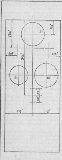
FIG.7. CONTROL & COIL DRILLING CENTRES
