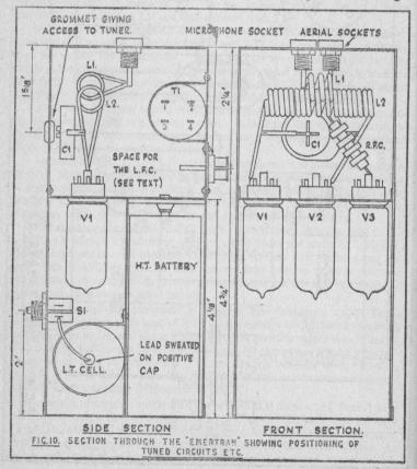
length of L600 solid co-ax cable terminating in a Belling-Lee L604/P plug. As neither side of the case carries any components, either or both may be made removable.
