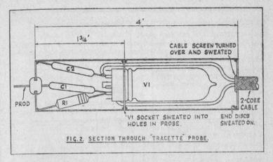
The back cover disc of the probe is drilled centrally to run over the screened cable, slipped up to the probe housing and the screening of the cable is unravelled for a \( \frac{1}{4}\)" or so and sweated down on to the interior face of the back disc, thus providing both a firm cable anchorage and the earth return between the probe and the main amplifier.
