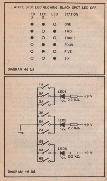
SWITCH 1 a, b, c is for station 1 SWITCH 2 a, b, c is for station 2 etc.
