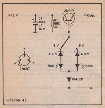
such as a 2N3055 should be substituted. The voltages supplied are 6.2v (1.5v + 4.7v) and 9v (2.2v + 6.8v) the LEDs indicate which voltage the regulator is switched to, red 6.2 volts, green 9 volts. The switch used can be a SPDT slide type.
