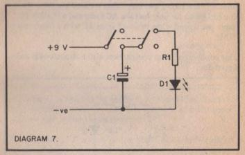
The electrolytic capacitor charges up again when the circuit is switched back. The value of the resistor R1 controls the length the LED glow persists, a lower value can be used, this will give a brighter glow for a shorter time. If a higher value of R1 is used this produces a dimmer glow which persists longer.
