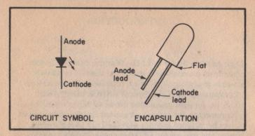
If the connection details of a LED are not known adopt the following procedure. Connect the LED WITH A  $1K\Omega$ **RESISTER IN SERIES** to a 9 volt battery, if the LED does not glow reverse connections. With the LED glowing the lead connected to the negative pole of the battery is the cathode.
