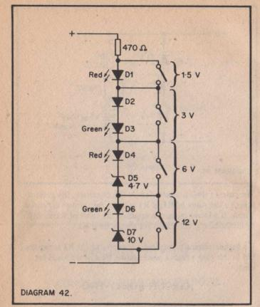
For each position the voltage control value is double the previous section. The first "element" is a red LED which gives a voltage drop of 1½ volts, the next element is a green LED ) and a silicon rectifier in series which gives a total voltage drop of nearly 3 volts (2.2 volts + 0.75 volts) as the forward voltage drops across a green LED is about 2.2 volts.
