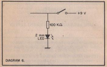
Although the gleam from a LED at such a very low current is not very bright the transition from nonillumination to illumination when switched on is easily noticed and this is a very useful indication of switching a function e.g. to 'record' on a battery tape recorder.
