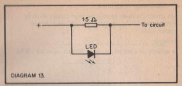
The voltage drop across a red LED is about 1½ volts, i.e. there must be a voltage of about 1½ volts across a LED for it to glow. A red LED is connected in parallel with a  $1.5\Omega$  3 watt wirewound resistor. The voltage drop across the resistor increases with increasing current, when the voltage drop exceeds 1.5 volts the LED will glow.
