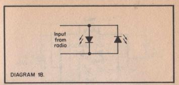
For the best results the LEDs display should be viewed in a darkened room, the effect is of gently pulsating light. The 2 LEDs can be mounted in front of 2 sheets of aluminium fixed together at right angles, this arrangement gives multiple images of the LEDs.
