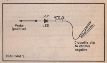
If the tester is required for use with a positive chassis car the LED should be wired the other way round so that the anode is connected to the chassis (positive).
