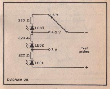
This is a simple inexpensive GOOD/NO GOOD tester for 3v, 4½v or 6v batteries. The switch sets the tester to the various voltages. A 3 volt battery will make LED 1 glow, a 4½ volt battery will make LED 1 and LED 2 glow, a 6 volt battery will make LED1, LED 2 and LED 3 glow.
