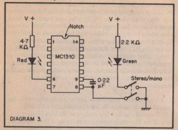
In the diagram the components in the rest of the decoder circuit are omitted for clarity. The stereo defeat switch is a DPST type. One of the miniature DPDT slide switches can be used, in this case the extra set of contacts are not connected.
