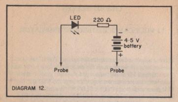
One caution is that the users fingers should not be touching the probes if the skin is slightly moist firm contact with the probes will make the LED glow dimly due to a small current flowing via the skin.
