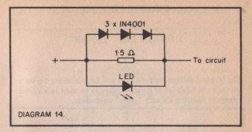
2.2 volts. If 3 such rectifiers are connected across a LED, when the voltage exceeds 2.2 volts the rectifiers conduct and, due to their much smaller forward resistance, short out the LED and extinguish it. This means that when the current through the resistor produces a voltage drop in excess of 2.2 volts the LED is extinguished.
