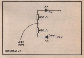
When the probe is connected to the 5 volt supply both red and green LEDs will glow. When the logic probe touches a circuit connection, if the GREEN LED glows brightly this indicates logic level 0, if the RED LED glows brightly this indicates logic level 1.
