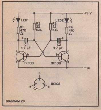
The values indicated in the circuit diagram give a rapid on/off display, if the value of C1 and C2 is increased this will give a lower frequency and hence slower flashing rate.
