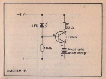
The current flow is controlled by the transistor, the current is set by the value of R1, if R1 is  $22\Omega$ , the current is fixed at 50mA. If a lower current is required the value of R1 should be increased e.g. for 25mA R1 should be  $39\Omega$ .
