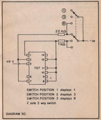
The 707 display can with the use of switching display several numbers in turn. The switching is simplified if the numbers have common segments. For example a circuit to display 8 or 9 is very simple the difference is segment E, only this needs to be switched ON and OFF to change the number. If segments ABCDFG are continuously on and E off 9 is displayed, if E is on an 8 is displayed. Other examples are 5 and 6 this pair of numbers differ in one segment only.
