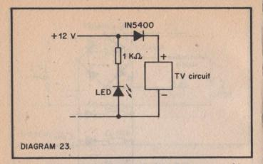
The 1N5400 silicon rectifier specified is a 3 amp type and is suitable for any portable television. The red LED can be fitted into the portable TV case next to the 12 volt battery connector.
