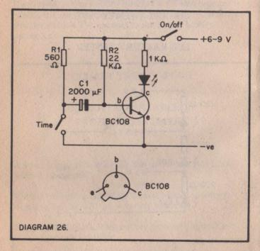
This is a simple electronic timer, when the TIME button is pressed the red LED is extinguished, about 30 seconds later the LED glows again to indicate time elapsed. The time period depends on the value of C1, increasing the value of C1 extends the time period. The circuit can be powered by 6 to 9 volts.
