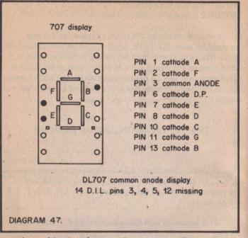
certain combinations form numbers. A more effective display is possible if two 707 displays and eight multivibrators using four 7400 ICs are connected together.
