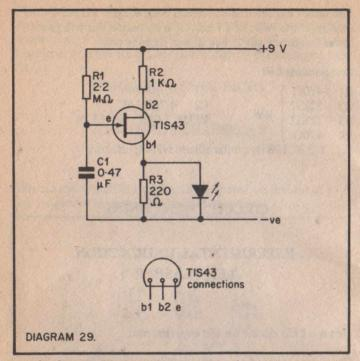
can be decreased by reducing the value of C1 e.g. to  $0.22\mu$ F or increased by using a higher value e.g.  $1\mu$ F or  $2.2\mu$ F.
