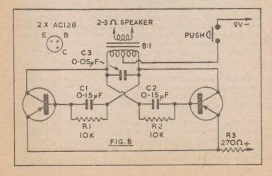
The primary of the transformer provides the collector load, and each transistor drives the base circuit of the other, via the capacitors and parallel resistors C1/R1 and C2/R2.
