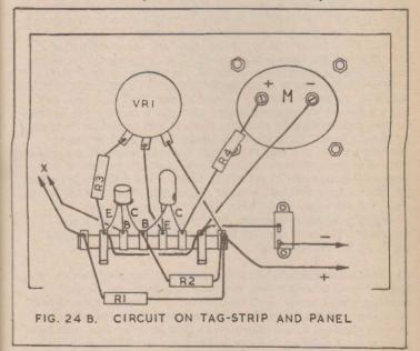
Insulated leads pass from terminals or sockets X to the electrodes. These can be small squares of copper foil (or other similar metals) taped to the subject's palm. A conductive jelly ought to be used here to obtain the best electrical contact between subject and electrodes, but will probably have to be omitted. VR1 should be set so that touching or moving the electrodes causes a large meter deflection.
