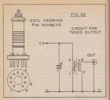
The use of the coils as plug-in units is also shown, and this method avoids switching, and simplifies band-changing. The coil cans provided by the manufacturer can be used as screens, where the layout makes this necessary to avoid instability or whistles due to the RF amplifier oscillating.
