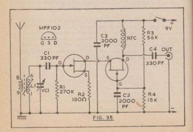
The circuit in Fig. 35 uses two FETs in cascade, and this arrangement is normally stable, with a reasonable layout. Tuning of L1 is by VC1, and signals are applied to the gate of the first FET. The drain of this device goes to the source of the second FET, resulting in good isolation of input and output circuits. The second FET gate is effectively grounded by C2. Signals are developed across the RF choke, and taken to the receiver by C4.
