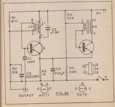
The OC72 functions as audio oscillator, the windings of the audio transformer being phased to achieve this. Common emitter coupling of the oscillators provides amplitude and frequency modulation of the RF signal.
