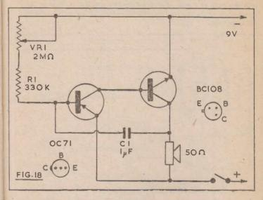
The few components can be assembled on a small tag strip. Place VR1 and the on-off switch on the case front. If a separate switch is fitted, this has the advantage that VR1 can be left at any wanted setting. A nicely varnished wooden case is probably best, as it also provides a soundbox effect, to increase volume. The bottom should be covered with felt or otherwise arranged to prevent scratching furniture or a piano top.
