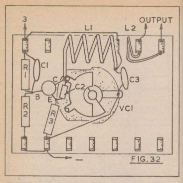
The BC200 shield lead is not connected. Miniature ceramic disc capacitors are probably most suitable. When the board is wired, it can be mounted by the bush of VC1. Extra washers are necessary between the tagboard and panel, so that the tags clear the metal.
