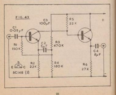
The 2-transistor buffer in Fig. 43 can help overcome such difficulties. It has a high impedance input, but a low impedance output. Its gain is 1 - that is, output is approximately the same as input, despite the impedance transformation.
