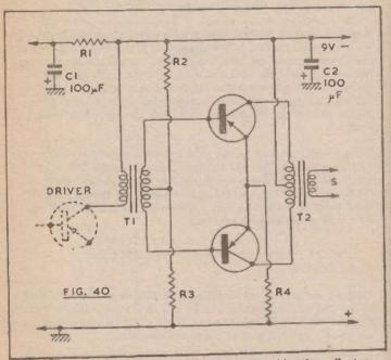
T1 is the driver transformer, and its primary provides the collector load for the previous audio amplifier. The centre-tapped secondary drives the output transistors in push-pull, one conducting when the other is cut off. Base operating conditions are set by R2 and R3. R4 is an emitter resistor, to limit emitter current.
