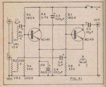
Input (1) is for relatively low impedance sources, and VR1 is the individual level control for this. Input (2) is more suitable for high impedances, and has the gain control VR2.
