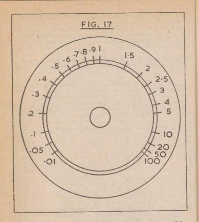
Values on this scale are multipliers. Thus the actual markings will be read directly for a range in which 1uF is the central scale marking. This range results from fitting a 1uF capacitor at C4, in Fig. 16. The unknown capacitor is placed at CX. Values may then be read from 0.01uF up to 100uF by turning the control knob of VR1 until the null is obtained, and reading from the scale.
