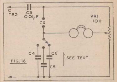
Fig. 16 is the practical bridge, receiving input from a multivibrator, one collector being connected to the coupling capacitor C3. A fairly strong, high tone is most suitable, as it will be best heard with low value capacitors. A suitable audio oscillator can employ the multivibrator circuit first shown, with 10k collector resistors, 100k base resistors, 0.01uF coupling capacitors, and a pair of OC71 transistors. Other circuits to supply a tone could of course be used.
