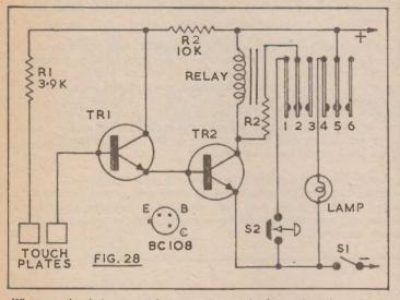
When no circuit is present between the touch plates, there is no base current for TR1, so emitter and collector current here is negligible. TR2 is also cut off, and so collector current through the relay winding is virtually zero.
