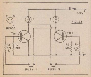
Both the push switches are normally open. In these circumstances each transistor base is held negative by resistors R2 and R3, and collector currents are negligible. Both indicator lamps A and B are thus extinguished.
