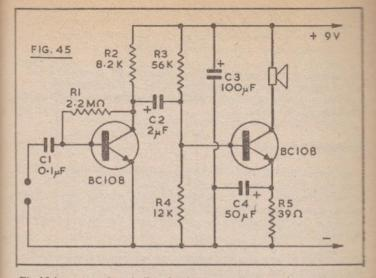
Fig.45 is a somewhat similar circuit, except that emitter bias for the output stage is provided by R5, and the speaker is placed in the collector circuit. A 15 ohm speaker is again suggested, though impedances up to about 75 ohms can be used. Current drain is about 15-20mA, with a little more gain, but distortion from overloading can arise more quickly if the input is too great.
