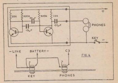
Fig. 6 is the complete circuit. For convenience, the multivibrator and battery are fitted in a box carrying two jack sockets. These are wired as shown, to take plugs for the key and phones. The type of high or medium impedance headset used for SW listening will do very well, but any phones can be employed, including crystal earpieces. An on-off switch is not necessary as current is only drawn when the key is down.
