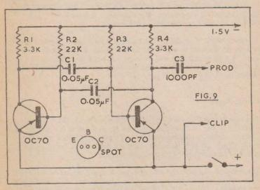
The resistors may of course be small, fractional-watt components, and C1 and C2 may be low-voltage capacitors. If only low-voltage transistor equipment will be tested, C3 may also be of low voltage (say 15V). But if valve equipment, or equipment having higher potentials will be tested, C3 must be chosen to suit, and be of adequate voltage rating. A 500V capacitor will usually be suitable for all but high-power circuits such as large amplifiers and modulators.
