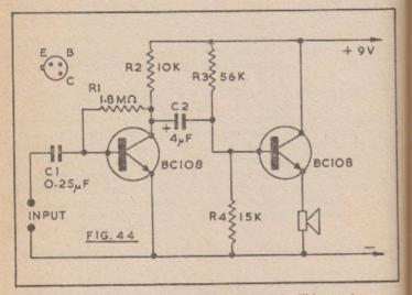
Base bias in the output stage is from R3 and R4. This transistor operates as a grounded collector amplifier – the collector is not actually connected to the "earth" or ground line, but is grounded as regards audio signals through the battery, which has negligible impedance.
