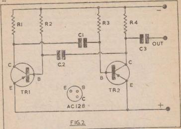
If a battery is connected in the wrong polarity to a circuit such as that in Fig. 1 or Fig. 2, no damage may arise if transistor currents are limited to safe values by the resistors R1 to R4. But in many cases this will not be so, and then immediate destruction of the transistors is likely.
