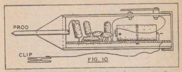
A flexible lead fitted with a clip forms the earth return connection. Test the oscillator before fitting it in the tube, either by touching the prod on an audio circuit, or by connecting headphones from prod to clip.
