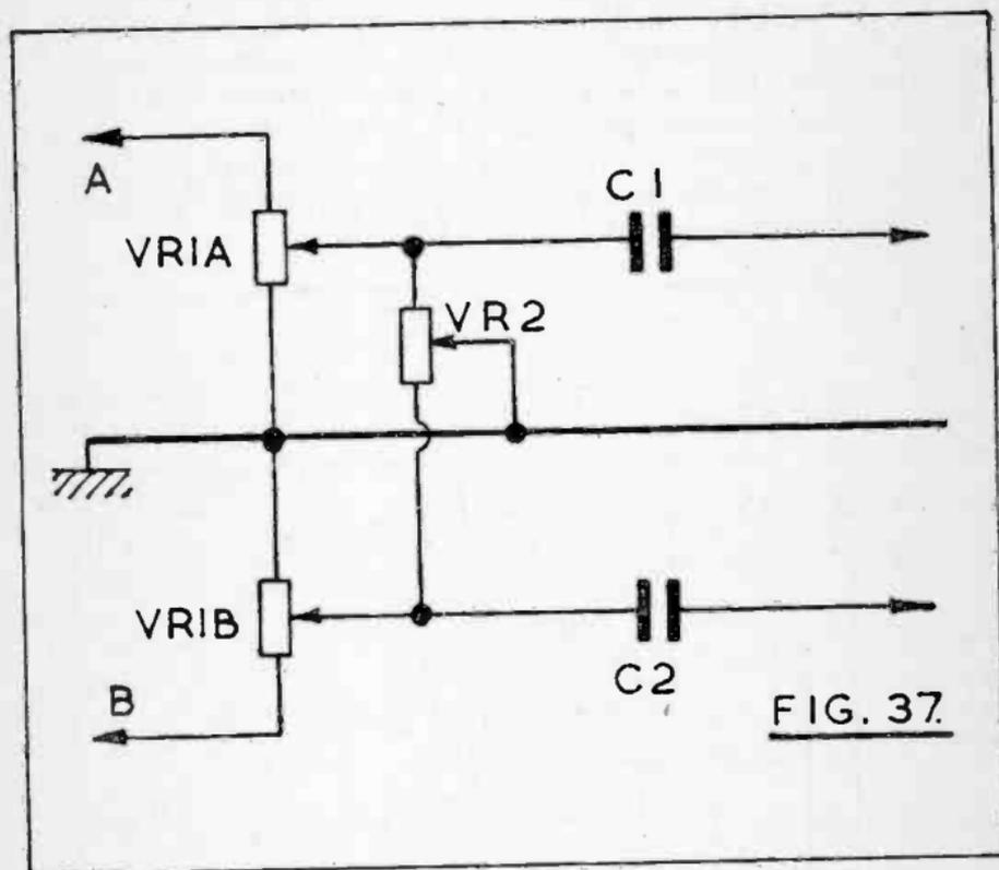
Fig.37 shows a circuit of this kind. Inputs A and B are from pre-amplifiers or other source, and volume is controlled by the ganged potentiometer VR1A/B. Here, 220k controls will often be suitable, though this can depend on other parts of the circuit. VR2 is the balancing control, and can generally be a 470k or 1 megohm linear potentiometer. C1 and C2 couple signals to the respective amplifiers. Other means of balancing will be found in the section on preamplifiers.
