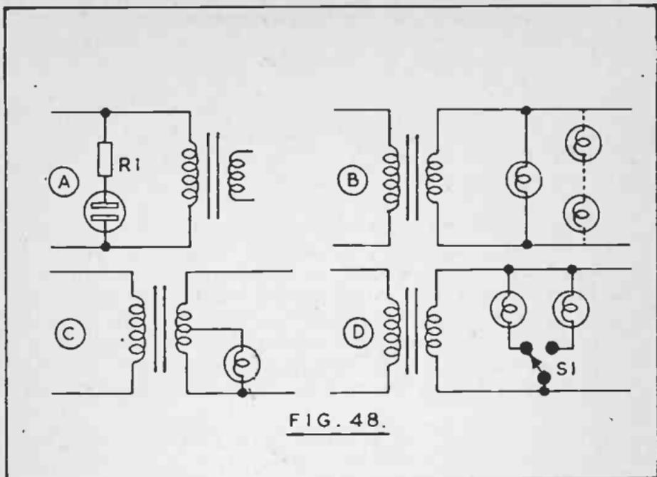
to minimise the additional load on the transformer. Two bulbs of the same current rating may be in series, to obtain a higher voltage with readily-available low-voltage bulbs.
