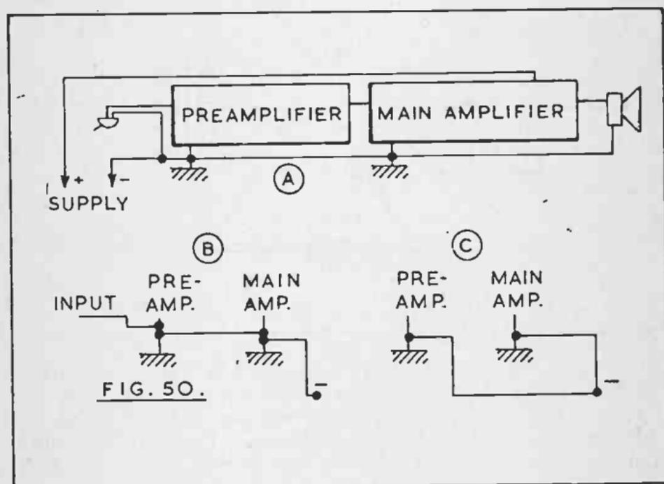
At B, current for the main amplifier and speaker does not flow in return circuits used by the preamplifier or input. At C, the power supply negative terminal is taken separately to both preamplifier and main amplifier, with a similar effect.
