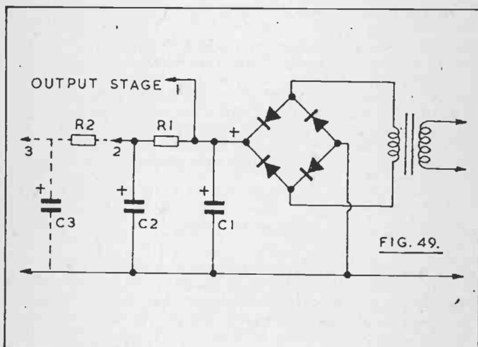
In Fig.49 C1 is charged by the rectifiers. Current is usually taken from here, at 1, for the output stage, and often driver/output stages. Some ripple is present, but maximum voltage and current are available at this point, and hum will not usually arise if C1 is of adequate capacitance.
