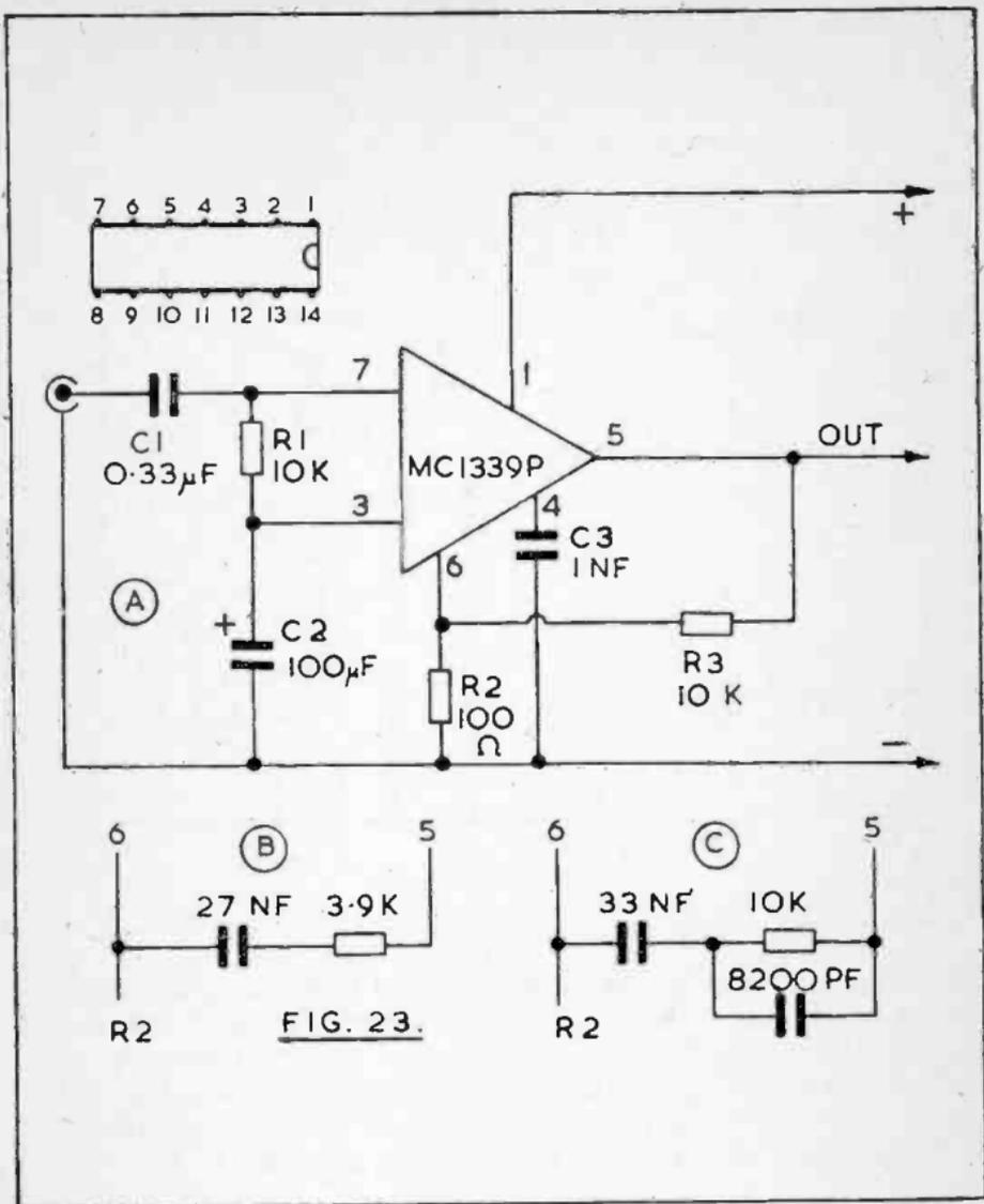
increases as frequency rises, reducing gain with higher frequencies. C has a similar effect, R3 being replaced by the items shown. This allows equalisation of the preamplifier for use with a magnetic pick-up. R1 is changed to 47k.
