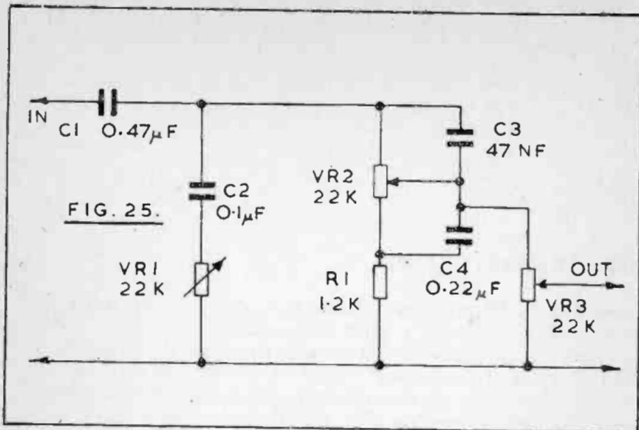
low value. Its reactance is lower at higher frequencies and in this position it thus allows higher frequencies to pass to VR3, providing emphasis of upper tones. This effect falls off as VR2 is adjusted away from R1, until the other maximum position of VR2 effectively removes C3 from circuit, while C4 reduces the upper frequencies. VR3 is the volume control.
