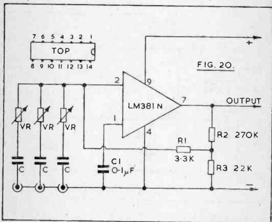
Fig.20 is a 3-channel mixer for inputs of medium impedance, and needs few components. Each input has an isolating capacitor C, the value being about  $0.5\mu\text{F}$ . VR for each channel is the volume control allowing individual adjustment of signal level, and can be about 470k.
