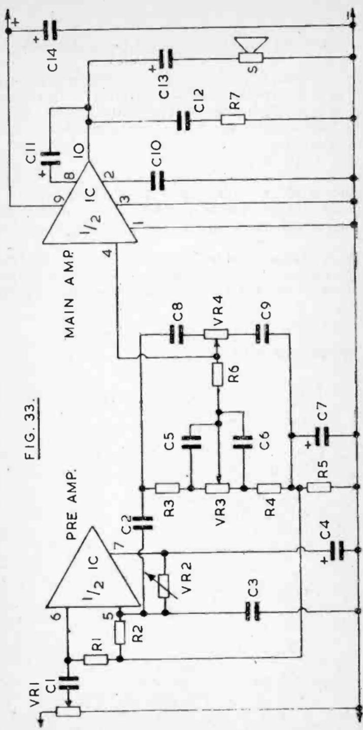
With the amplifier sections in cascade gain is high, and the layout should separate input and output circuits and components. C3 should be close up to leads 4 and 5. Both preamplifier and main amplifier have very high impedance inputs, and with some layouts a low value HF bypass capacitor may also be required for the preamplifier input.
