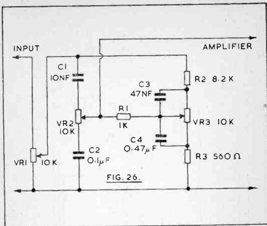
type could be likened to a treble boost control. Simple equipment may have a top-cut control only, with circuitry which tends to emphasise treble. Other circuits may use a single potentiometer, arranged to lift treble at one extreme, and lift bass at the other. Slightly more complicated are circuits such as those shown, which give a useful degree of control over treble and bass with separate potentiometers.
