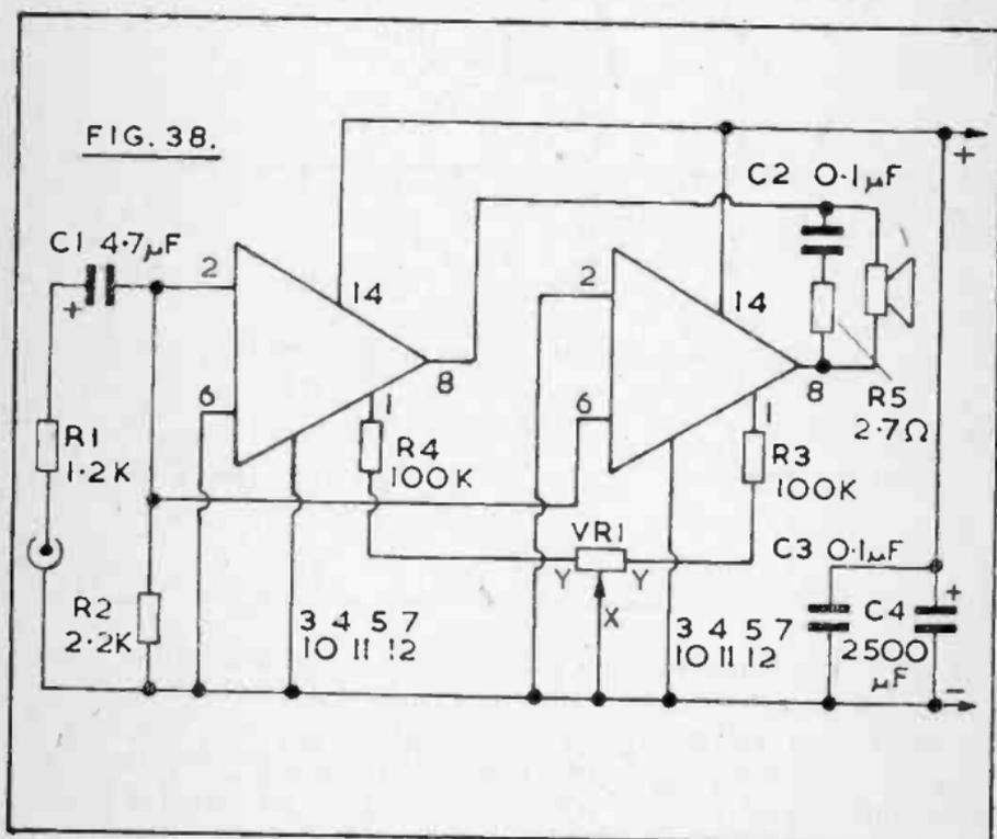
C3 across C4 is to help avoid HF instability (possibly not audible) which will cause heavy current, but very poor reproduction. The speaker and output circuits should be removed from input circuits, for the same reason.
