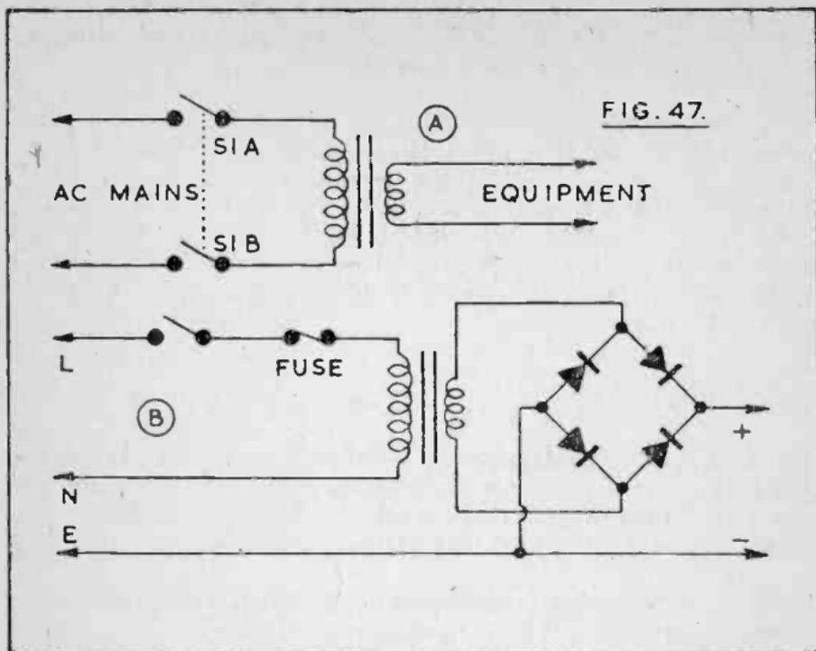
current flowing through the earth return would blow the protective fuse, so that the equipment remains safe.
