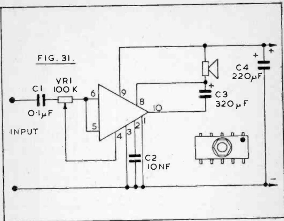
The layout should place the by-pass capacitor near 9 and 1. No instability difficulties should arise with normal separation of input and output circuits.
