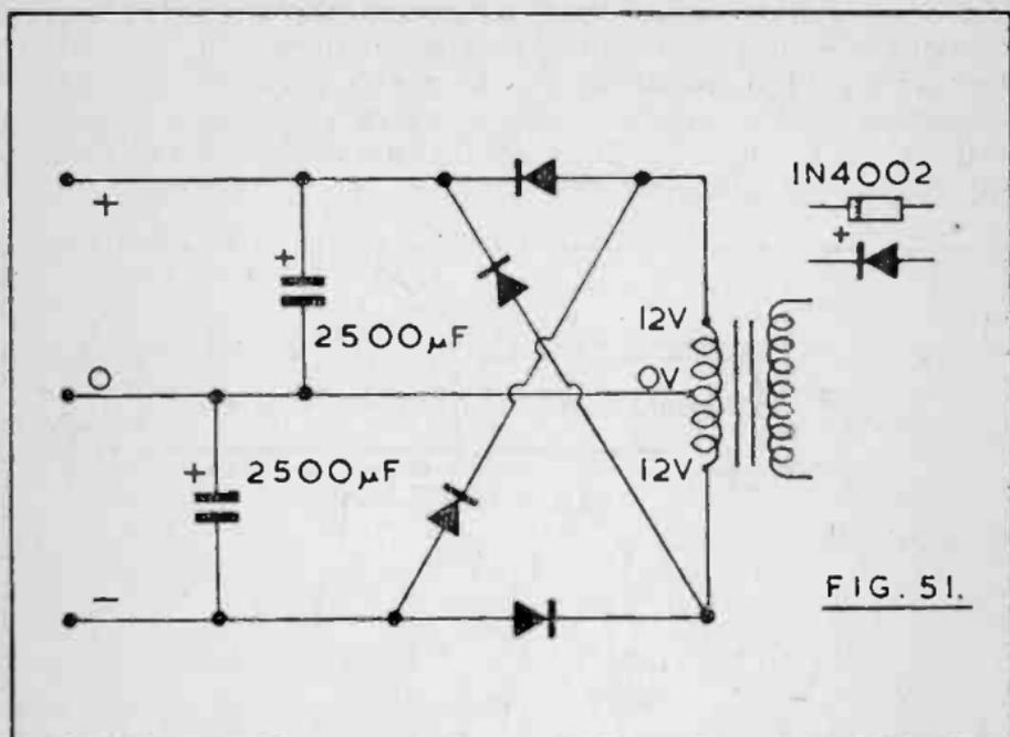
The circuit in Fig.51 can be used when a split power supply is required. In Fig.46 the use of a centre-tapped transformer and two rectifiers provides a positive supply line with the centre-tap of the secondary as negative line. By adding further rectifiers as in Fig.52 an equal but opposite polarity supply is obtained, with reference to the centre tapping.
