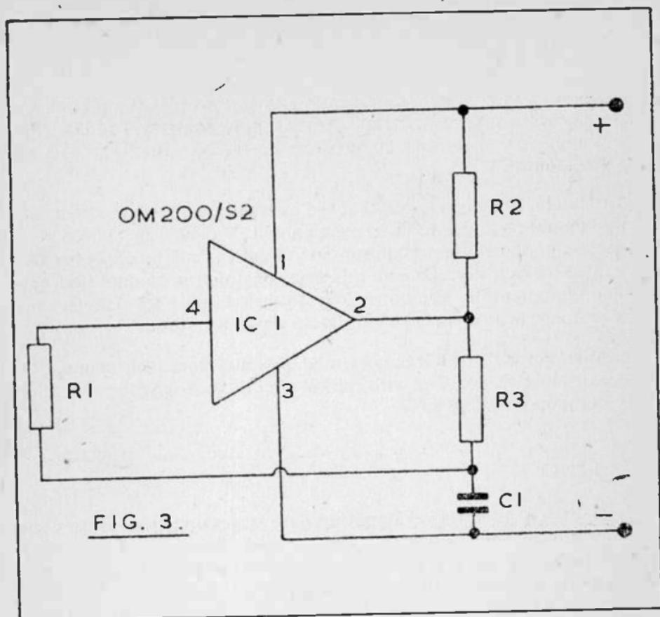
amplifier. Otherwise the audio power available here is used without further amplification. R2 is then an earpiece.
