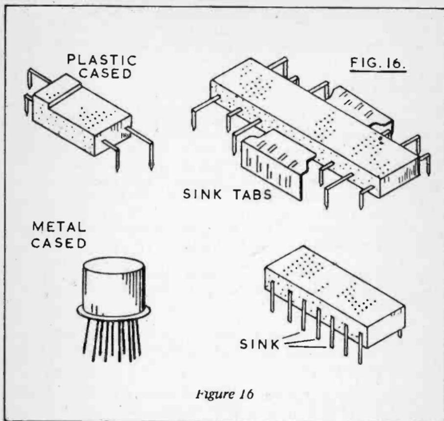
The SL414/5 ICs are an example of how power dissipation permissible in the device depends on heat sinking. With an ambient temperature of  $25^{\circ}\text{C}$  and no heat sink, dissipation is limited to just under 2.5W. With an 18swg aluminium heat sink approximately  $4 \times 6\text{cm}$  in size, dissipation is raised to over 6 watts. The heat sink is thus an essential part of most IC amplifier designs, and must not be omitted.
