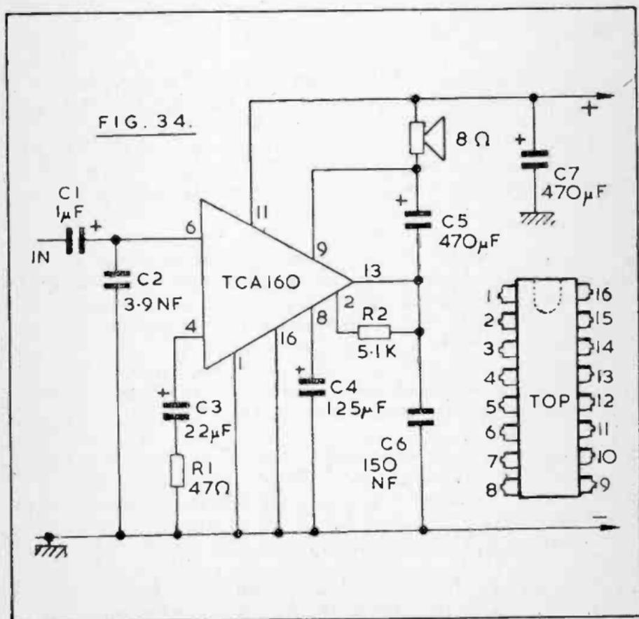
In Fig.34 coupling to the input is via C1. C2 may be modified in value. Its purpose is to limit upper frequencies, and to avoid instability if the input is not connected. In a similar way, C3 may be increased in value to obtain an extended bass performance. R1 may also be adjusted to change gain. However, values shown are typical and can generally be used.
