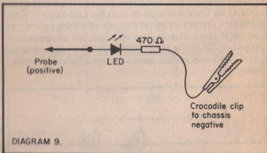
If the tester is required for use with a positive chassis car the LED should be wired the other way round so that the anode is connected to the chassis (positive).
