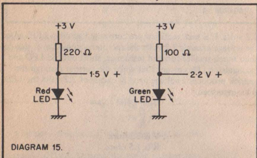
This is very useful as zener diodes are not available in voltages below 2.7V. The current through the LED must, as with a zener diode, be limited by a resistor. If a 2.2 volt reference source is required a green LED can be utilised. The LEDs are under forward bias unlike a true zener diode which is reverse biased for voltage regulation i.e. with cathode positive.
