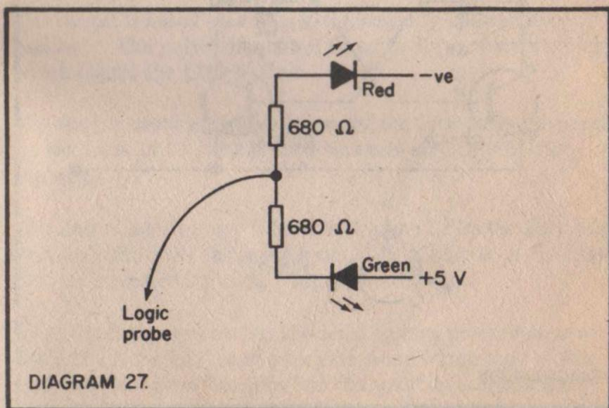
When the probe is connected to the 5 volt supply both red and green LEDs will glow. When the logic probe touches a circuit connection, if the GREEN LED glows brightly this indicates logic level 0, if the RED LED glows brightly this indicates logic level 1.
