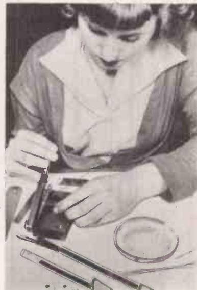
The whiskers of the GET-1 are soldered to the support wires in a delicately adjusted jig, every care being taken to ensure that no strain is imposed on the whiskers during this operation.
