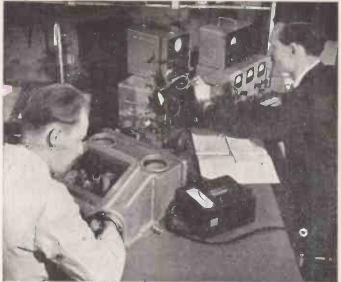
A view of the G.E.C. laboratories, where the electrical characteristics of experimental transistors are being measured in a moisture-free box. The right-hand operator is measuring the back current of the collector and current gain, observing characteristics on an oscilloscope.
