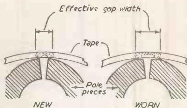
Fig. 3. Showing the increase in effective gap width due to wear on the pole pieces.
