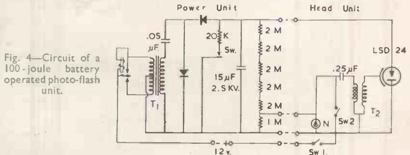
Fig. 4—Circuit of a 100-joule battery operated photo-flash unit.
