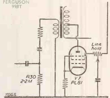
to about 4MΩ. In replacing this component it is advisable to use a resistor of solid carbon 1 watt type.—M.A.H., Exeter.
