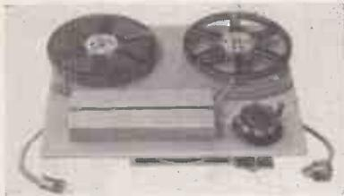
A tape mechanism using a three-motor driving system, made by M.S.S.
