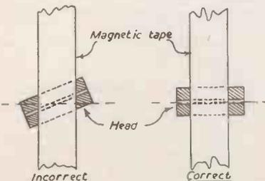
Fig. 2. Incorrect and correct alignment of the recording head.
