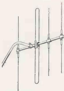
A 4-element aerial designed for use in either the primary service area or fringe areas of Band III.
