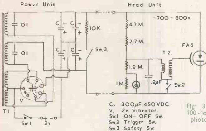
Fig. 3—Circuit of 100-joule portable photo-flash unit.
