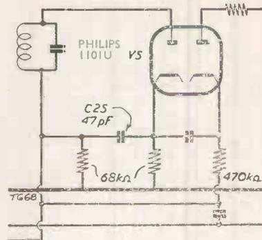
voltage tests showed no obvious discrepancies. After this, attention was directed to the sound detector stage and in checking over the components it was found that the 47pF filter capacitor C25 had developed a leak of around 30kΩ.—R.R., Mansfield, Notts.
