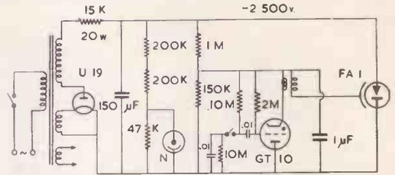
the common earth. If triggering circuit is in order, a spark should jump across when pressing switch.
