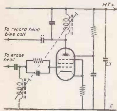
Fig. 4. A typical h.f. oscillator circuit.
