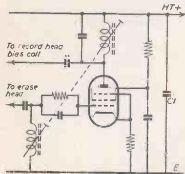
Fig. 4. A typical h.f. oscillator circuit.
