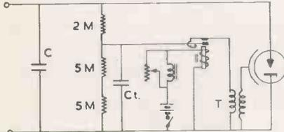
Fig. 6—Diagram of a relay-triggered system.
