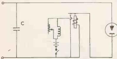
Fig. 7—Trigger system for a self-ignition tube.
