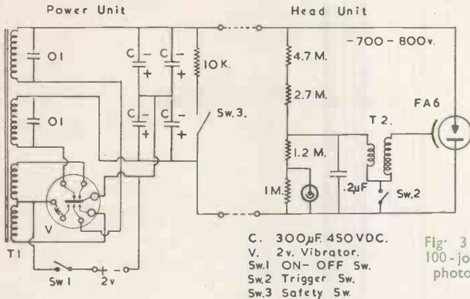
Fig. 3—Circuit of 100-joule portable photo-flash unit.
