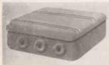
Fig. 1: A cross-over network box, to couple two aerial inputs together to provide a common input to the receiver
