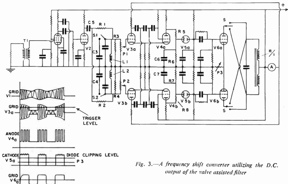
Fig. 3.—A frequency shift converter utilizing the D.C. output of the valve assisted filter
