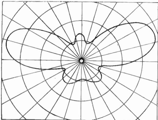
Fig. 3.—Directional antenna pattern.
