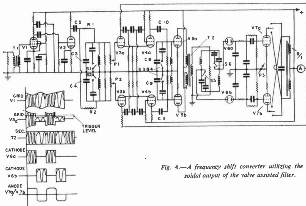
Fig. 4.—A frequency shift converter utilizing the sinusoidal output of the valve assisted filter.
