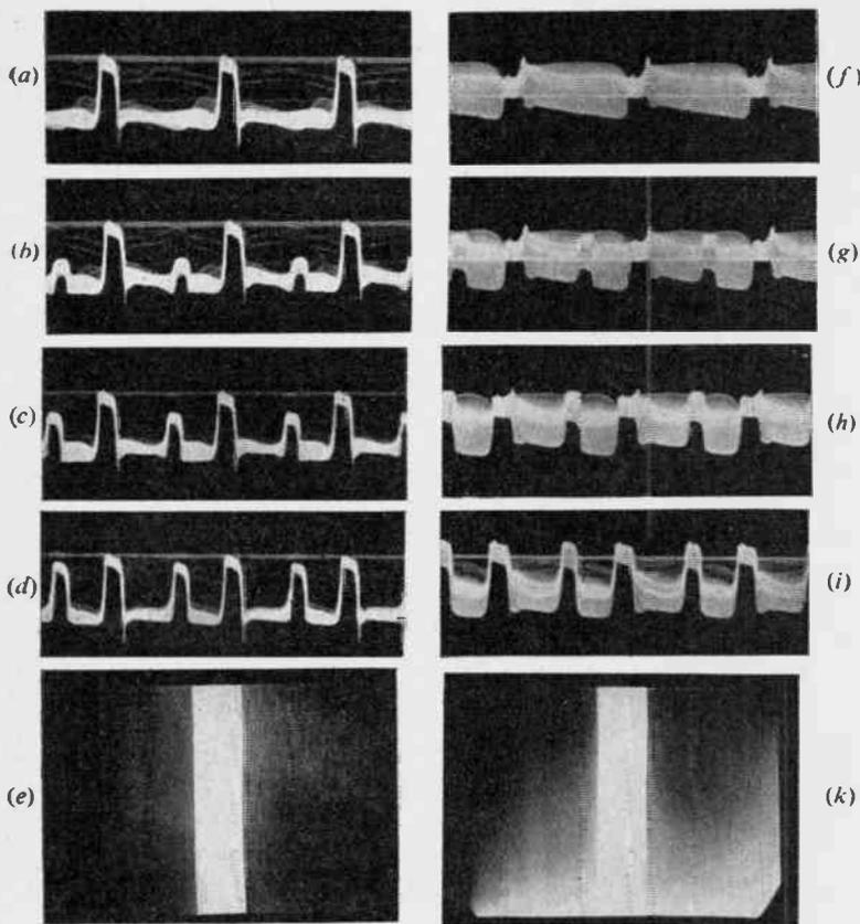
Fig. 11.—Oscillograms of the Photicon output signal and television pictures scanning a vertical white bar on a black field:
