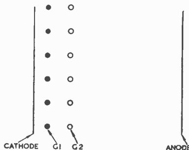
Fig. 11.—Section of a tetrode with aligned grids in a plane perpendicular to the helix wires.
