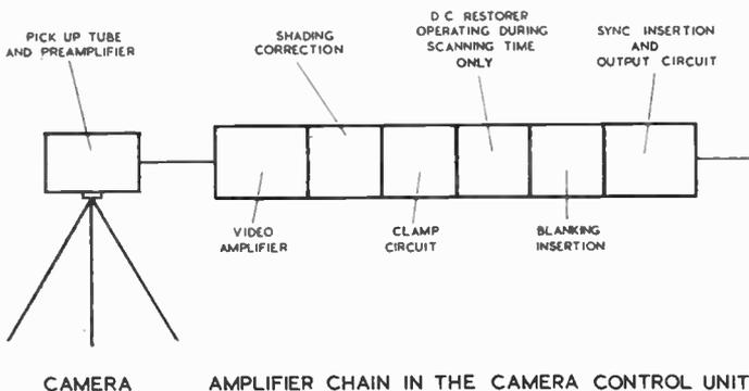
Fig. 5.—Block diagram of the amplifier chain in a "Photicon" camera control unit.
