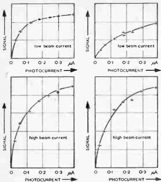
Fig. 12.—Signal output as a function of scene brightness (photo-current) with and without bias technique, televising a pattern of vertical black-and-white strips.
