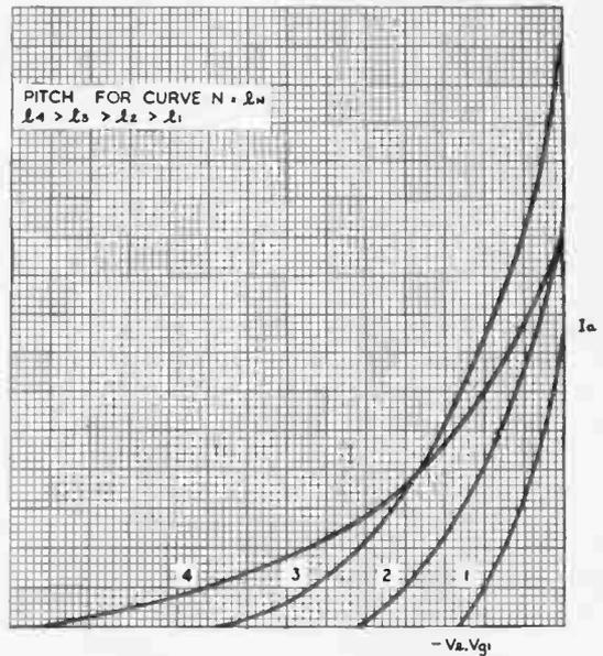
Fig. 12.—Series of curves of  $I_a$  versus  $V_{g1}$  for an aligned beam tetrode with various pitches on  $g_1$  and  $g_2$  keeping  $V_a = V_{g2} = \text{const.}$
