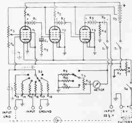
Fig. 3.—Modified Vance amplifier.
