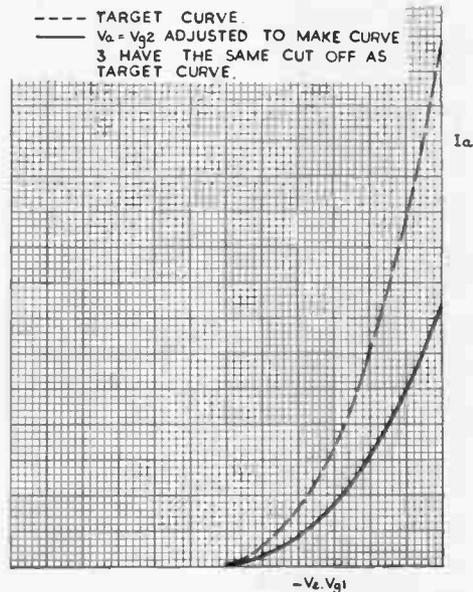
Fig. 13.— $I_a$  versus  $V_{g1}$  curve showing the first stage in adjusting the characteristics to fit the target curve.
