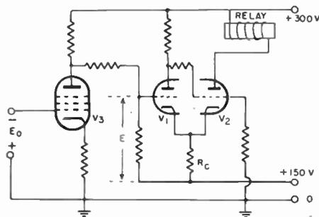
Fig. 15.—Trigger circuit for automatic titrations (Muller and Lingane).
