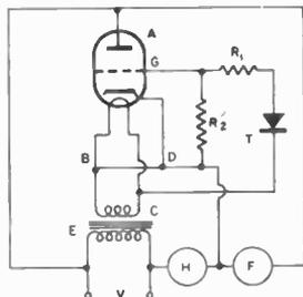
Fig. 28.—Thermo-regulator for mercury thermostat (Swinehart).
