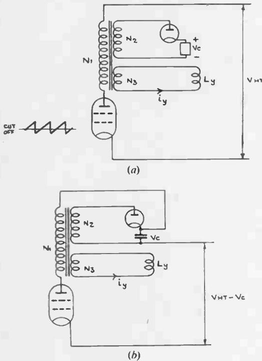
Fig. 5.—Series power feedback basic circuit.
