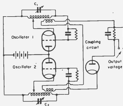
Fig. 25.—Circuit for the measurement of the solid to gas ratio (Dotson and others).
