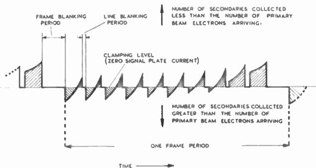
Fig. 3.—Diagram of an image iconoscope signal after "clamping" over one frame period without light on the photo-cathode.
