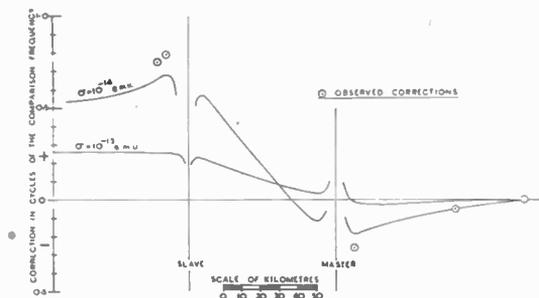
Fig. 11.—Decca survey chain in Sweden: comparison frequency 354 kc/s.
