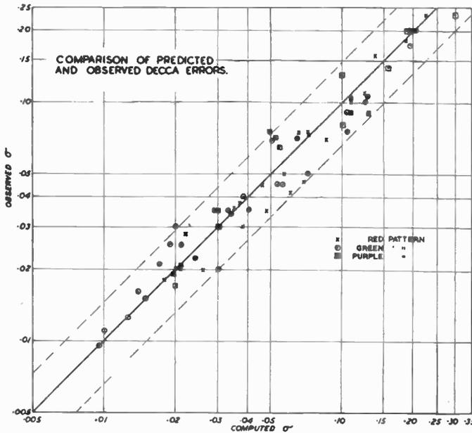
Fig. 7. Comparison of predicted and observed Decca errors.
