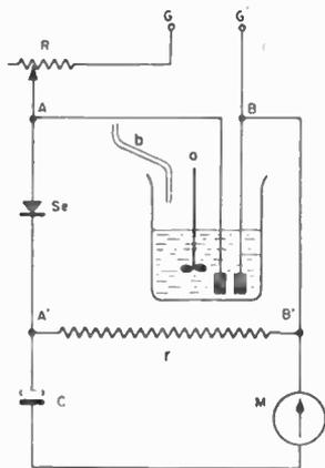
Fig. 20.—Principle of Delahaye's method for electro-metric titrations.
