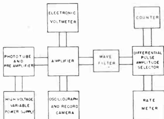
Fig. 7.—Apparatus for size distribution studies in aerosols (Gucker and O'Konski).
