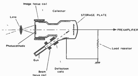
Fig. 1.—Diagram of an image iconoscope type pick-up tube.
