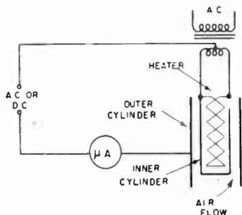
Fig. 30.—Halogen vapour detector (White and Hickey).
