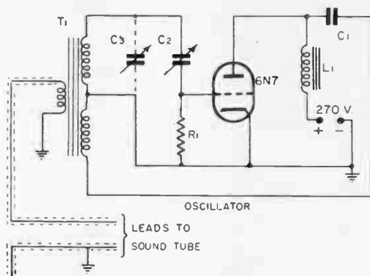
Fig. 9.—Doubly-stabilized tuned grid oscillator (Crouthamel and Diehl).
