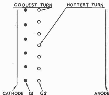
Fig. 10.—Section of a tetrode with non-aligned grids in a plane perpendicular to the helix wires.
