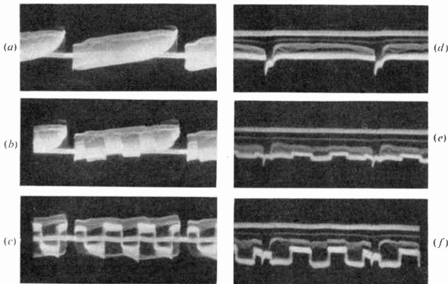
Fig. 4.—Oscillograms of an image iconoscope signal after "clamping" over one frame period, televising a pattern of black-and-white horizontal bars: (a), (b), (c) without shading correction, light level increasing; (d), (e), (f) with shading correction, light level increasing.
