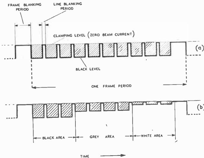
Fig. 10.—Diagram of the P.E.S. Photicon output signal waveform after clamping on the same time base as Fig. 3, televising a black frame (a) and a frame of three tones (b).
