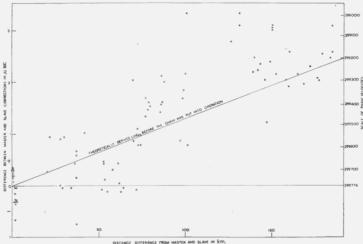
Fig. 16.—North British Decca Chain: results of observations on the comparison frequency 253.9 kc/s.
