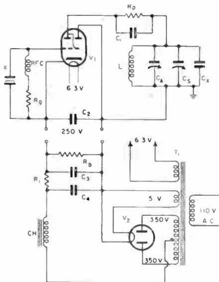
Fig. 22.—Bender's modifications of Alexander's dielectric constant meter.
