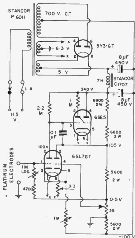
Fig. 26.—Mains-operated instrument for Karl Fischer moisture determinations (Kieselbach).
