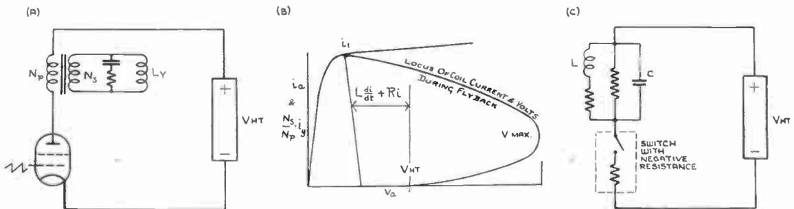
Fig. 2.—Heavily damped scanning with no energy recovery. Saw-tooth grid drive.
