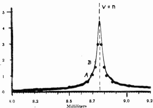
Fig. 13.—Variations of indicator current in titration of  $\text{AgNO}_3$  by a  $\text{NaCl}$  solution (Delahaye).
