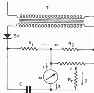
Fig. 21.—Circuit for the compensation of capacitor leakage currents (Delahaye).
