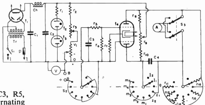
Fig. 14.—Electronic device for potentiometric titrations (Delahaye).
