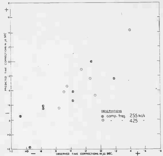
Fig. 15.—Theoretically predicted time corrections v. observed corrections.
