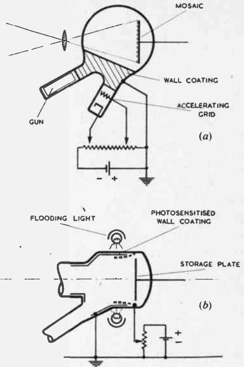
Fig. 6.—Arrangements to irradiate the storage surface with low-velocity electrons.
