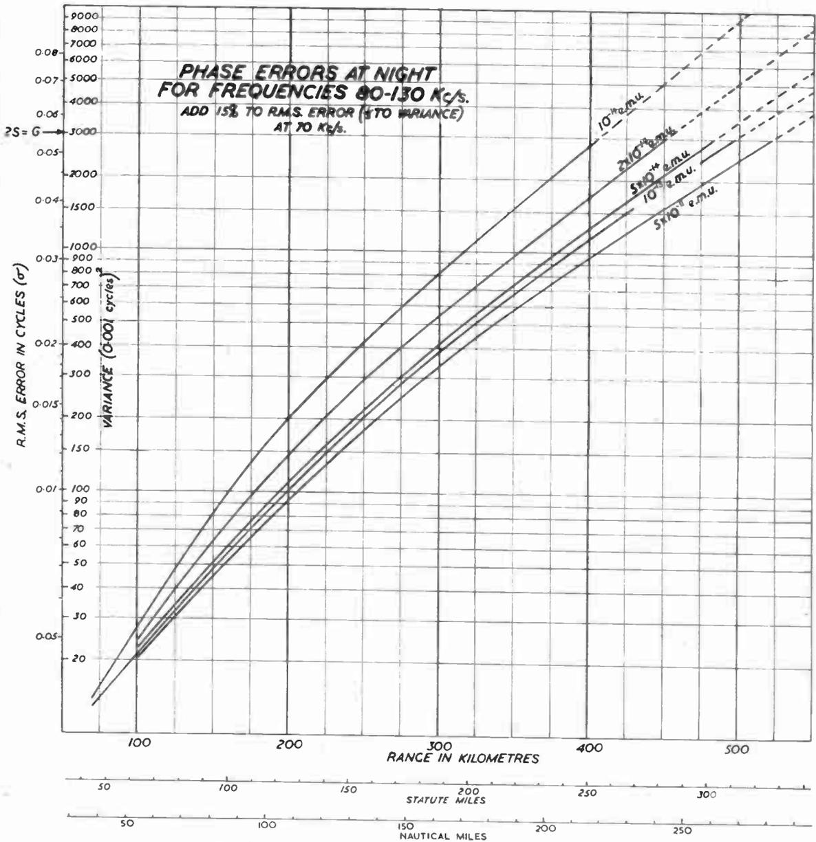
Fig. 4. Phase errors at night for frequencies 80-130 kc/s.
