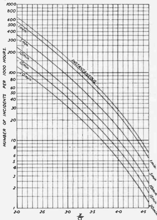
Fig. 10. Number of separate occasions per 1,000 hours' observation when error is likely to exceed a given value of  $x/\sigma$ .
