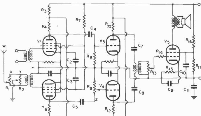
Fig. 19.—Apparatus for the cancellation of stray interferences in conductivity measurements (Ives and Pittman).
