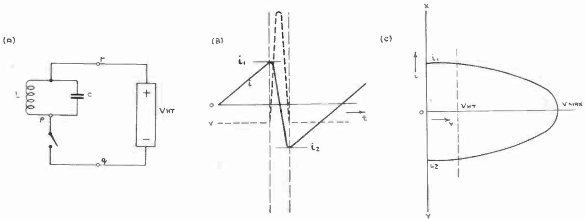
Fig. 1.—The basic scanning circuit.
