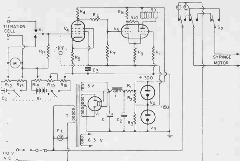
actual physical contact with the solution. They are particularly suited for titrations where the endpoint is difficult to detect by other methods. Blaedel and Malmstadt,<sup>47</sup> describe a titrimeter operating at 30 Mc/s. West, Barkhalter and Broussard,<sup>49</sup> also describe a titrimeter, utilizing a heterodyne principle to detect the detuning and/or loss produced by the progress of titration.
