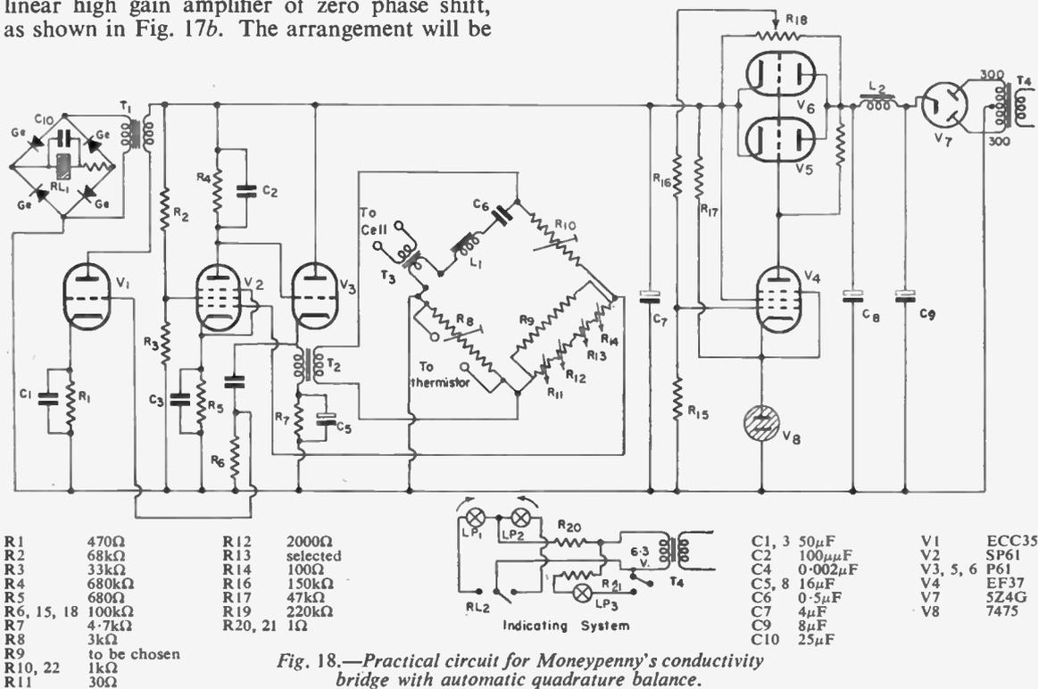
Fig. 18.—Practical circuit for Moneypenny's conductivity bridge with automatic quadrature balance.
