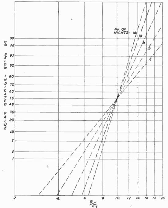
Fig. 8. Graph showing the number of whole nights' observations required to obtain an error value within any specified limits.
