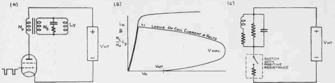
Fig. 3.—Heavily damped scanning with no energy recovery. Square pulse grid drive.
