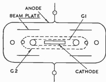
Fig. 9.—Plan of electrodes in a typical beam tetrode.
