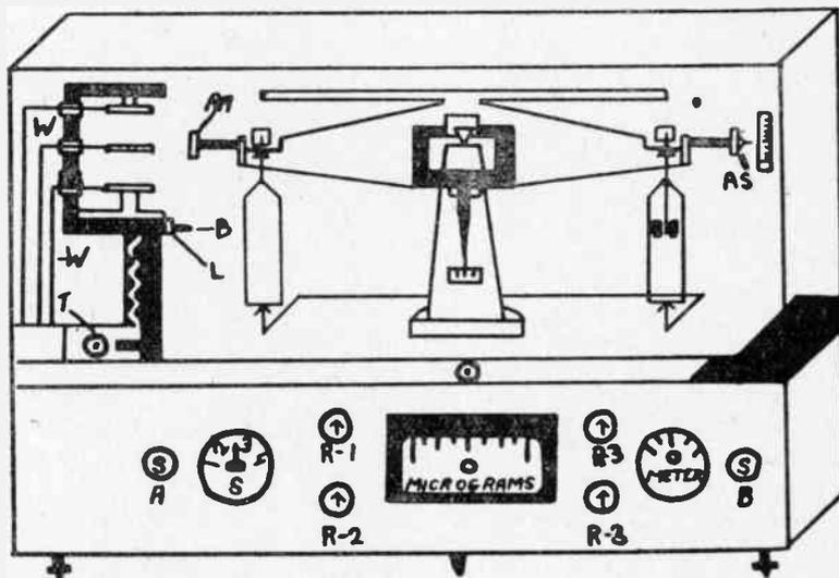
Fig. 32.—Principle of electronic balance indicator (Feuer).
