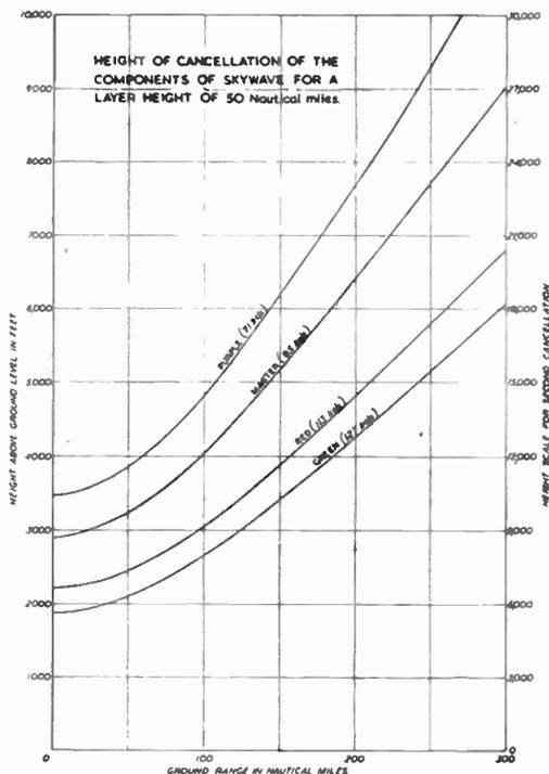
Fig. 11. Height of cancellation of the components of skywave for a layer height of 50 nautical miles.
