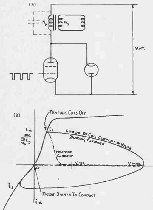
Fig. 4.—Parallel power feedback.
