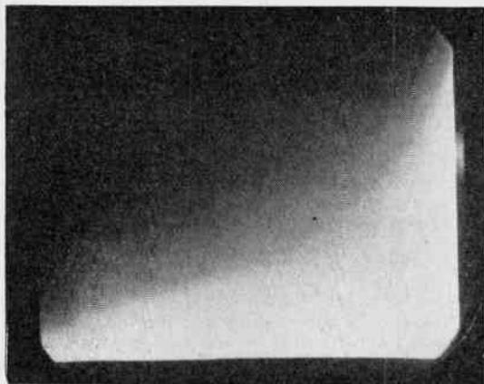
(a) Typical nature of background shading due to spurious signals without light on the photo-cathode.
