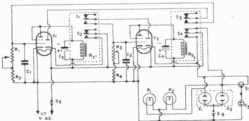
Fig. 29.—Reflux ratio timer (Fisher).
