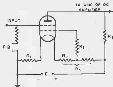
Fig. 2.—Balanced electrometer circuit (Caldwell).
