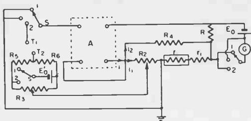
Fig. 1.—Principle of Morton's potentiometric pH meter.
