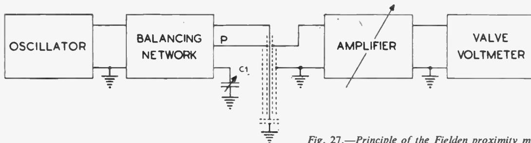
Fig. 27.—Principle of the Fielden proximity meter.
