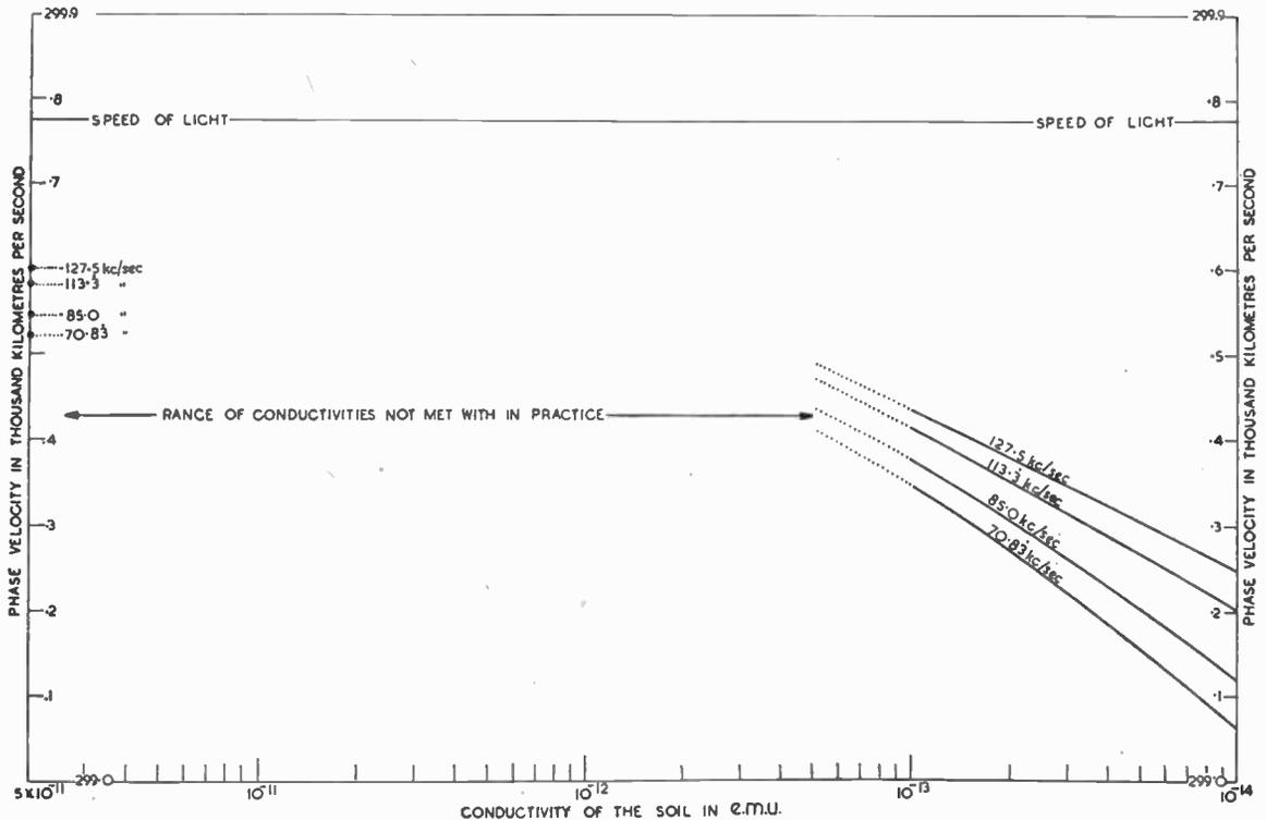
*Fig. 7.—Phase velocity at long range versus homogeneous soil conductivities.*
