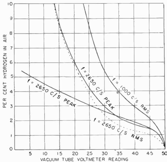
Fig. 11.—Calibration curves for hydrogen-air mixtures (Crouthamel and Diehl).
