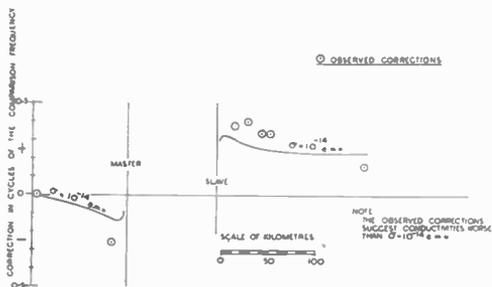
Fig. 10.—Decca survey chain in Sweden: comparison frequency 265 kc/s.
