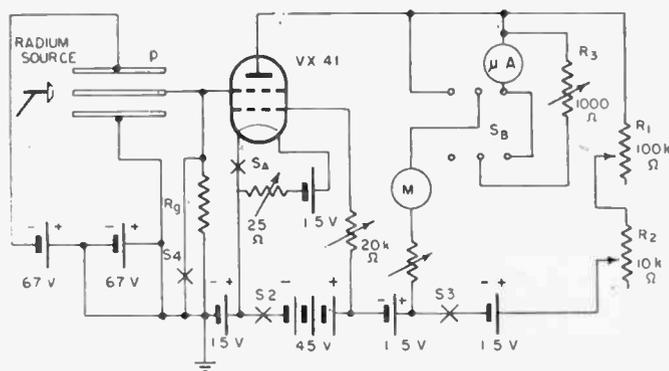
Fig. 33.—Circuit arrangement for Feuer's electronic balance indicator.
