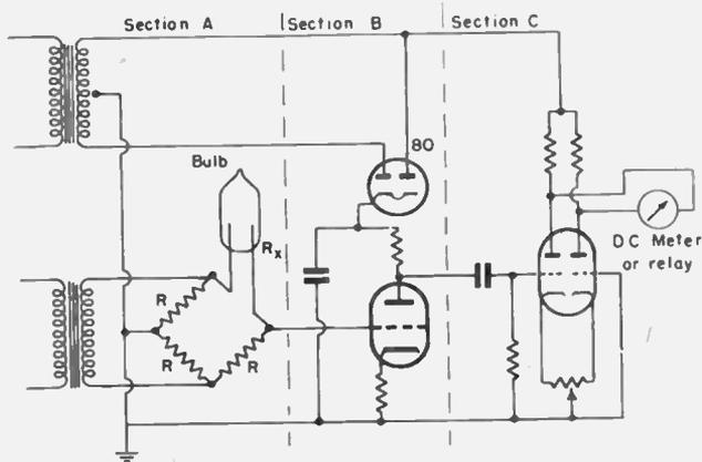
Fig. 31.—Electronic thermometer for thermistors (Weiller and Blatz).
