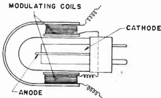
Fig. 5.—Magnetic modulation of electron current in photo-tubes (Kalmus and Striker).
