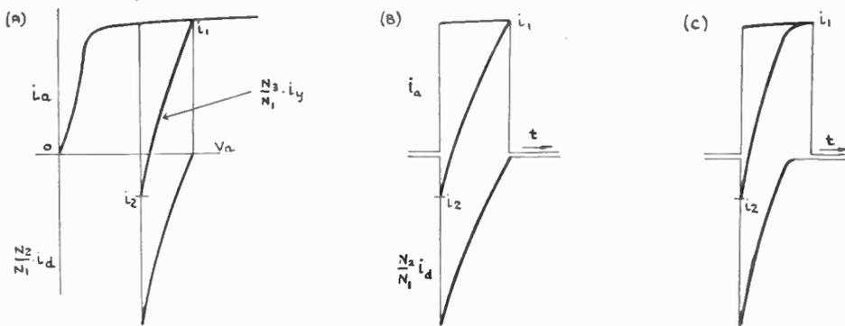
Fig. 7.—Relationship between diode current and pentode current for series power feedback when grid drive is square pulse.
