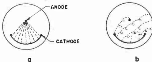
Fig. 6.—(a) Approximate path of photoelectrons in the absence of magnetic field.
