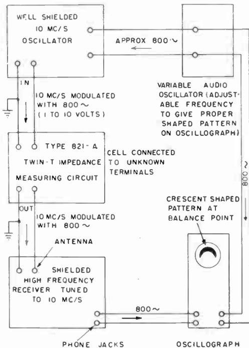
Fig. 23.—Oscillographic method for dielectric constant determinations (Elliott, Jones and Lockhart).
