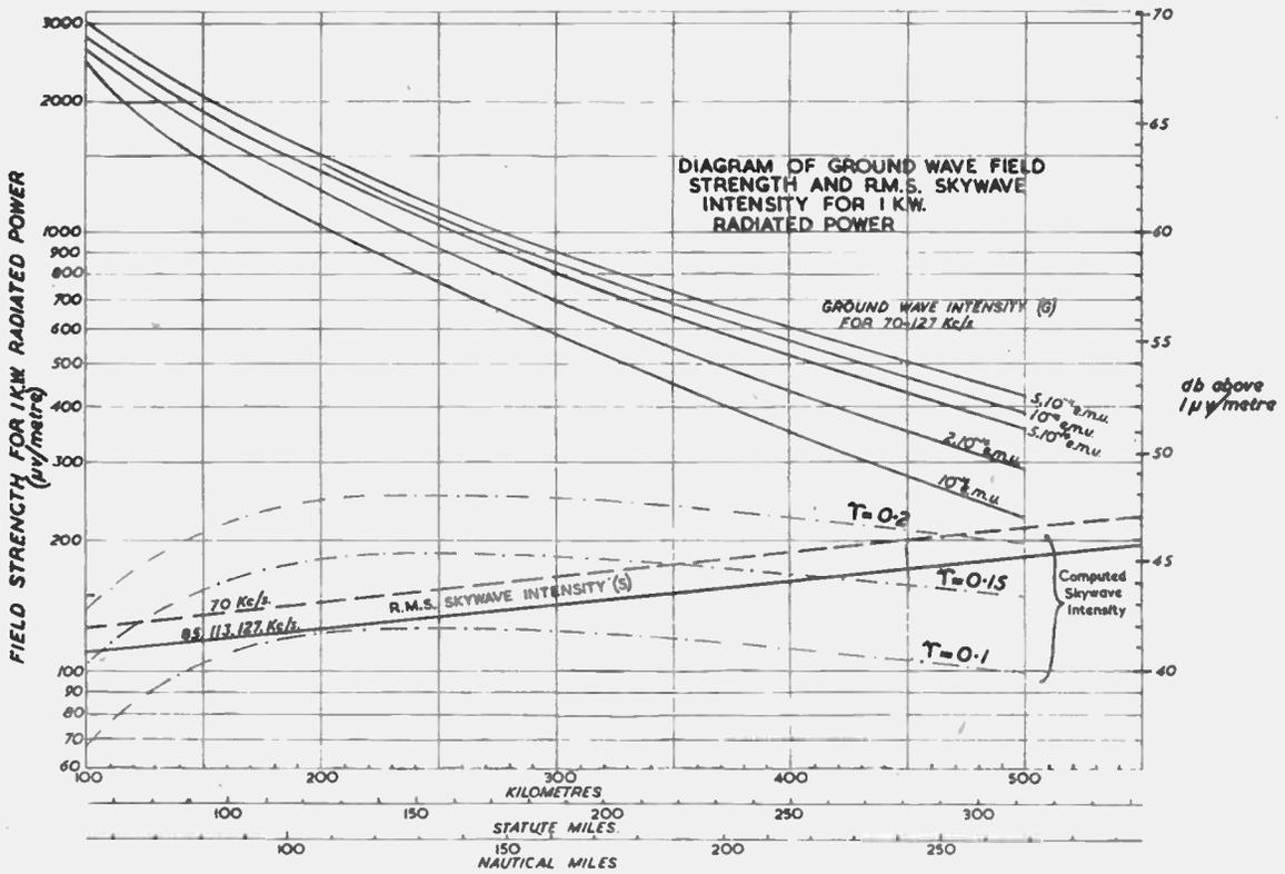
Fig. 2. Diagram of ground wave field strength and R.M.S. skywave intensity for 1 kW radiated power.
