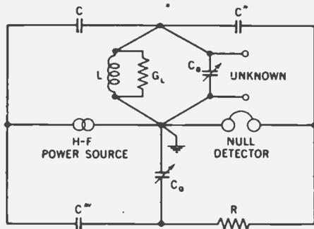
Fig. 24.—Twin-T impedance measuring circuit (General Radio).
