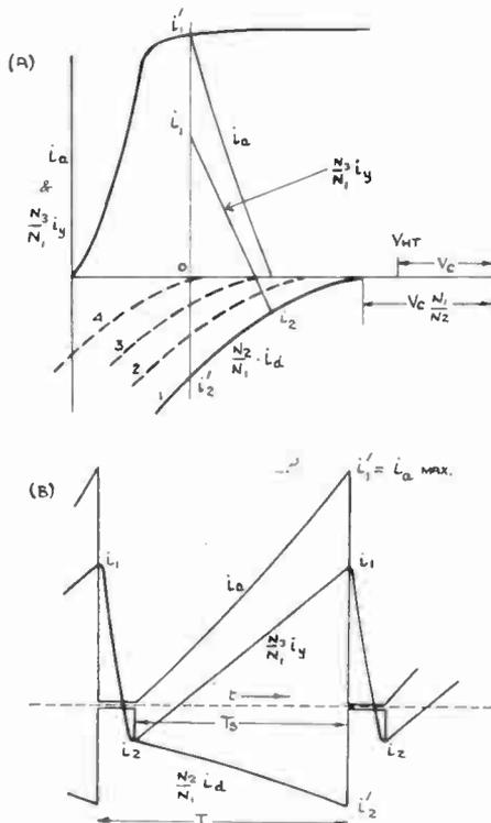
Fig. 6.—Relationship between diode current and pentode current in circuit of Fig. 5(b) when scanning coils have finite resistance and no correcting voltage is applied to the diode cathode.
