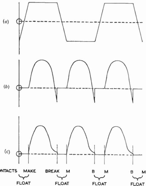
Fig. 8.—Voltage and current waveforms for circuit of Fig. 7. (a) Buffered transformer, output voltage waveform, (b) input (d.c.) current waveform, undamped output circuit, (c) input (d.c.) current waveform, damped output circuit.
