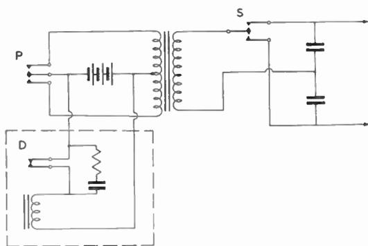
Fig. 2.—Split reed, separately-driven vibrator power pack.
