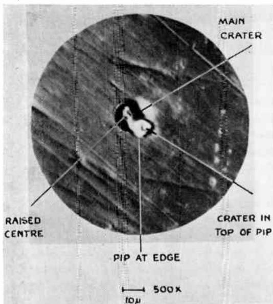
Fig. 4.—Shadow photograph of cathode contact after a single break at 1.5 V, 28 A.
