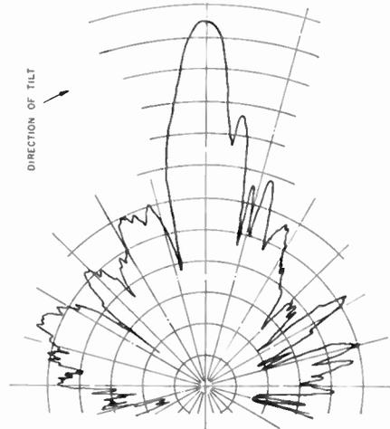
Fig. 6.—Vertical polar diagram with maximum tilt.
