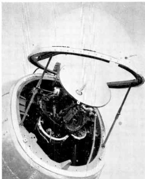
Fig. 3.—Scanner installed in nose of Viking with radome open.
