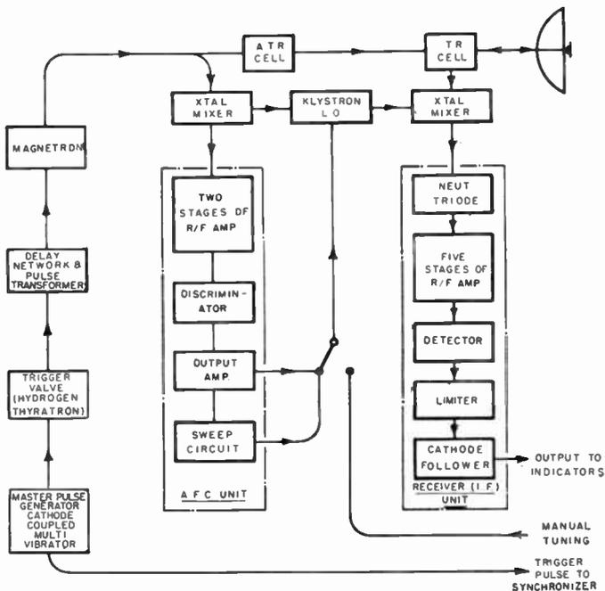
Fig. 9.—Transmitter-receiver—block diagram.
