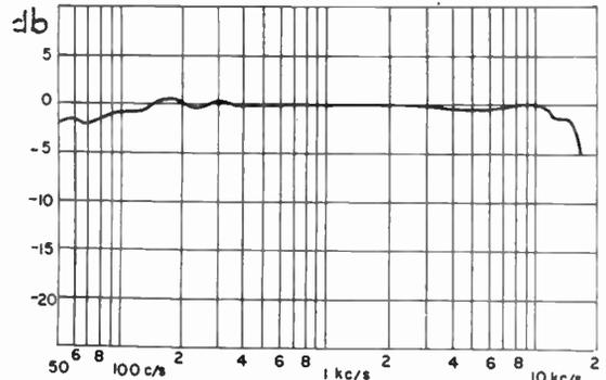
Fig. 6.—Overall frequency characteristic (L.C. tape).
