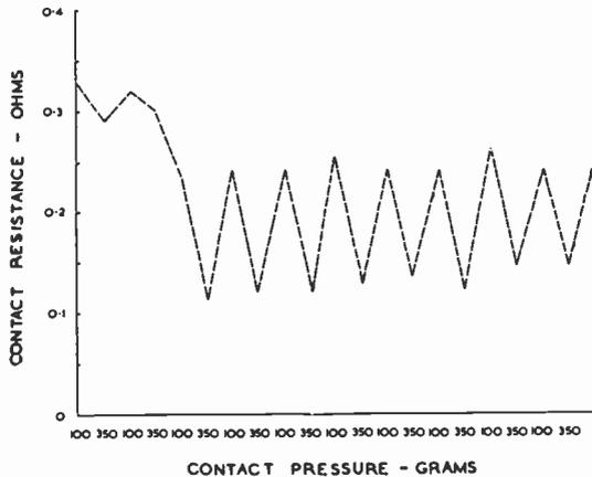
Fig. 1.—Relation between contact resistance and contact pressure.
