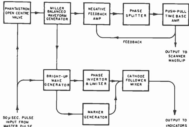
Fig. 10.—Synchronizer unit—block diagram.
