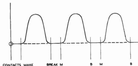
Fig. 9.—Input current. Commutated circuit with H.C.R.
