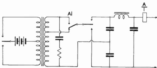
Fig. 12.—Power pack regulation by relay in transformer secondary circuit.
