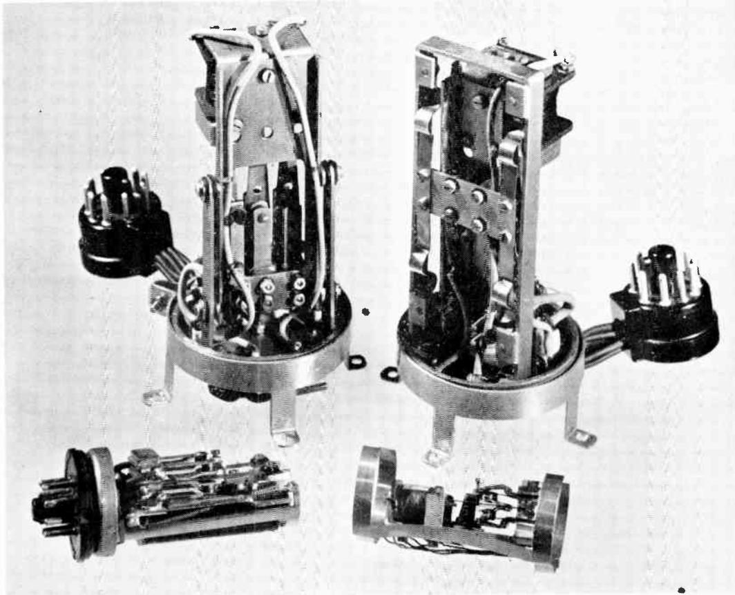
*Fig. 13.—Methods of mounting vibrators.*
