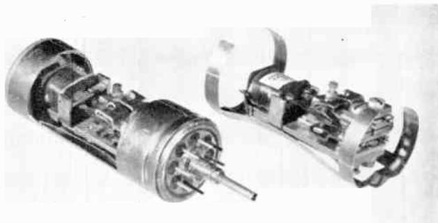
Fig. 16 (middle, right).—Miniature heavy-duty vibrator.
