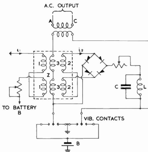
Fig. 11.—Power pack regulated by a saturable reactor in primary circuit.
