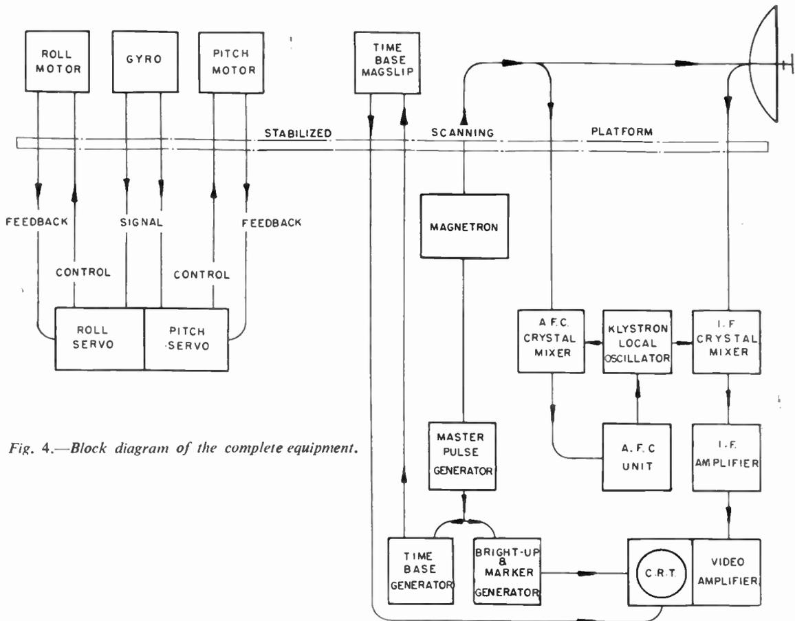
Fig. 4.—Block diagram of the complete equipment.
