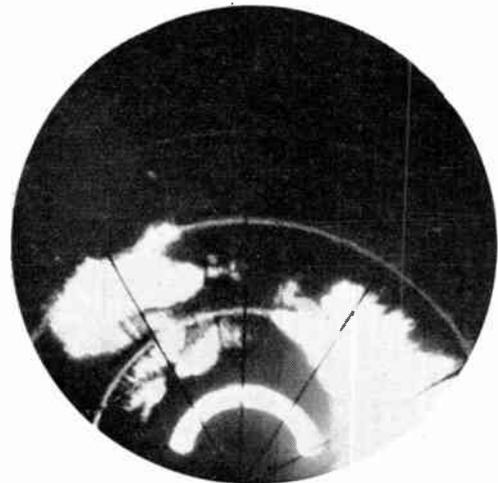
Fig. 12.—Example of a gap between two cumulo-nimbus clouds. This gap was observed on the indicator before it was seen visually. The aircraft was directed through by radar observations only.
