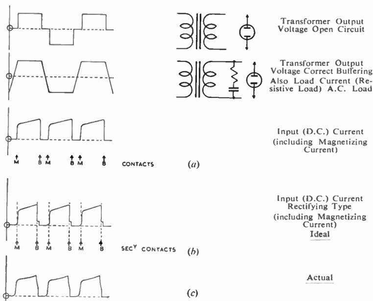
Fig. 6.—Voltage and current waveforms of vibrator, without and with commutation.
