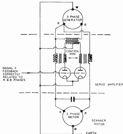
Fig. 7.—Simplifier servo amplifier unit.
