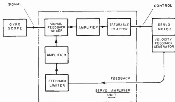
Fig. 8.—Servo system—block diagram.
