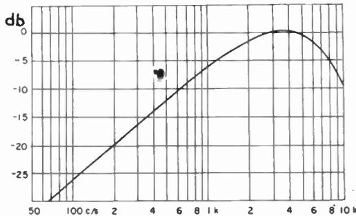
Fig. 2.—L.C. tape characteristic at 15 in per sec.
