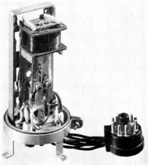
Fig. 18 (bottom, right).—High-power (250W) vibrator.
