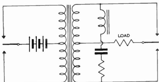
Fig. 10.—Parallel commutating circuit. Rectified load.
