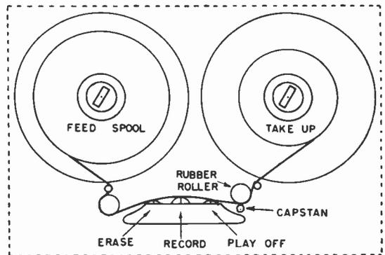
Fig. 1.—Layout of Magnetofon.
