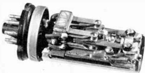
Fig. 17 (left).—Cleaned-up version of A.M. Type 14 vibrator (X331).
